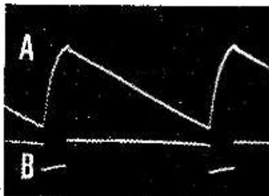
Fig. 2: The timebase waveform (above) and the flyback suppression (below) in the P.W. Workshop Oscilloscope.
