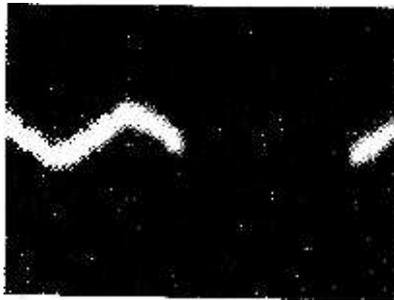
Fig. 31: Noise and hum from an amplifier.
