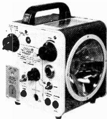
1209D. In addition to the many features of the well established Transistor Strobflash, the new design provides a high sensitivity input (minimum external trigger: 200mV r.m.s.) which enables the Strobflash to be triggered directly from such sources as vibration meters, vibration analysers or from an electromagnetic pickup.
