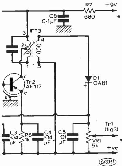
▲ Fig. 2: Intermediate frequency amplifier circuit.
