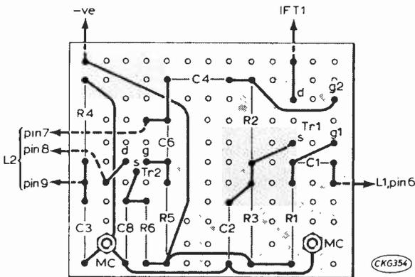
Fig. 5: Underside wiring of board shown in Fig. 4.
