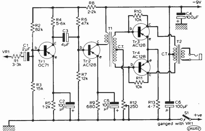
▲ Fig. 3: Circuit of the audio amplifier and output stages.
