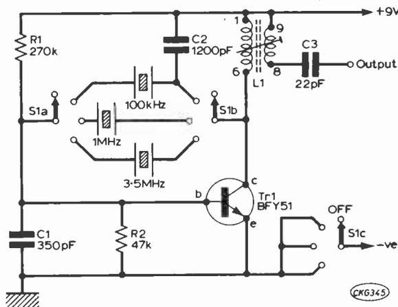
Fig. 1: Circuit diagram of the crystal marker.
