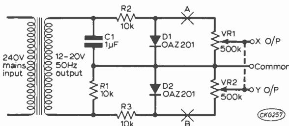
Fig. 1: The circuit of the 'scope calibrator.
