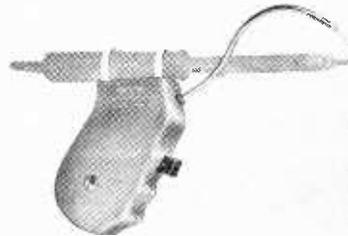
both the iron and solder in one hand, being free to hold the work with the other hand.
