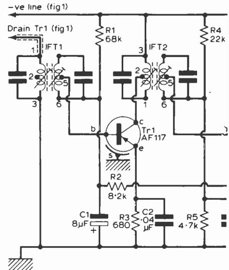
◀ Fig. 1: Circuit of the mixer-oscillator board.
