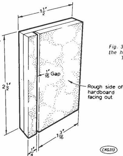
Fig. 3: The dimensions of the hardboard side fillets. Two are required.
