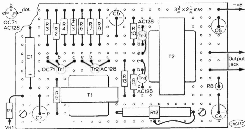
Fig. 8: Components on the audio stages board are placed as shown. Observe correct polarity of the several electrolytic capacitors.
