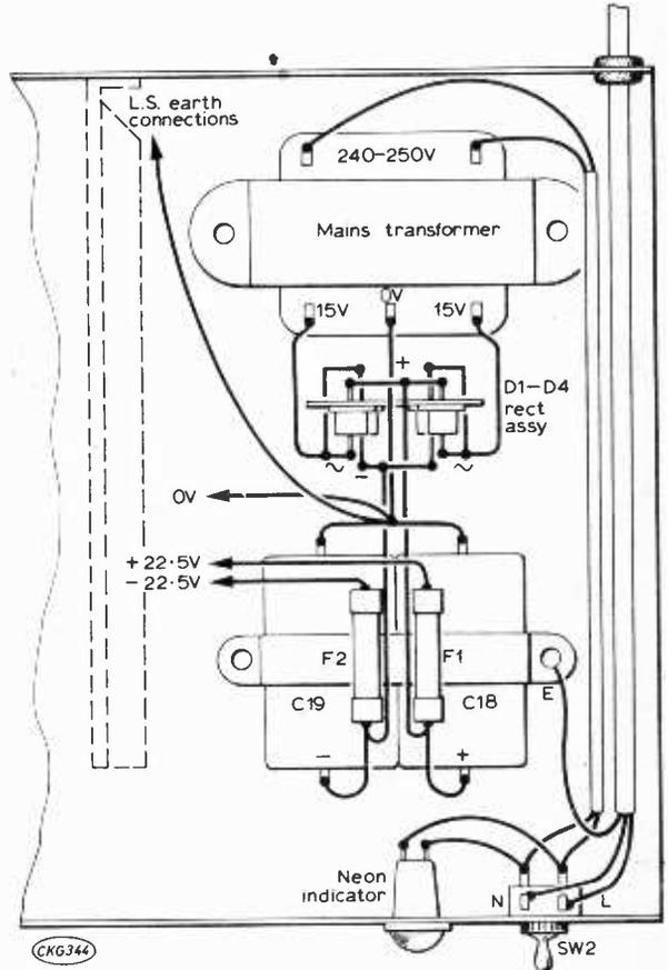
Fig. 9b: The layout of the power supply.
