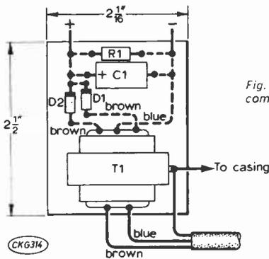
Fig. 2. The wiring of the components on the drilled s.r.b.p. board.
