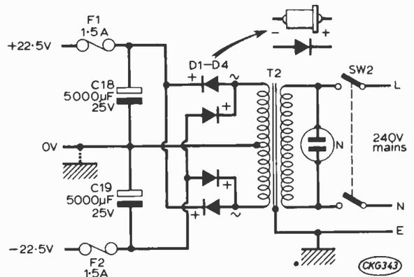
Fig. 9a: The circuit of the power supply.
