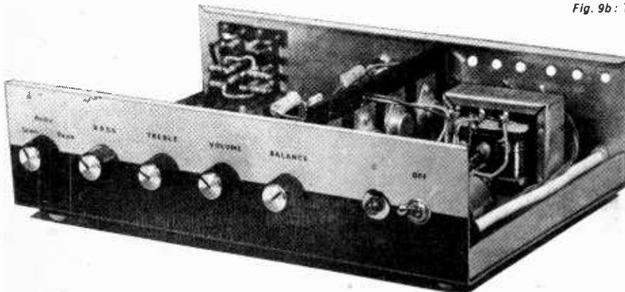
to create stray coupling and hence r.f. feedback. The cure would be to connect a by-pass capacitor of 100-250pF from collector of Tr2 to Tr3 to chassis.
