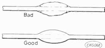
Fig. 1: Many dry joints exhibit an inward curve where the solder meets the wire (top). A smooth contour from wire to solder is usually the sign of a good joint (bottom).
