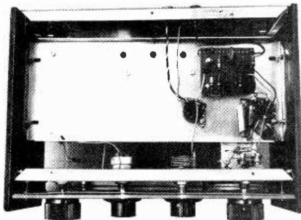
Only the mixer-oscillator board and associated coil holders are mounted underneath the chassis.
