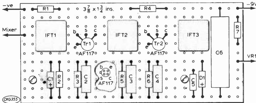
Fig. 6: Layout of components on the i.f. amplifier board and lead-out connections for the AF117 transistors.
