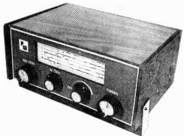
General view of completed receiver with metal strap fitted to lift front edge.
