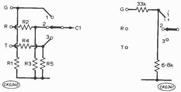
Fig. 7b (left): The circuit of the input selector section. Fig. 7c (right): Modification for a ceramic pickup.
