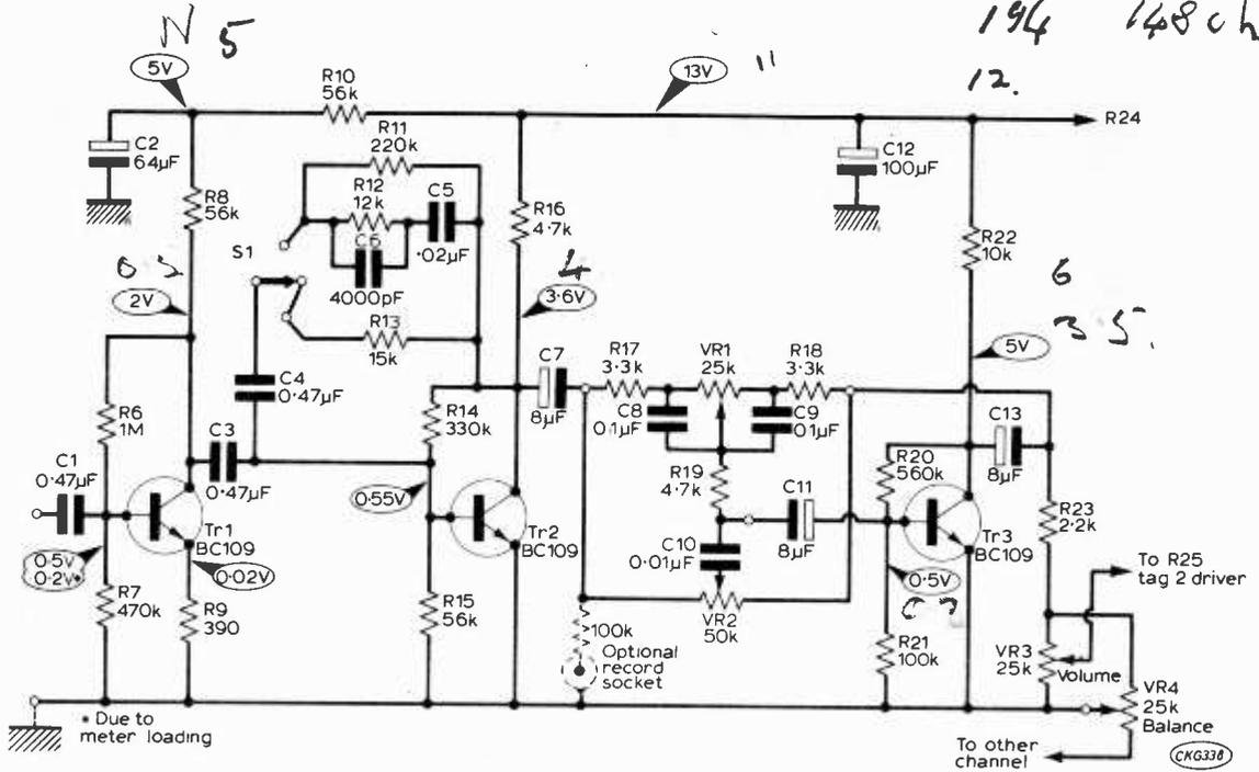
Fig. 6b: The circuit of one channel of the preamplifier. The decoupling components in the positive line are common to both channels.
