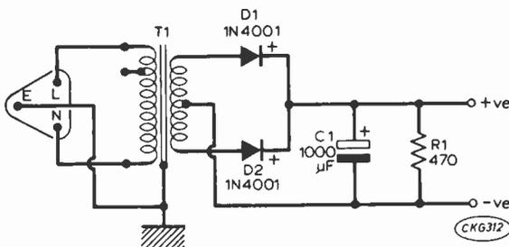
Fig. 1: The circuit of the battery eliminator.
