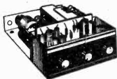
A superb solid state audio amplifier. Brand new components throughout. 5 silicon transistors plus 2 power output transistors in push-pull. Full wave rectification. Output approx. 13 watts
