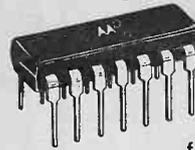
From Motorola, a monolithic dual stereo preamplifier for low noise
