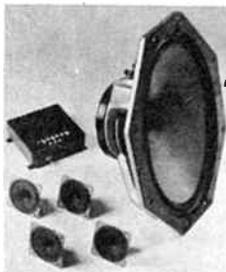
**15" 14A/780.** Bass unit on a rigid diecast chassis. Superior cone material handles up to 50 watts RMS, and is treated to give a smooth frequency response. Resonance 30 Hz. Flux 360,000 Maxwells. Impedance at 1 kHz is 8 ohms. 3" voice coil.
