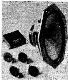
**15" 14A/780.** Bass unit on a rigid diecast chassis. Superior cone material handles up to 50 watts RMS, and is treated to give a smooth frequency response. Resonance 30 Hz. Flux 360,000 Maxwells. Impedance at 1 kHz is 8 ohms. 3" voice coil. Rec. retail price £40.80.
