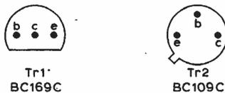
Fig. 5: Transistor base connections.
