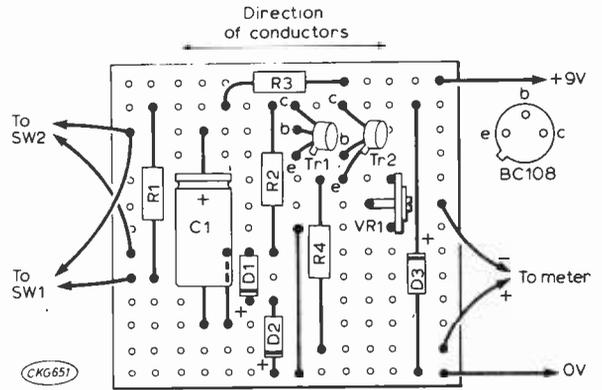
Layout of circuit on Veroboard. No breaks are necessary in the copper rails.
