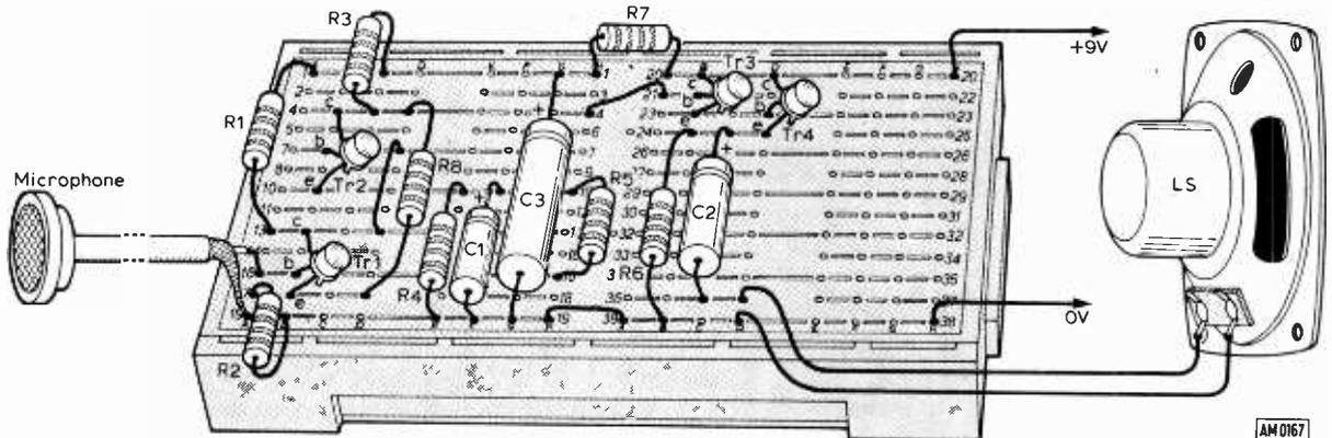
Fig. 58: Component layout for Fig. 57.
