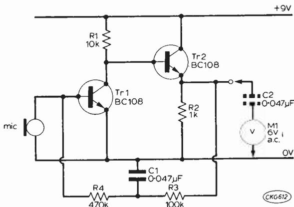
Fig. 51: The signal level at Tr2's emitter is comparable to that produced by the circuit of Fig. 45.
