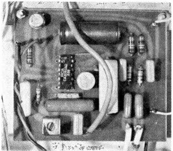
A view of the completed Stereo Decoder board.
