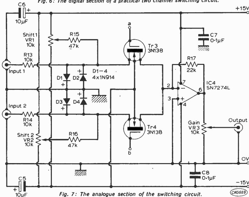
Fig. 7: The analogue section of the switching circuit.
