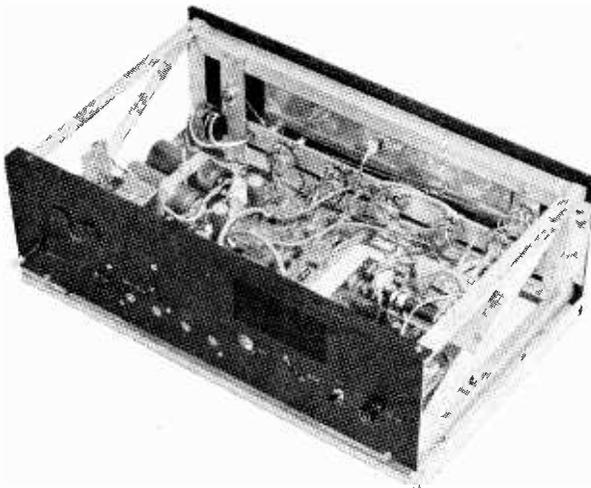
is spray painted. After marking and drilling all holes the paper coating on the rear side is removed except for masked areas and several coats of cellulose paint sprayed on. The original was sprayed black.
