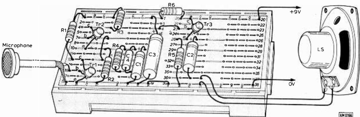
Fig. 56: Component layout for Fig. 55.
