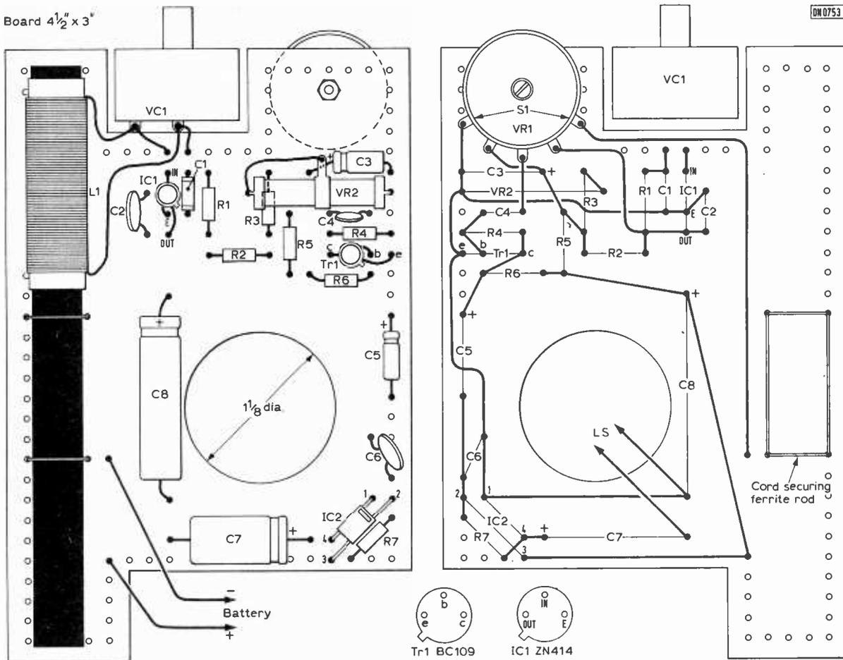
Fig. 2: Component layout and wiring. The circuit board is 0.15in. matrix plain Veroboard.
