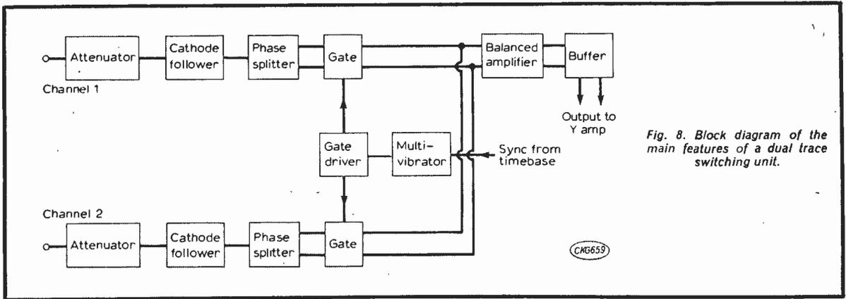
Fig. 8. Block diagram of the main features of a dual trace switching unit.
