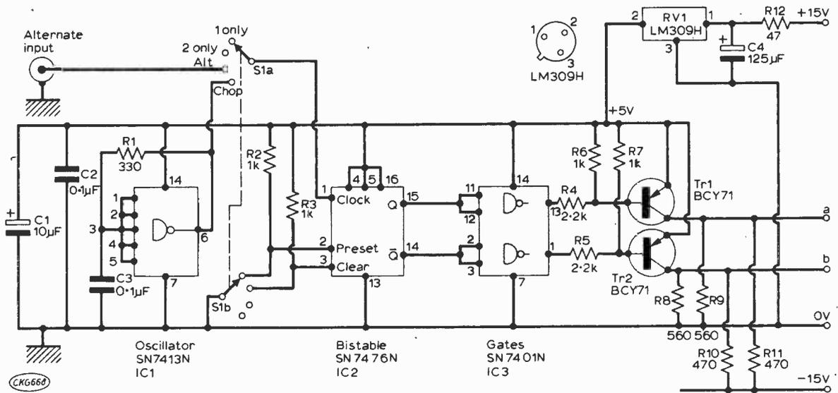
Fig. 6: The digital section of a practical two channel switching circuit.
