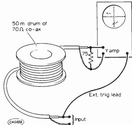
Fig. 7. Set-up using a 50m drum of co-axial cable as a simple delay line.
