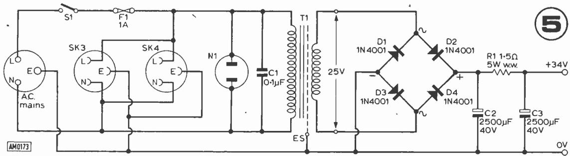
Fig. 19: Circuit of the Power Supply. C1 reduces interference from mains-borne transients.
