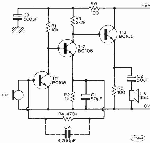
Fig. 55: This circuit has almost identical performance to that of Fig. 47 but is much more economic on components. Its gain, however, is uncontrolled and unpredictable.
