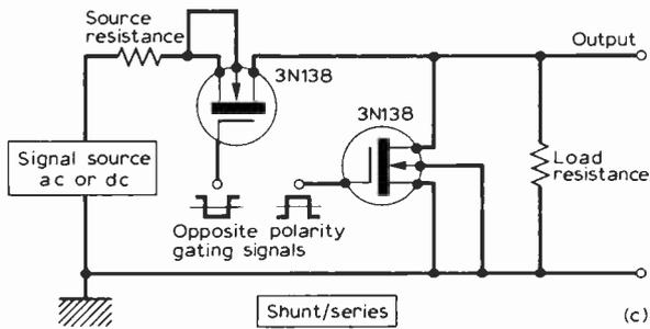
Fig. 2: Chopping circuits (a) shunt (b) series and (c) shunt-series.
