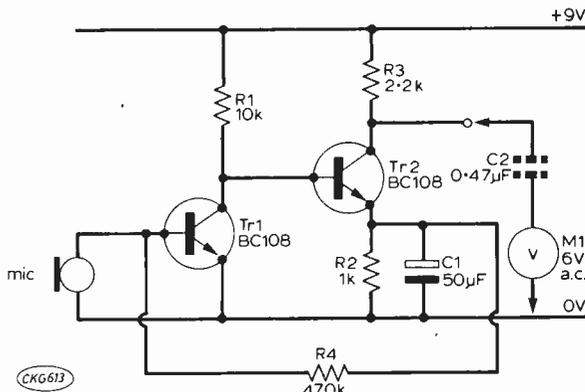
Fig. 53: The voltage gain of this circuit is similar to the first two stages of Fig. 47 but uses fewer components.
