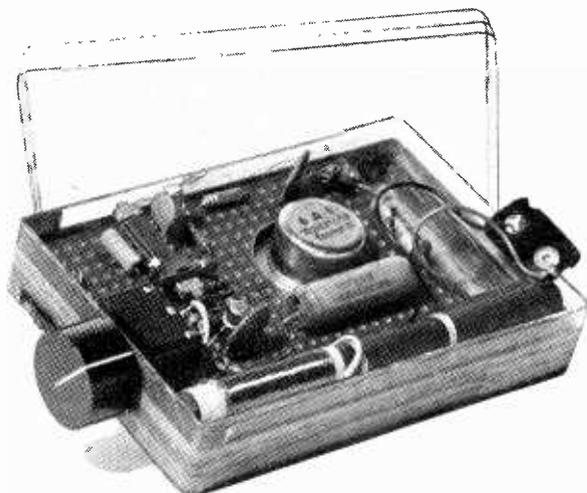
**T**HIS receiver is designed to fit the pocket, having the tuning control and edge-operated potentiometer and switch at one end of the case, so that there are no projections elsewhere. It provides good volume. The actual external dimensions are  $4\frac{3}{4} \times 3\frac{1}{4} \times 1\frac{3}{8}$  in., and this allows easy construction without cramping of the components.
