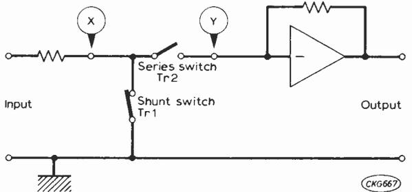
Fig. 5: A current mode shunt-series chopper circuit.
