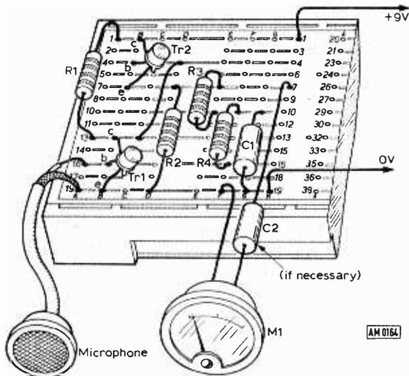
Fig. 52: Component layout for Fig. 51.
