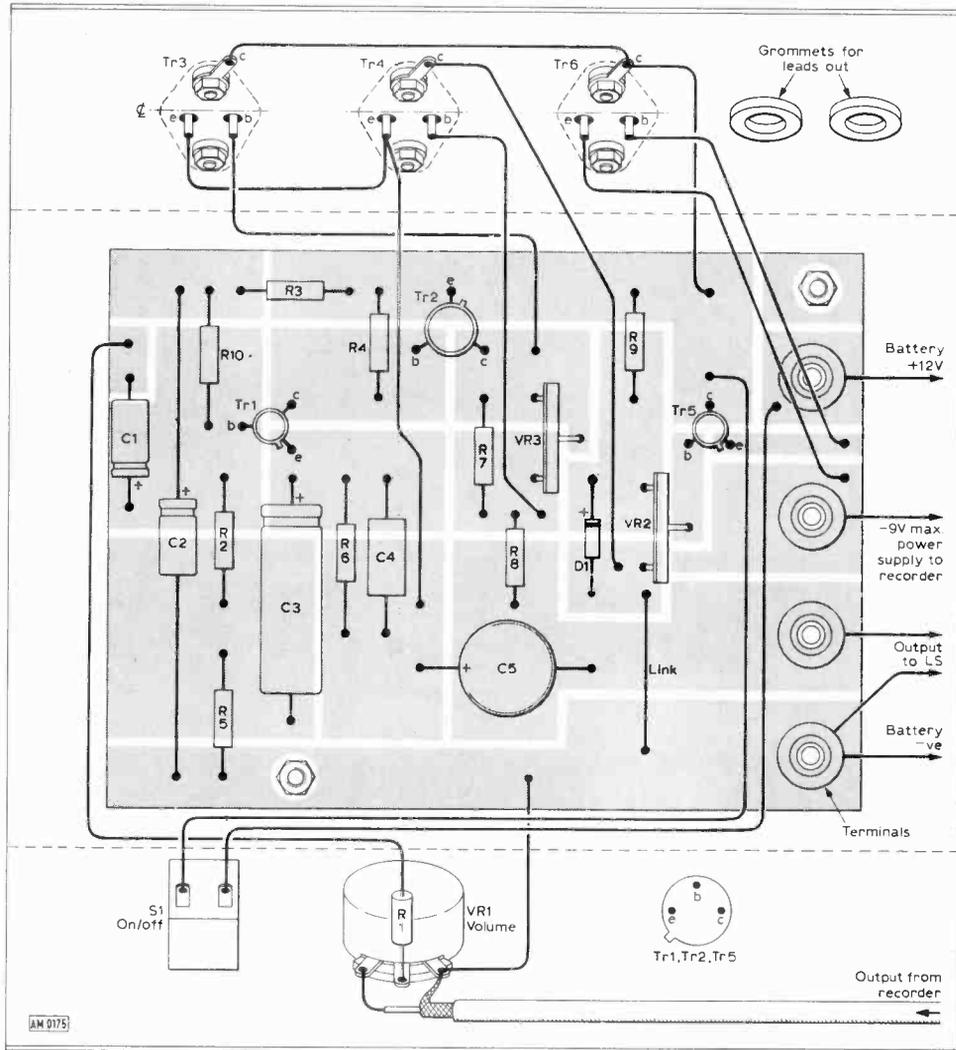
Fig. 3: (above) wiring of PCB to power transistors and volume control.
