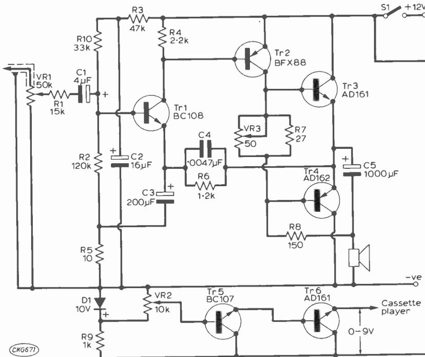
Fig. 1: (left) Circuit of the amplifier and power supply for the cassette recorder.
