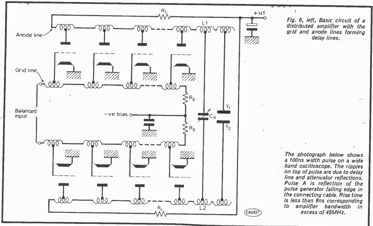
Fig. 6, left, Basic circuit of a distributed amplifier with the grid and anode lines forming delay lines.
