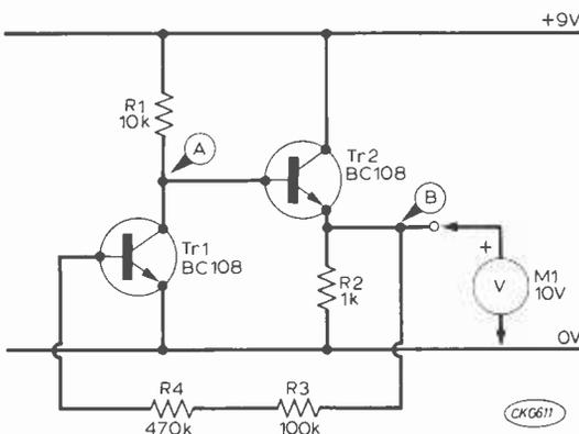
Fig. 49: Bias is derived from the output of the emitter follower.
