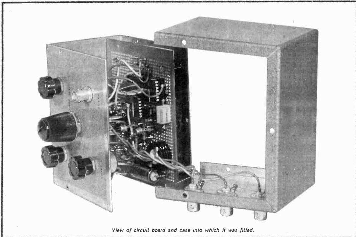
View of circuit board and case into which it was fitted.
