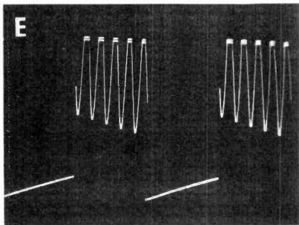
Photograph D, left, shows output of an amplifier driven by a 100Hz square wave and a 1kHz sinusoidal tone burst. Photograph E, above, shows same signals at a slightly higher power level so that clipping occurs. The difference in clipping levels occurs because of the 100Hz ripple on the power supply which is not synchronised with the tone burst.
