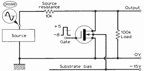
Fig. 4: Typical shunt chopper circuit using the 3N138.
