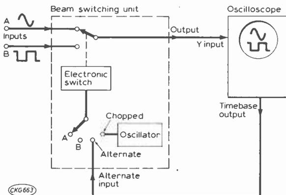
Fig. 1: Block diagram for an oscilloscope trace doubling unit.
