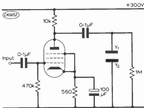
Fig. 1. Simple AC amplifier with asymmetrical output, not recommended for scope use.
