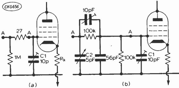
Fig. 5. (a) A simple direct attenuator and (b) a  $-10$  dB attenuator with compensating capacitors.
