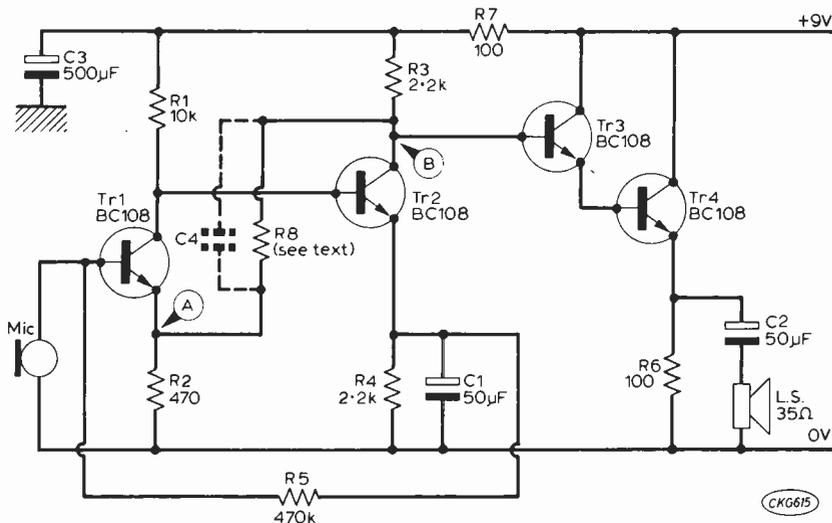
Fig. 57: A refined version of Fig. 55. The gain is set by the ratio of R8 with R2. R4 has a different value to increase the quiescent potential at Tr2's collector and a super alpha pair is used to drive the speaker—reducing the load on Tr2.
