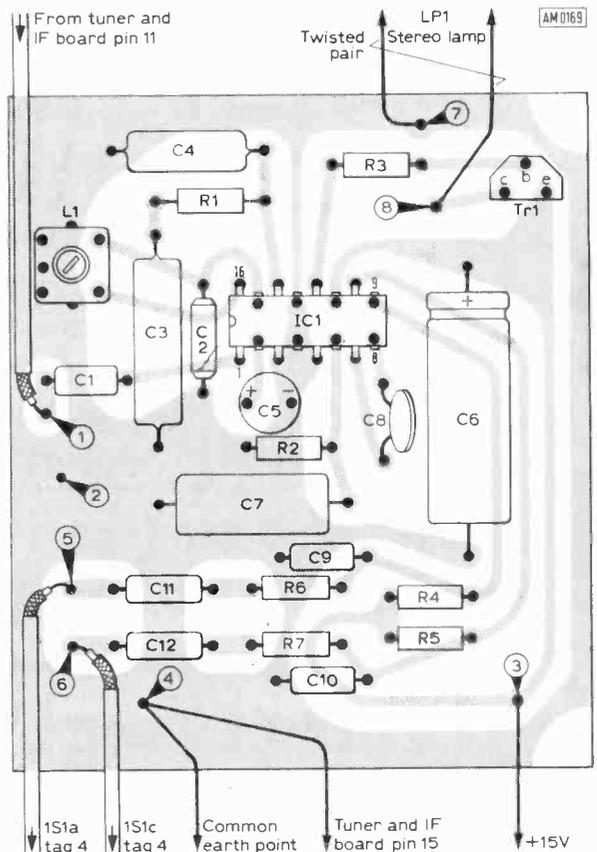
Fig. 15: Component location and printed circuit layout for the Stereo Decoder board. Both drawings are actual size.
