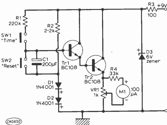
Circuit of the electronic timer using a meter to display the time interval.
