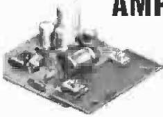
The AL10, AL20 and AL30 units are similar in their appearance and in their general specification. However, careful selection of the plastic power devices has resulted in a range of output powers from 3 to 10 watts R.M.S. The versatility of their design makes them ideal for use in record players, tape recorders, stereo amplifiers and cassettes and cartridge tape players in the car and at home.
