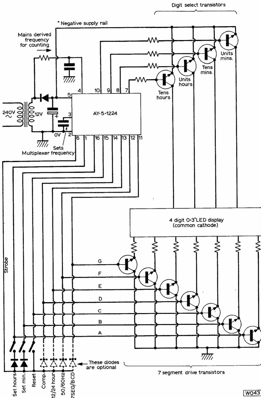
Fig. 1: General application circuit for the AY-5-1224 integrated circuit, emphasizing the few components needed externally.
