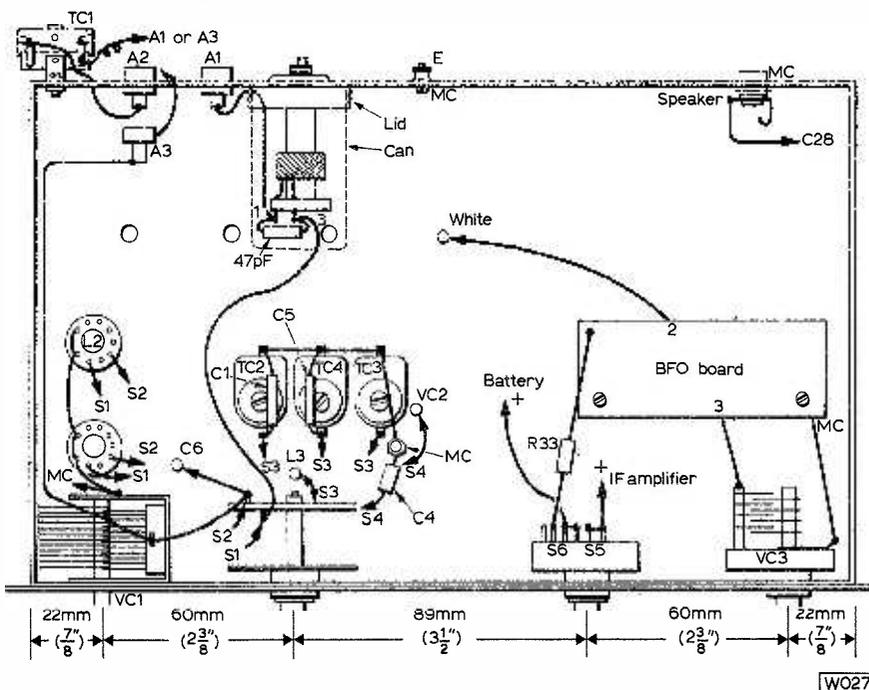
Fig. 9: Aerial tune (VC1), BFO pitch (VC2) and trimmers viewed from underneath. The diagram also shows the positioning of the BFO board and the three alternate aerial sockets, A1, A2 and A3.
