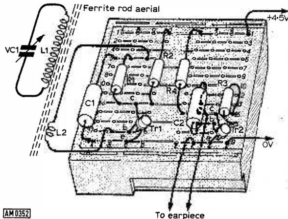
Fig. 117: Layout of circuit of Fig. 116.
