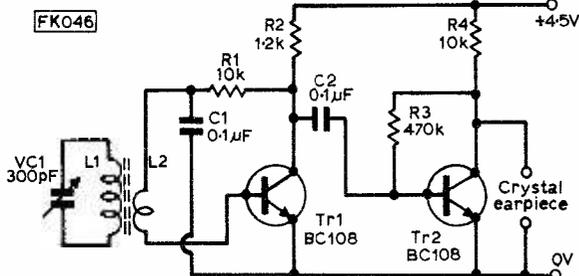
Fig. 116: Circuit modification to retain high Q of tuned circuit.
