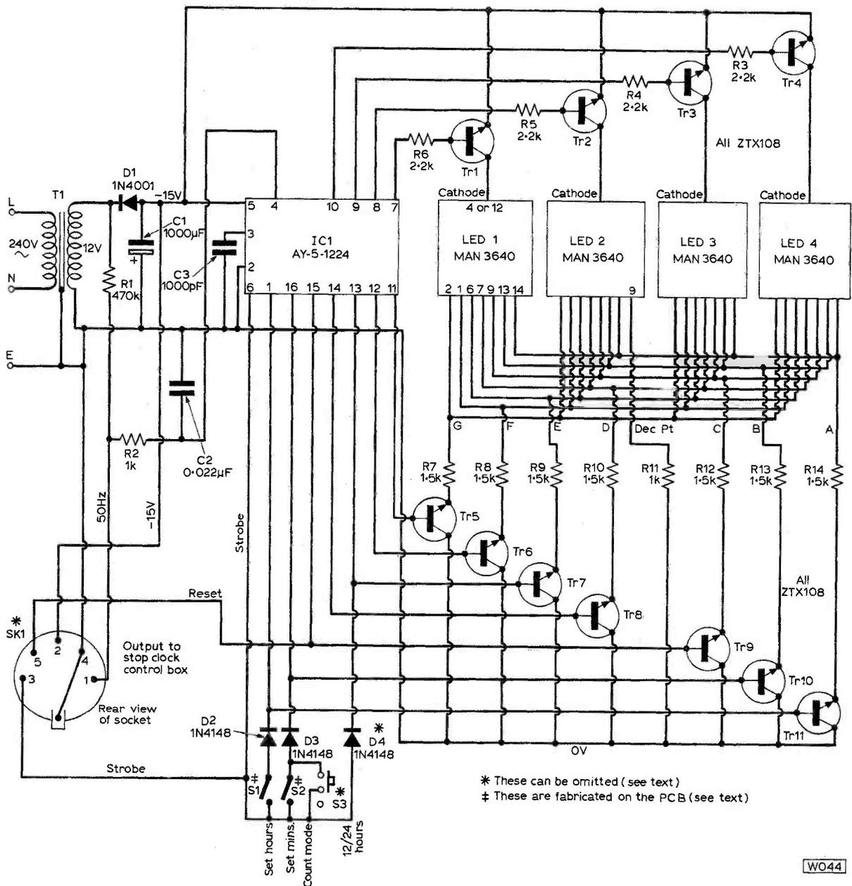
Fig. 2: Circuit of the clock described in the article, including the switch and socket required for the stop-clock facility.
