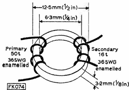
Fig. 4: Transformer T1, is of toroidal construction, efficient for broadband RF applications.
