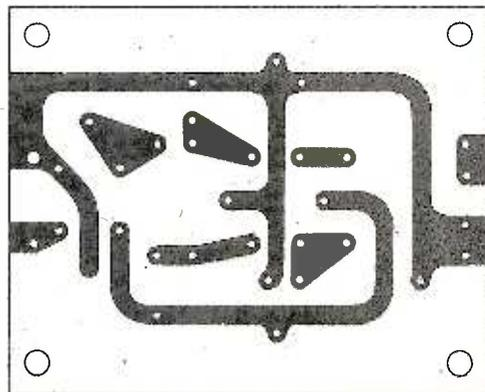
Fig. 5: PCB, full size, showing the component layout above and foil side below.
