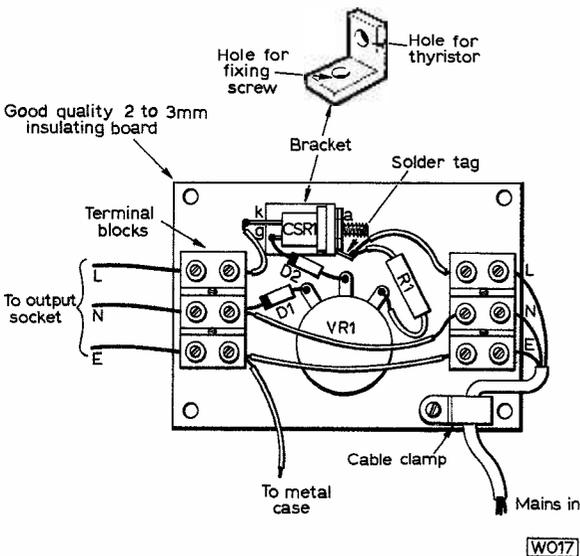
Fig. 2: Layout of the components in the Motor Speed Controller. Note that the bracket holding the thyristor will be live.
