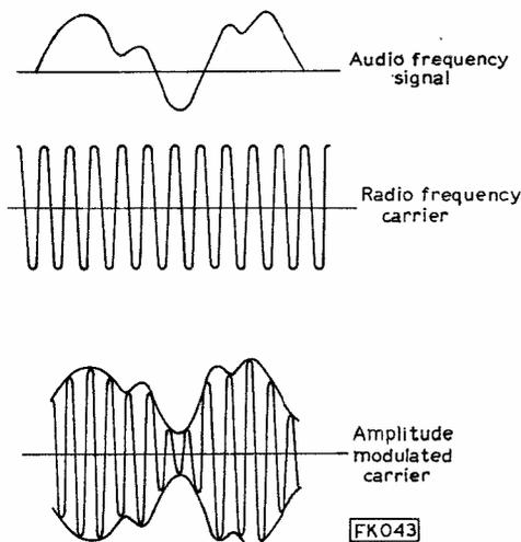
Fig. 112: Formation of an amplitude modulated (AM) signal from audio and RF sources.
