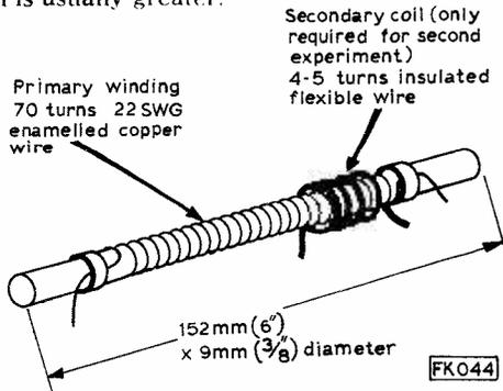
Fig. 113: Construction of aerial coil on ferrite rod, used in experiments shown here.
