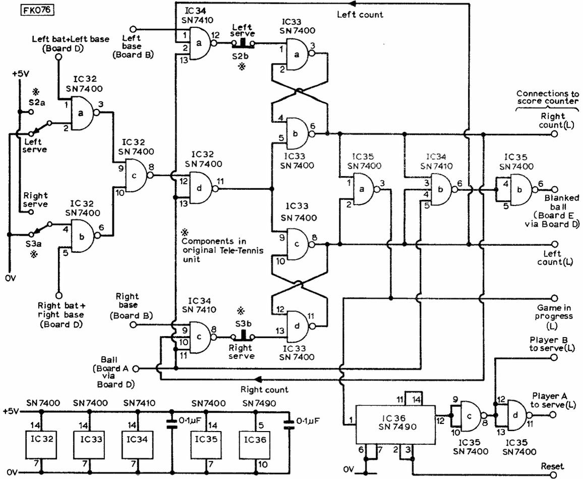
Fig. 1: Logic diagram of Board G which contains the new Serve/Lose logic. The (L) after some of the signals indicates negative logic (logic 1 = 0V).
