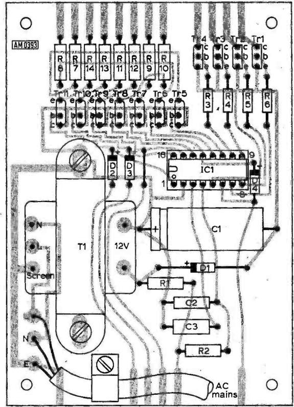
Fig. 5: Main PCB, left, actual size and component layout, right.
