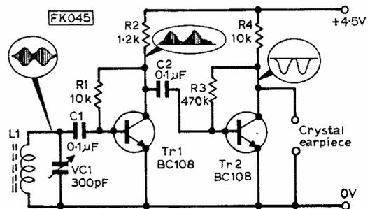
Fig. 114: First experiment, demonstrating effect of loading on coil Q.
