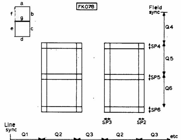
Fig. 4: An enlarged section of the score display which shows the timing of the various segments which go to make up the characters. The smaller character at top left shows the segment designation referred to in the text.
