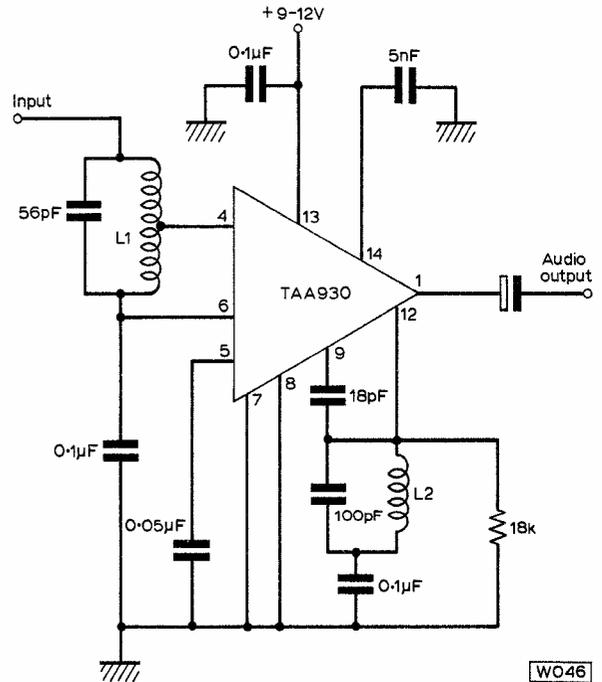
Fig. 1: A typical circuit using the TAA930 integrated circuit in a television sound system.
