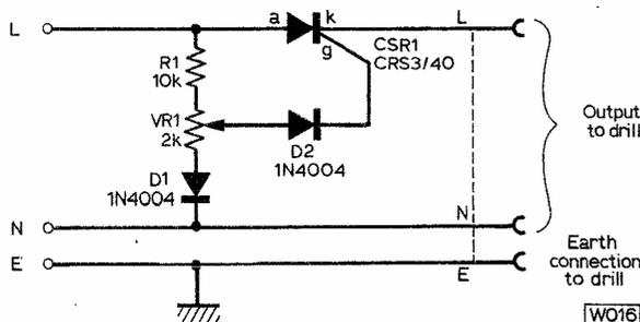
Fig. 1: Circuit diagram of the Motor Speed Controller.
