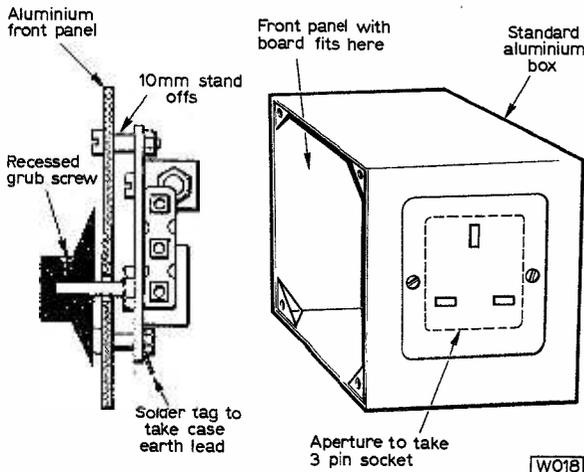
Fig. 3: Suggested "safe" method of housing the Motor Speed Controller.
