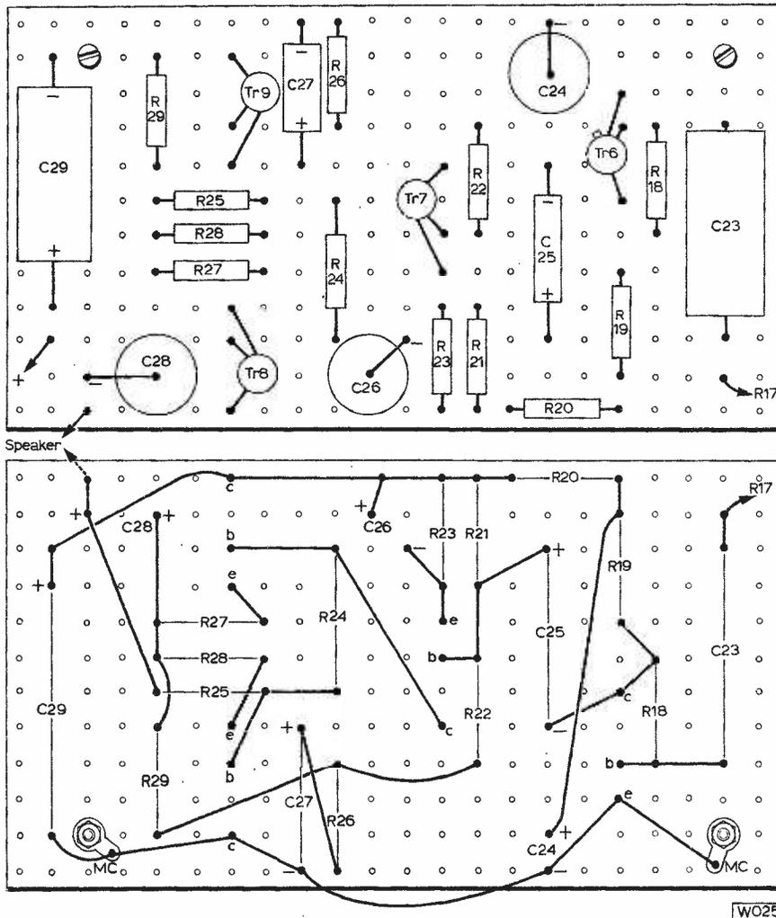
Fig. 7: Audio amplifier board, showing both component side and wiring side. Recommended speaker impedance for this circuit is 15Ω, although a jack socket is provided for headphones should they be preferred.
