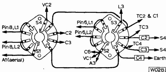
Fig. 10: Bandswitching for the Dual Conversion receiver is achieved with the wafer switch shown above. In the prototype only one wafer was used with contacts mounted both sides.
