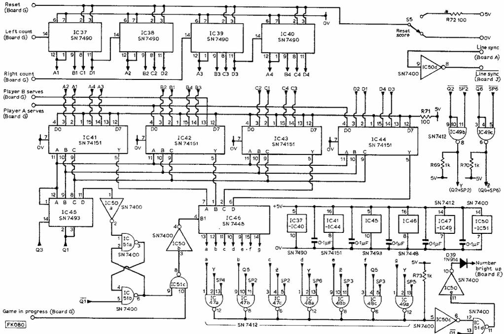
Fig. 5: Logic diagram of Board H, the character generation board. S5 is a new component which can be mounted on the front panel.
