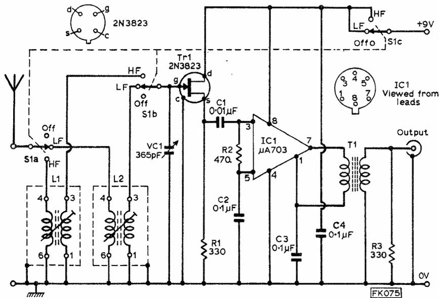
Fig. 3: Complete circuit diagram of the SW Pre-amplifier giving details of IC1 ( $\mu$ A703) and Tr1 (2N3823) base connections.
