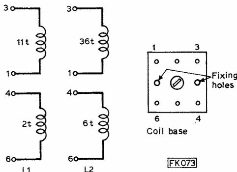
Fig. 2: L1/L2 coil winding details and pin configuration.
