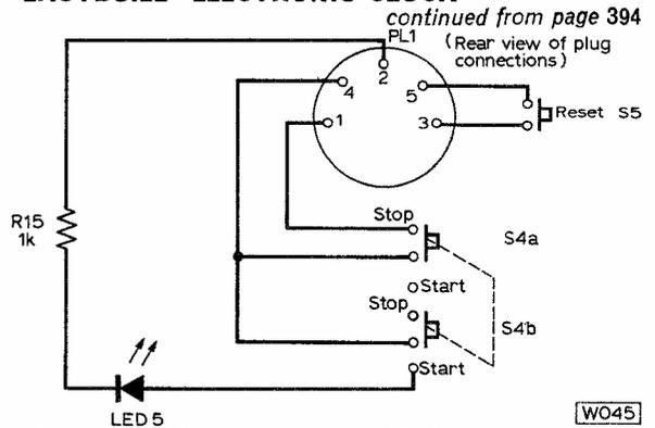
Fig. 6: Circuit of the remote control unit for the stop-clock facility. [W045]
