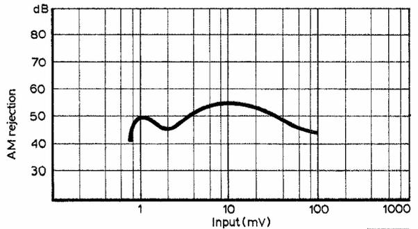
Fig. 2: AM rejection plotted against input voltage.
