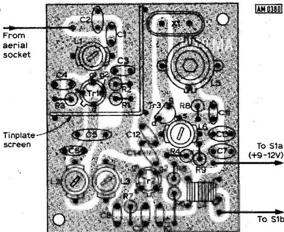
Component side view of the PCB, shown approximately 1½ times actual size. For components to fit the hole spacings correctly, the leads should be kept as short as possible.
