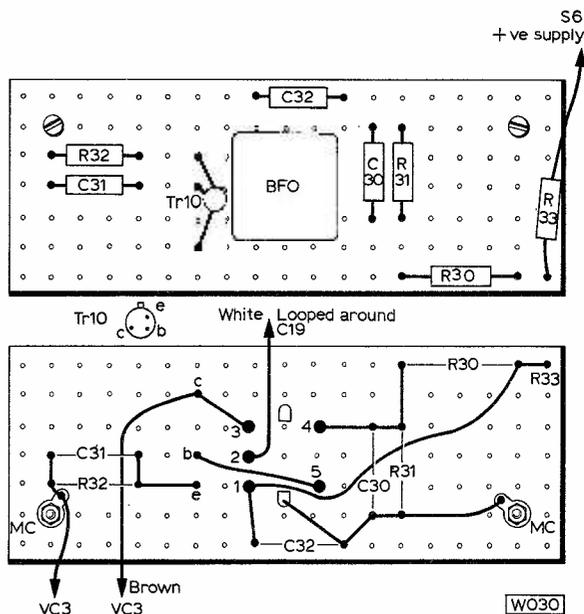
Fig. 12: Underside and topside of BFO board. The output signal is taken via an insulated lead, looped around C19.
