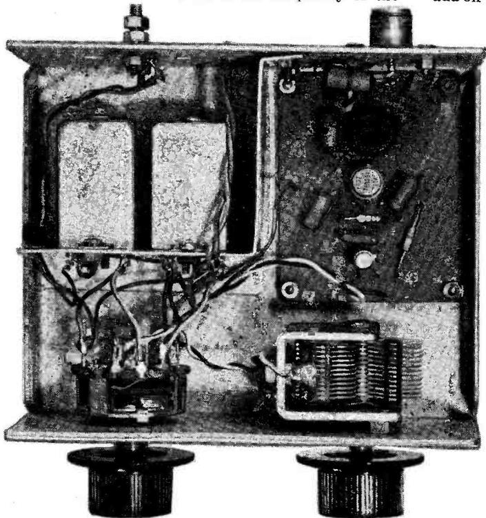
*Interior view from above, of the 'U' shaped chassis, showing details of the PCB, coils and switch layout. The two coils, L1/L2 are mounted on a small screen with their bases towards the front panel to facilitate short wiring.*
