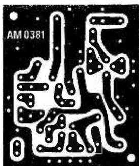
Fig. 2: Full size drawing of the printed circuit board viewed from the underside. Owing to its small size, considerable care should be taken in the drawing and etching of this board.
