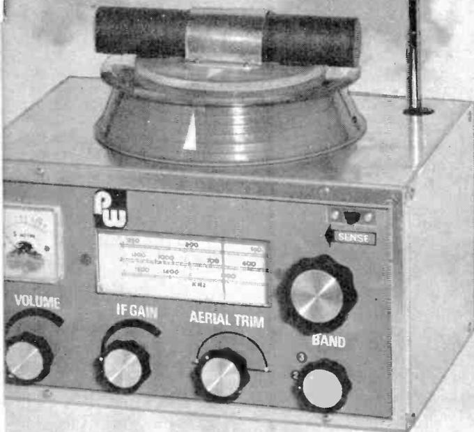
The sense aerial is then used to provide another signal. With one position of the ferrite rod, signals from both aerials will combine, giving a greater meter deflection than the other position, where ferrite aerial and sense aerials are out of phase. By this means it is possible to find which bearing is correct of the two minimum readings obtained without the sense aerial.
