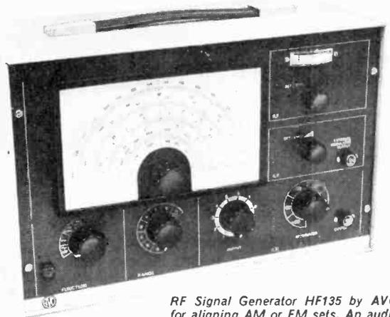
RF Signal Generator HF135 by AVO for aligning AM or FM sets. An audio output is also available.
