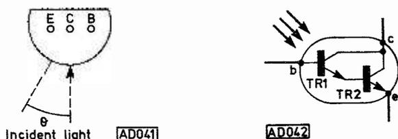
Fig. 1: (left): Encapsulation of the 2N5777. The device is most sensitive to light arriving along the direction of the arrow.
