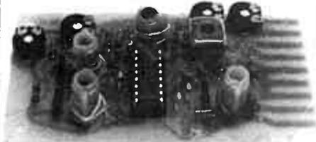
The EF5400, the first VHF tunerhead with one IC. It includes PIN diode agc loop, balanced osc/mixer, RF stage. Tunes 88-108 with only 2-8v DC bias, and is adaptable up to 230MHz. £9.75 built/tested. Special frequency ranges on applic.
