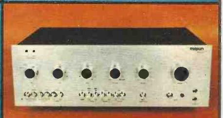
A very high quality 40W per channel stereo amplifier with a superb specification and lots of extras. Full construction details in our catalogue.
