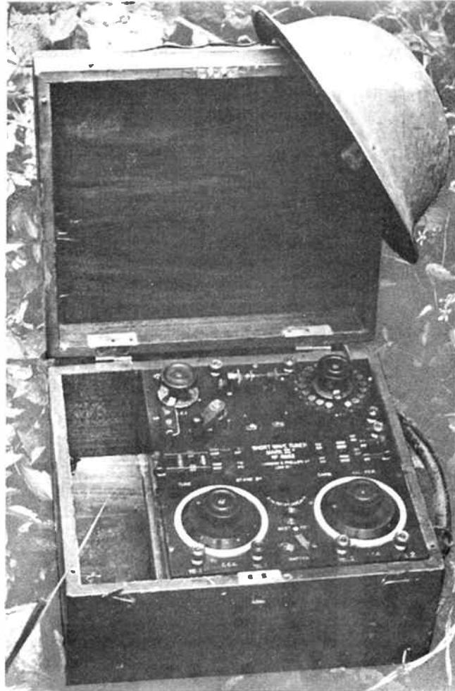
Fig. 3: Short-wave Tuner, Mark III made by Johnson and Philips
