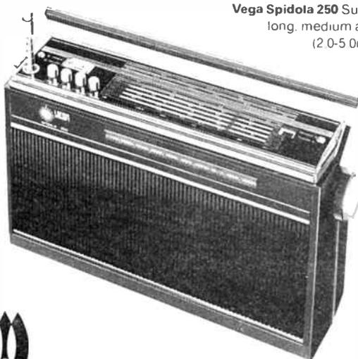
**Vega Spidola 250** Superhet portable receiving VHF/FM, long, medium and 6 short-wave bands: 150-60m (2.0-5.0mHz), 60-40.5m (5.0-7.4mHz), 31.6-30.7m (9.5-9.77mHz), 25.7-24.8m (11.7-12.1mHz), 19.85-16.75m (15.1-17.9mHz), 14-13.8m (21.45-21.75mHz).
