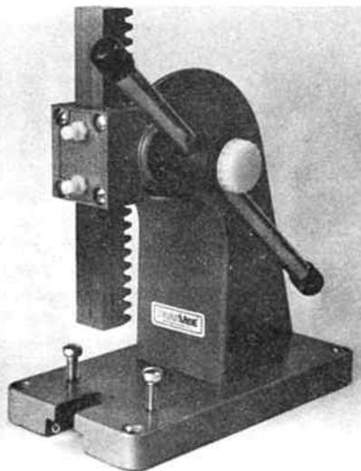
178mm high, is ideal for pressing bearings, forming and assembling small parts, staking rivetting and broaching. Built to stand the rigours of daily production line usage, the press has a rated capacity of 500psi.
