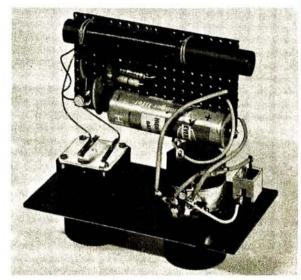
General view of the tuner showing the rod aerial fixed to the board with fine thread.
