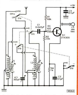
Circuit of the Booster which uses a single transistor and an external aerial. An earth connection will often help to increase the signal even further.
