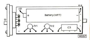
Having got the size of the board right the parts can be fitted as shown here. The battery wires are soldered to the battery contacts. A battery holder would take up too much space.
