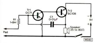
The circuit of the Rain Warning Bleeper could hardly be simpler. Altering the values of R1 and/or C1 will change the tone.
