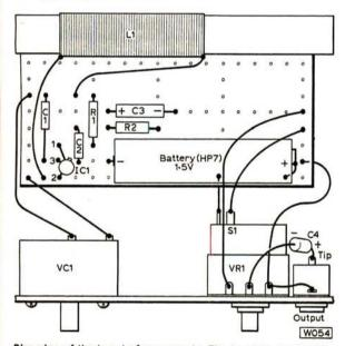
Plan view of the layout of components. The board is connected to VC1 and S1 by heavy copper wires.
