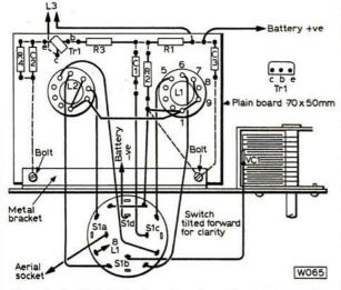
The parts should be laid out as shown here. The switch is, in fact, mounted on the vertical part of the metal bracket.
