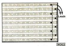
The size of the piece of veroboard used for the rain-detecting pad is not important but ensure alternative rails are connected as shown here.
