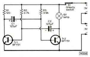
The simple multivibrator circuit is activated by the gravity switch S1. The operating current of the lamp should be as low as possible.
