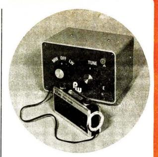
Here the output coil of the Signal Booster is placed close to the internal aerial of the transistor radio.
