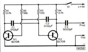
The Signal Injector also uses a multivibrator circuit the output of which is very rich in harmonics.
