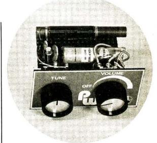
A single silicon integrated circuit provides several functions not normally available in TRF receivers.
