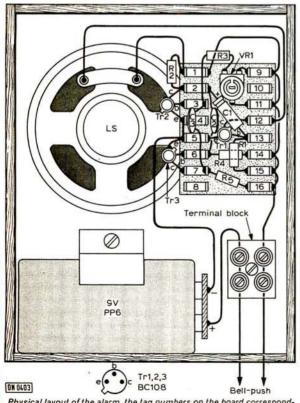
Physical layout of the alarm, the tag numbers on the board corresponding to those shown in the circuit diagram.
