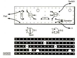
Position of the components and foil side of the veroboard showing breaks required to be made before assembly.
