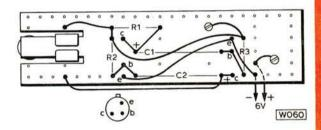
Layout of the components on a piece of plain veroboard and associated
