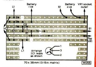
Diagram showing breaks required on the veroboard before components are soldered in place.
