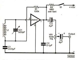
The tuner circuit using the ZN414 IC. Under no circumstances must the supply voltage exceed 1  $\cdot$  5V.
