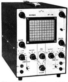
Brimar Group and has a very bright, clear, well defined display even at the fastest sweep speed of 200ns/div. The instrument is mains powered with a power consumption of approx. 10 watts. Overall dimensions of the black p.v.c. finished aluminium case are  $216 \times 165 \times 280$ mm deep and the cream-white front panel is silkscreened with black annotations.
