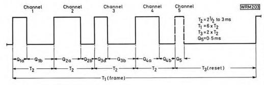
Fig. 1: The encoder output waveform showing the fixed frame length, the reset or synchronising pulse and the individual channel pulses (Q1a etc). Channel 5 is nonproportional and is intended for such applications as retracting undercarriages
