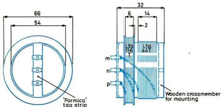
All coils 32s.w.g. enamelled copper wire wound in same direction
