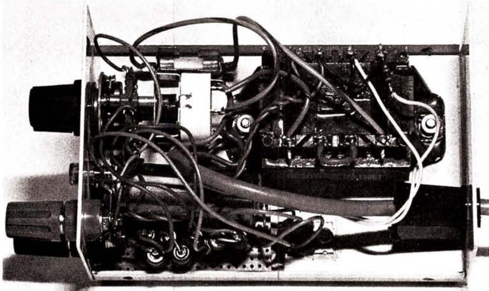
This picture shows the inside of the prototype NiCad charger. The layout is not critical and the more adventurous constructor could combine the charger shown here with the servo tester to be described in Part 7
