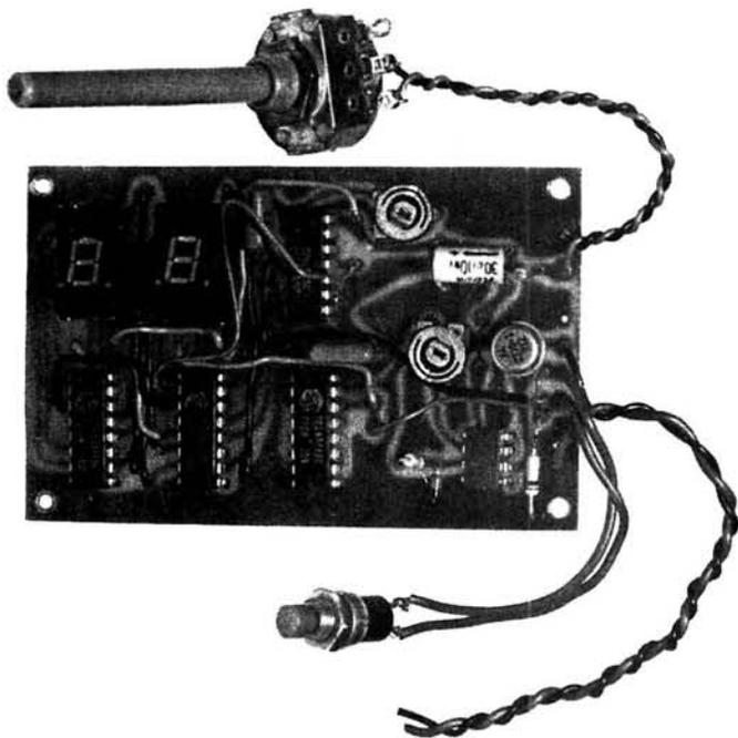
Accurate timing is essential in photographic practice if consistent results are required. The clock described in the following chapters was designed to cover the enlarger exposure and print developing stages in a black and white set-up. However, the clock would also be useful for timing colour processes or taking photographs where exposure times in excess of one second are involved.
