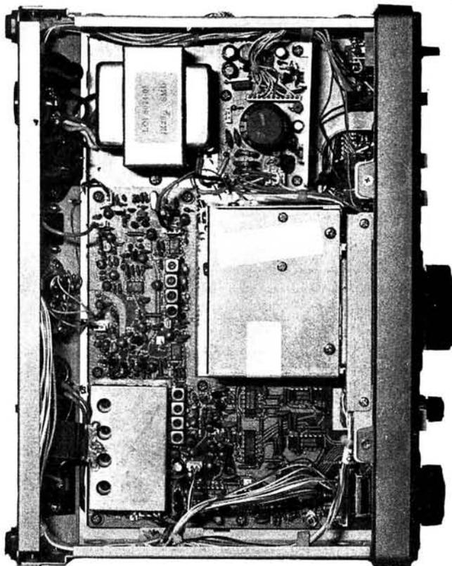
A bottom view, showing the p.i.l. synthesiser board, v.f.o. and power supply. All p.c.b.-mounted component references are marked on the board
