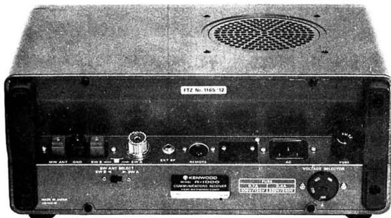
The rear panel is shaped so that the receiver can be placed close to a wall with the external connectors fitted
