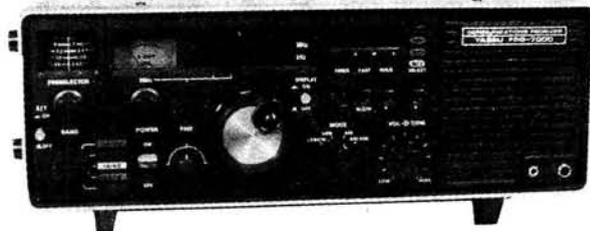
● 0.25 Thru 29.9MHz Coverage with 1kHz Readout
