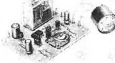
**KS470 SOUND OPERATED SWITCH.** Complete with dynamic microphone, adjustable sensitivity, relay - 1 pole change over contacts rated at 5 amp, operates from 9-12V D.C. semiconductors 2 x BC208 & 1 x I.C. 741. **£11.22 Inc VAT**
