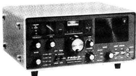
The FRG7 is a precision-built all-purpose communications receiver, featuring solid state construction for long life and high performance. It utilizes a Wadley Loop drift cancellation system, for high sensitivity, image rejection and stability.
