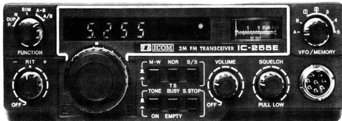
**25 Watts – 5 Memories – Scanning – 600kHz AND User Selectable Repeater Shift – Full Coverage in 5kHz or 25kHz Steps**
