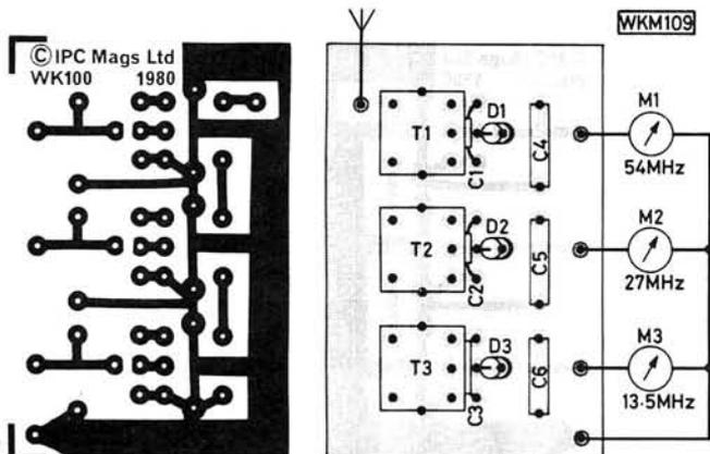
**Fig. 5: The copper track pattern of the wavemeter p.c.b. shown here full size. Fig. 6 (above right): The component placement drawing of the wavemeter p.c.b. Ambit International will be able to supply ready built and aligned boards for those constructors without the necessary gear**
