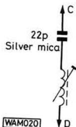
**Fig. 1: A 72MHz trap. The coil is 4 turns of 22 s.w.g. enamelled copper wire, wound on a 4.8mm diameter former fitted with a dust iron core**
