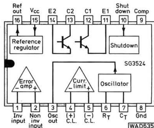
Fig. 1: The connections to the SG3524 device
