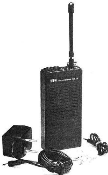
The AR-22 is a pocket-sized v.h.f. f.m. receiver tuning over a range of 141.000MHz to 149.995MHz, which includes, of course, the 2m amateur band. A phase-locked loop synthesiser
