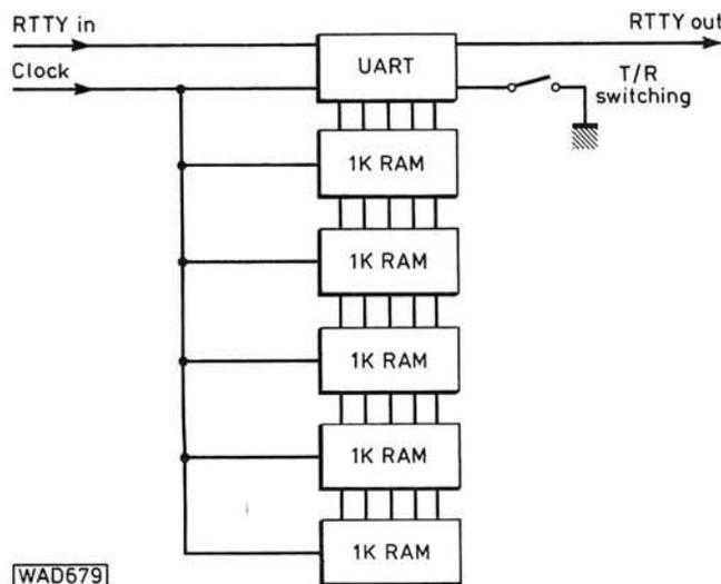
**Fig. 30: Basic block diagram of a 1K RTTY store**
