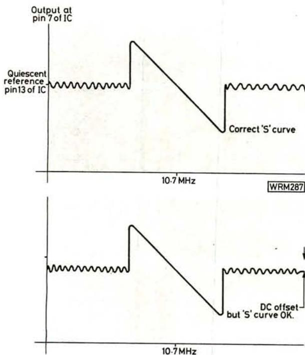
Fig. 18: The effect of a d.c. level shift at the f.m. detector
