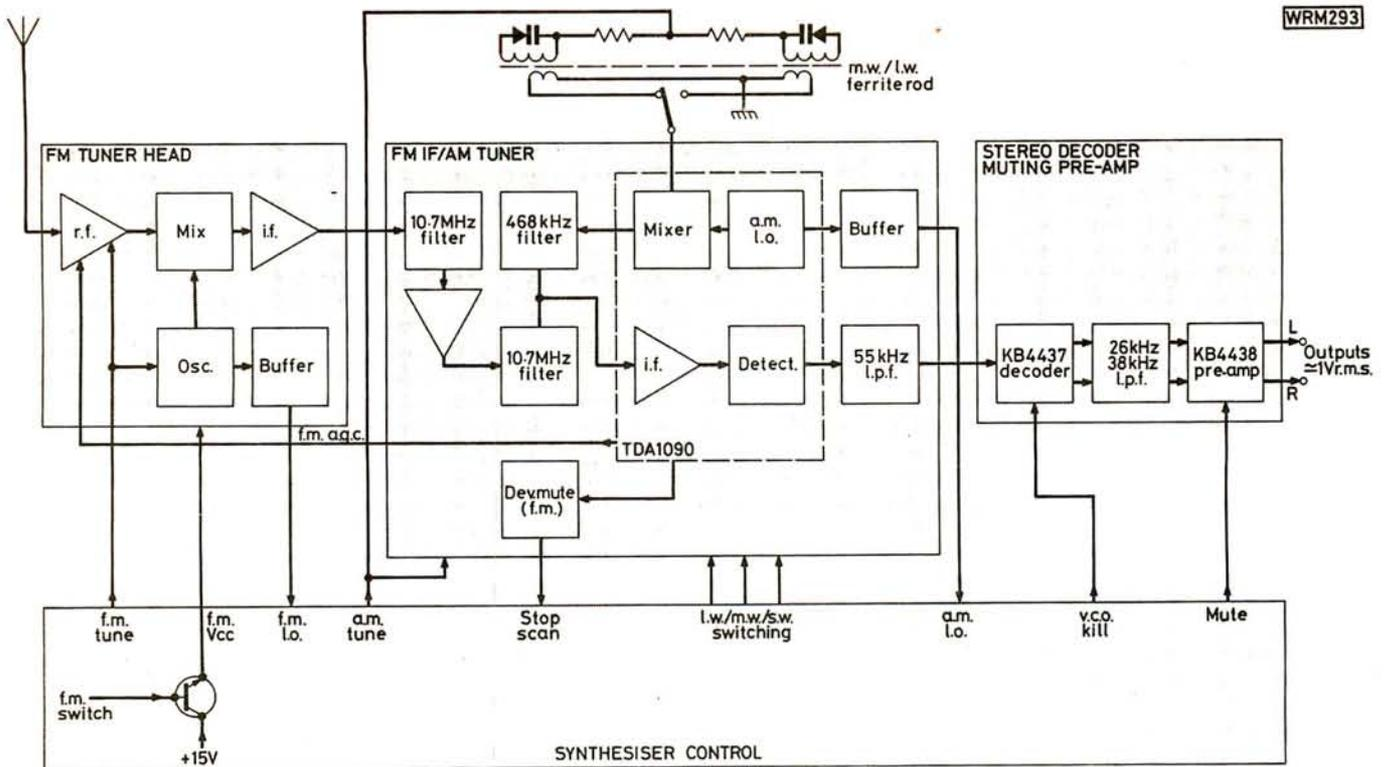
Fig. 11: Simplified block diagram of the complete tuner system
