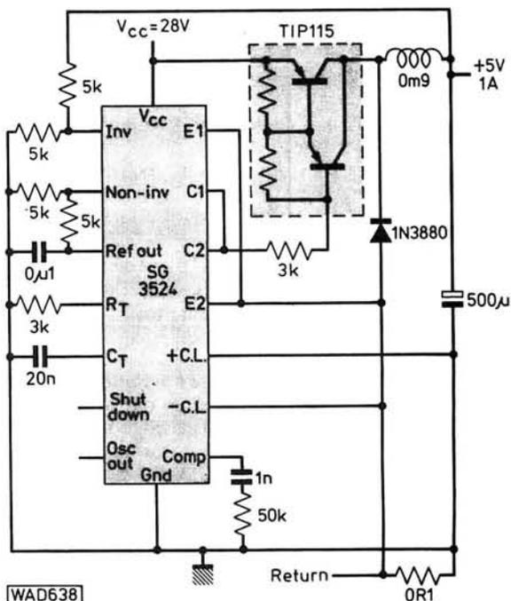
**Fig. 4: This circuit uses an external TIP115 Darlington to boost the maximum output current to 1A**
