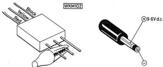
**Fig. 2 (left): Identifying leads to be shorted Fig. 3 (right): Polarity of the external power connector**
