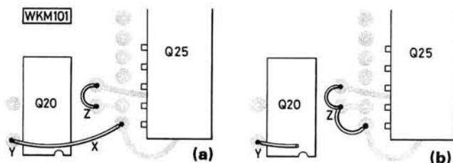
**Fig. 1: Extending the frequency range. In some later models Q20 (TC9122P) and Q25 ( $\mu$ PD 651C-13) are numbered Q14 and Q15 respectively**
