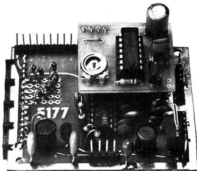
**The main d.f.m. board with the add-on unit in position. Note that some extra support for the add-on board will be needed and could be provided by the use of "Sticky Fixers"**
