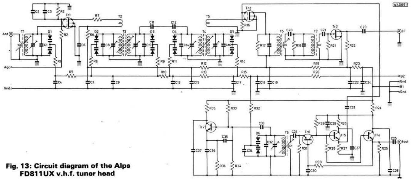
**Fig. 13: Circuit diagram of the Alps FD811UX v.h.f. tuner head**
