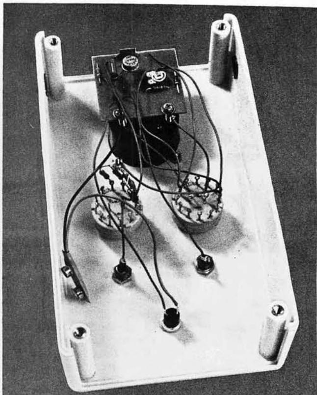
0-10V voltmeter which can be used to check the loaded supply potential. The battery should be replaced when this falls much below 8V.
