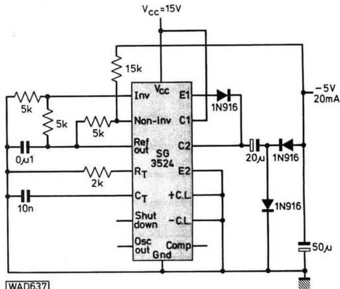
**Fig. 3: An inverter circuit providing an output of -5V, 20mA**
