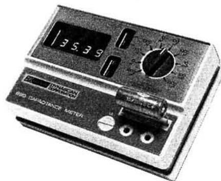
Accuracy is 0.5% or 1% of full scale, and resolution down to 0.1pF according to range.
