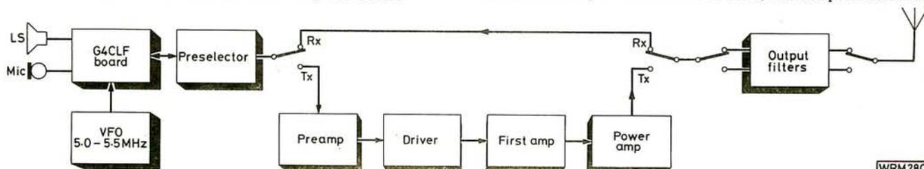
Fig. 1: The block diagram of the complete Helford transceiver
