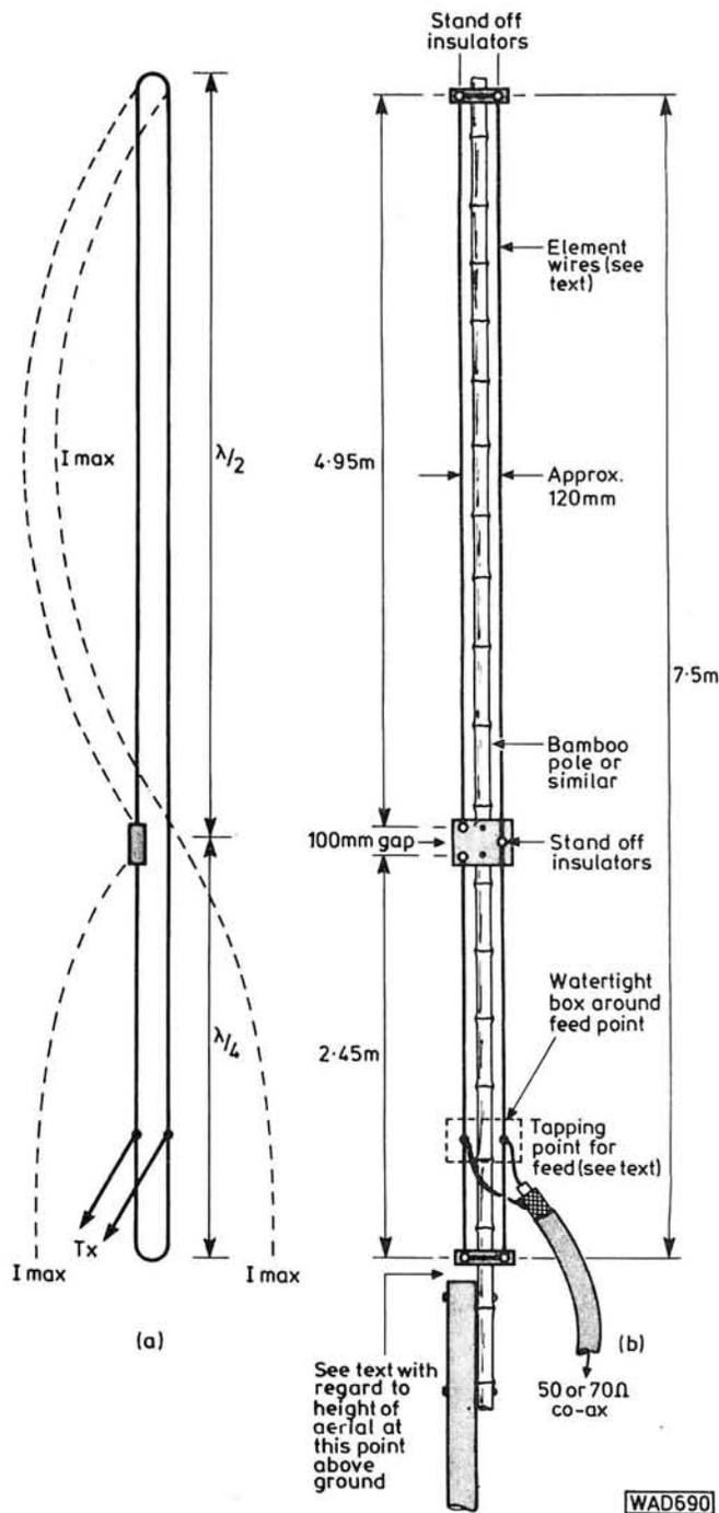
Fig 1: (a) Electrical function of the "Slim Jim" aerial. (b) Suggested method of constructing a "Slim Jim" for 28MHz (10 metres)
