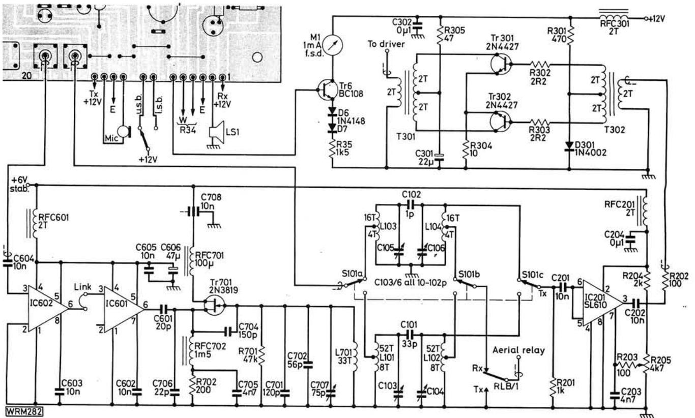
**Fig. 5: The circuit diagram of the external circuitry needed to operate the G4CLF Board. This is the complete PW Helford with the exception of the power supply and relay switching circuits**
