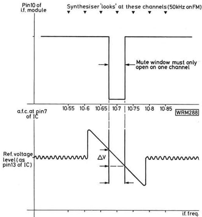
**Fig. 19: Deviation mute window determination. The values of R22 and R34 are chosen so that the a.f.c. voltage swing is sufficient to turn on Tr3 and Tr4 (Fig. 14) at the extremes of the mute window**
