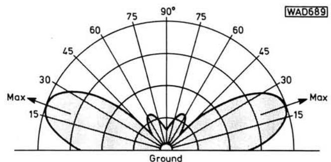
**Fig. 2: Approximate vertical radiation pattern when the centre point of the radiating section is  $\lambda/2$  above ground of good conductivity, and the aerial is situated in very clear surroundings**
