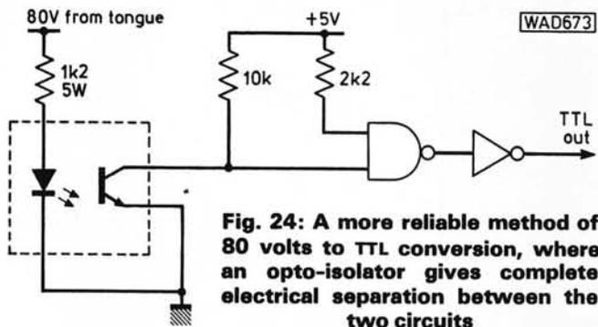
**Fig. 24: A more reliable method of 80 volts to TTL conversion, where an opto-isolator gives complete electrical separation between the two circuits**
