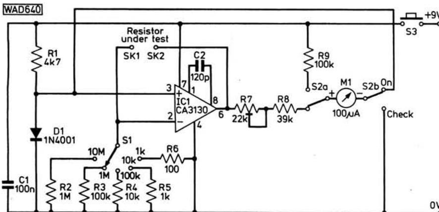
Fig. 2: The complete circuit diagram of the resistance meter
