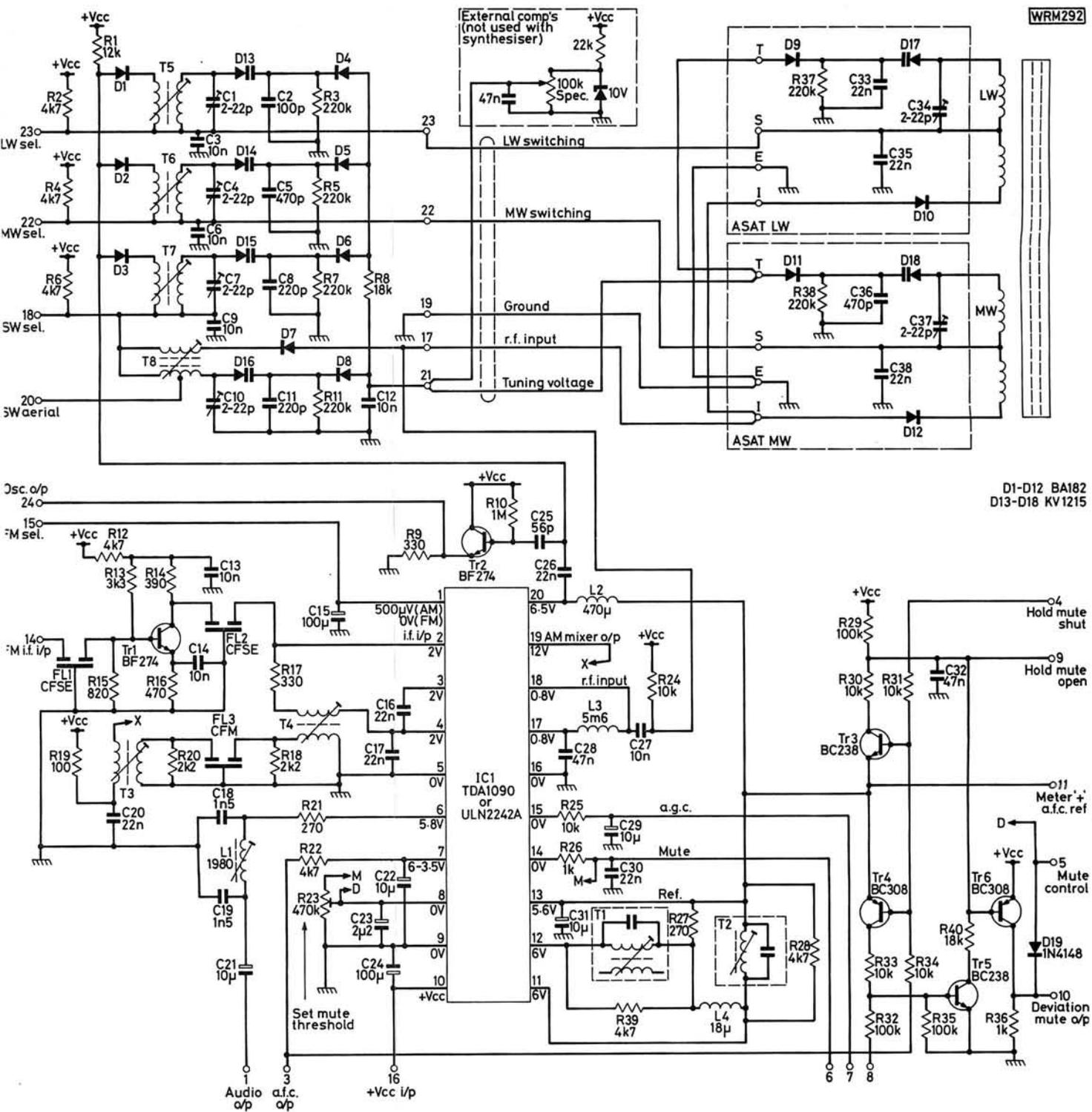
**Fig. 14: Circuit diagram of the f.m. i.f./a.m. tuner module, with associated remote tuned and switched ferrite rod aerial**
