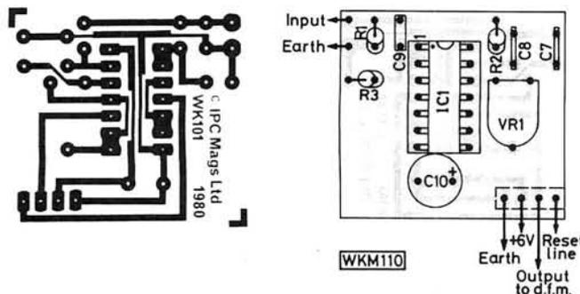
**Fig. 7: The copper track pattern of the add-on period measuring unit shown here full size. Fig. 8 (above right): The component placement drawing for the add-on unit. This board plugs directly onto the main d.f.m. board as shown in Fig. 4**
