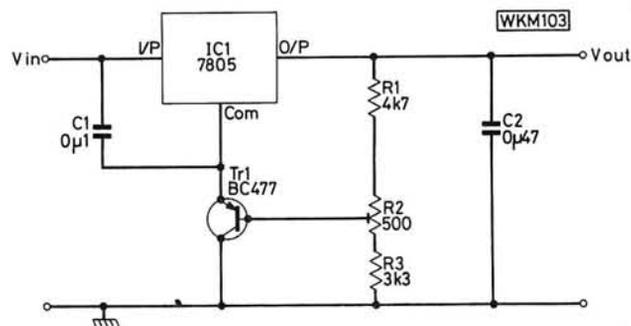
**Fig. 4: A stabiliser circuit capable of providing +9.6V at currents up to 1A from a 12V car battery supply**
