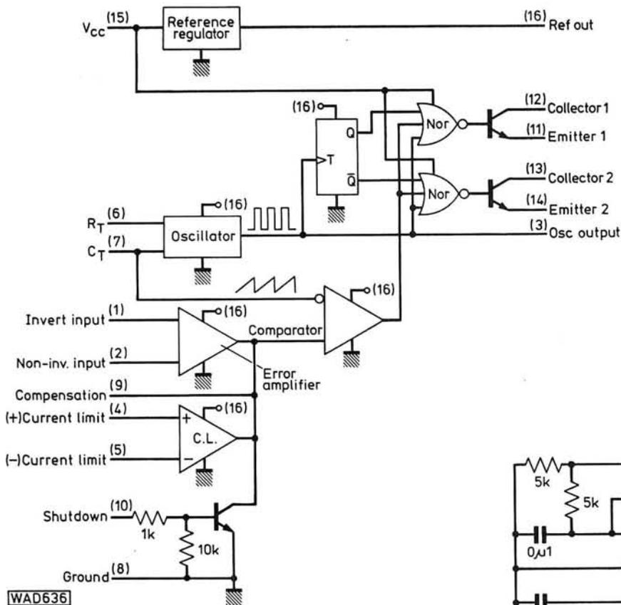
**Fig. 2: Internal circuitry, in block form, of the SG3524**
