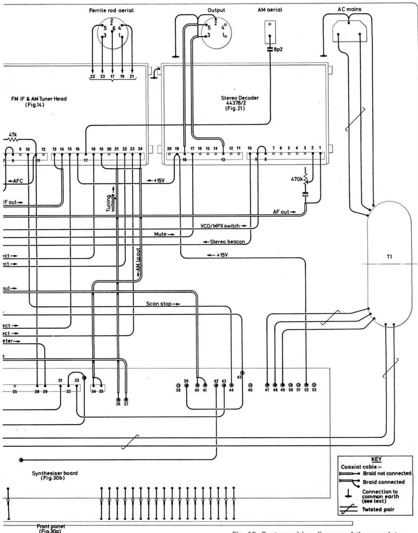
Fig. 10: System wiring diagram of the complete tuner, identifying signal flows and control requirements
