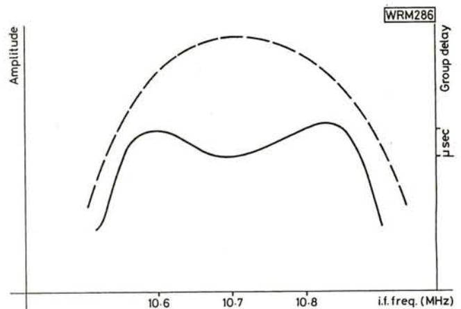
The crucial feature of any f.m. filter is the group delay (see Fig. 17)—which is related to the phase linearity by:  $\text{Group Delay} = \text{Phase change/frequency change}$ . The ideal phase change from one side of the filter to the other is a straight line. This is the same as the slope of the f.m. detector, which uses exactly the same principle when demodulating f.m. signals in a quadrature system, to convert frequency change into amplitude change.
