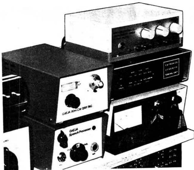
It is not necessary to build a terminal unit to join the ranks of RTTY enthusiasts, since commercial units are available. The intending purchaser can opt for a straight terminal unit, using the type of modulation and demodulation techniques discussed in earlier parts of this series, or a complete RTTY system.
