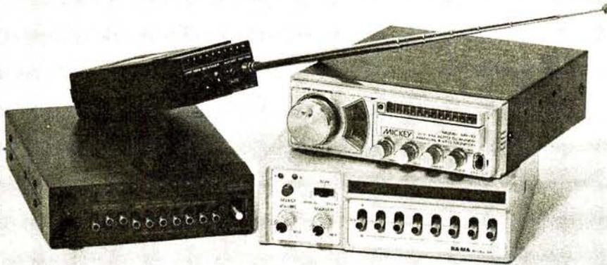
The MR-110, bottom left, is a v.h.f. scanning receiver intended for mobile operation, with 10-channel capability and lock-out facility. Sensitivity is  $0.8\mu\text{V}$  (20dB S/N) and the unit is powered from an external 12V source. Priced at £49 the MR-110 is supplied with crystals fitted for 5-channels extra.
