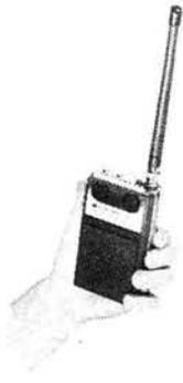
This 10 channel scanner out performs many of its rivals due to its highly sensitive front end and excellent filtering. A one channel 50MW transmitter is incorporated and is ideal for local use. Controls include squelch, volume, auto scan and manual channel stepping. The unit comes complete with channels S20, R1, R2, R7, Nicads, Charger, helical antenna and wire antenna.
