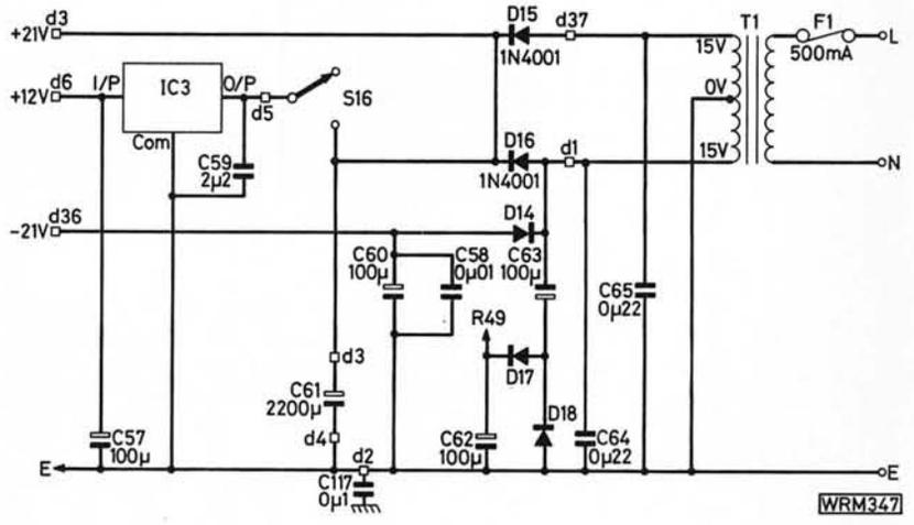
Fig. 1 (top): Circuit diagram of f.m. and TV sections of the PW Winton Tuner
