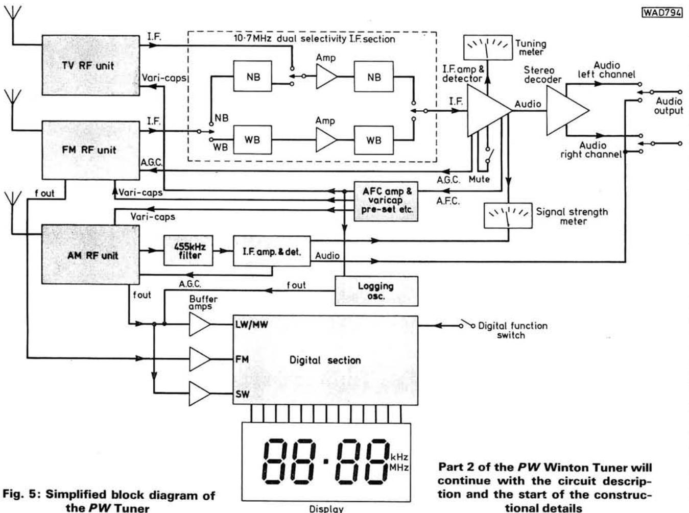
**Fig. 5: Simplified block diagram of the PW Tuner****Part 2 of the PW Winton Tuner will continue with the circuit description and the start of the constructional details**
