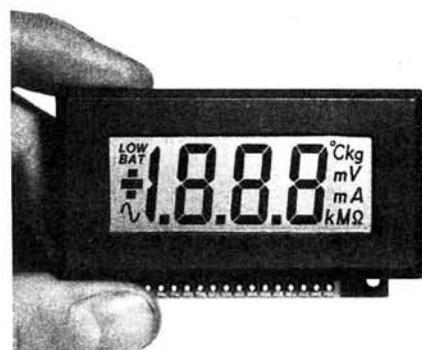
Other standard features include a digital hold facility, auto-zero, auto-polarity, external band-gap reference for maximum stability, single-rail supply of 5V to 15V d.c. drawing 200 $\mu$ A, programmable decimal points and a 200mV f.s.d.
