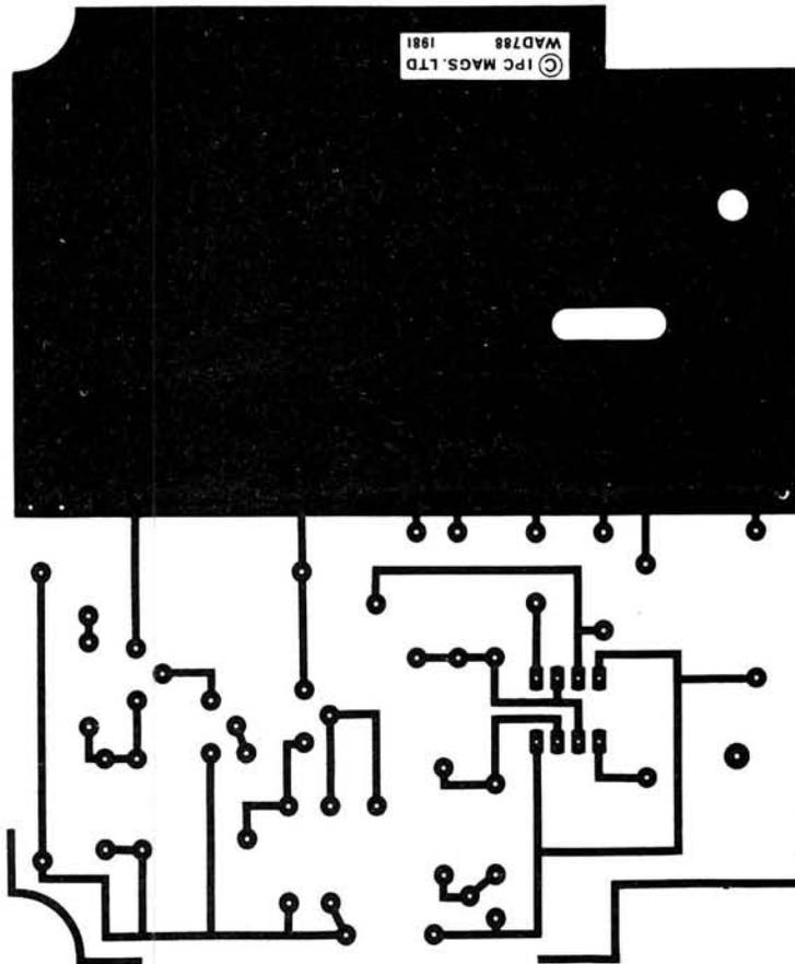
Fig. 4 (above): The copper track pattern of the p.c.b. shown full size. Fig. 5 (below): The component placement for the p.c.b.
