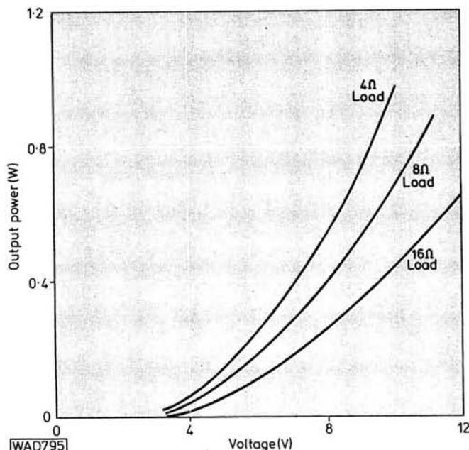
Fig. 1: Output power with varying supply voltage
