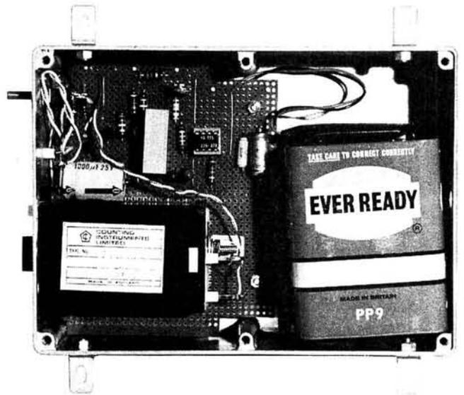
Internal view of the prototype engine hours counter. This unit was built using plain matrix board instead of the p.c.b. which was developed from the original layout
