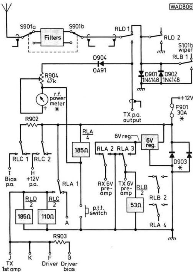
**Fig. 30 (above):** The circuit for the power switching of the PW Helford. D903 can be a single diode of, say, 50A current rating if available. If not then two 26A diodes may be used. The connection points referred to appear in Fig. 31, except F, G, H and I (see text)
