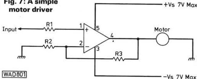
the amplifier are at the same potential; that is, when the input is at ground potential. As the input is made positive with respect to ground the motor will rotate in one direction, but when the input is made negative, the motor will rotate in the other direction. Resistors R2 and R3 set the gain and therefore the sensitivity of the circuit.
