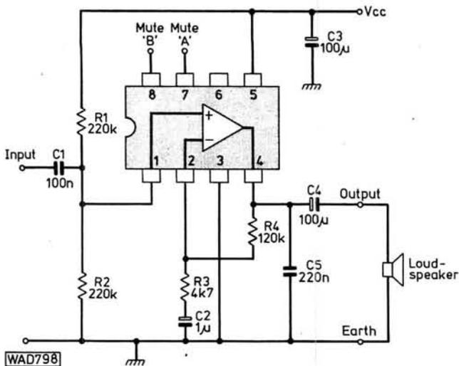
Fig. 4: A simple audio amplifier using the SL6310C
