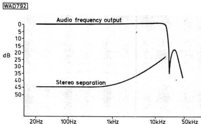
Graph showing audio frequency response and separation on stereo
