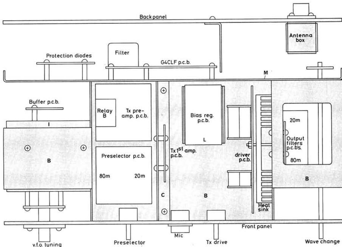
**Fig. 34 (above): Underside view of the PW Helford case showing how the various screens and p.c.b.s mount. Fig. 35 (below): Top view of the case**
