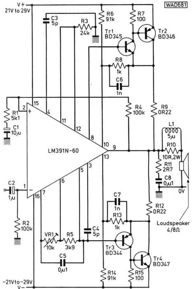
Fig. 17: A power amplifier using an integrated circuit power driver
