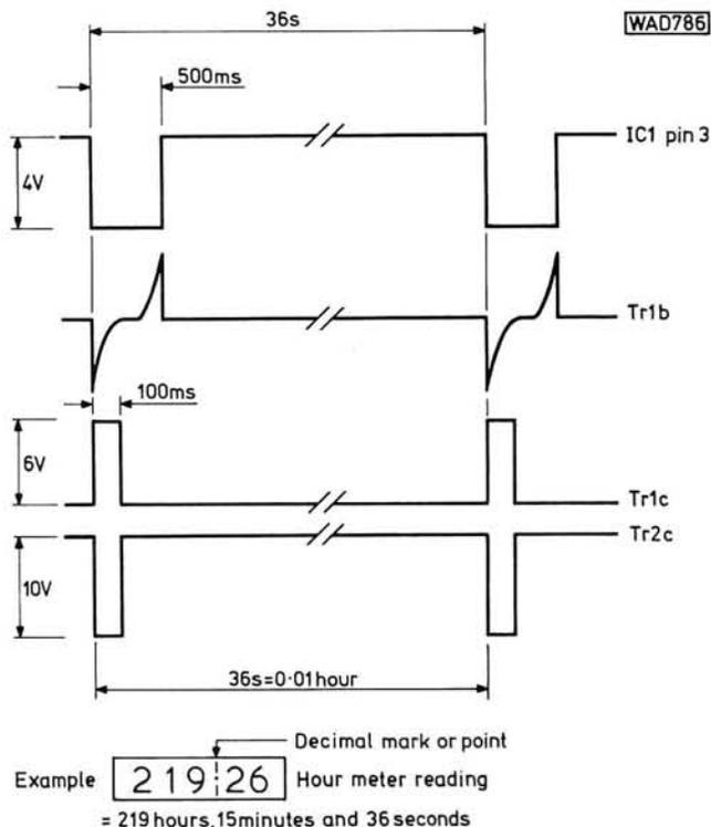
Fig. 1: The timing and duty cycle duration sequence for the counter
