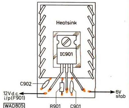
Fig. 28: Full size copper track pattern for the 6V stabiliser board. Fig. 29 (right): Component placement. Components are soldered directly to the copper
