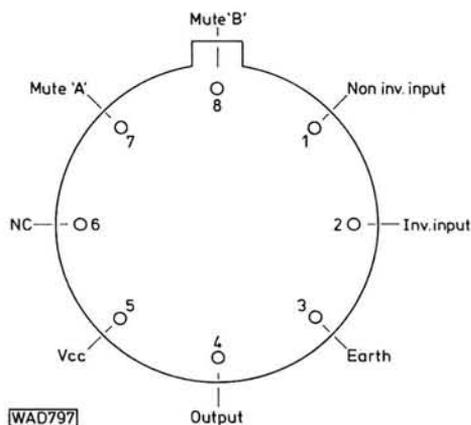
Fig. 3: Pin-outs for circular package
