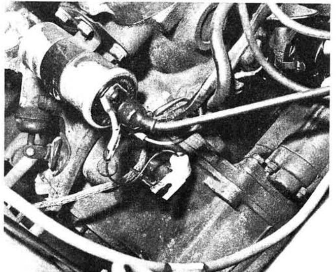
**Fig. 2: Temporary quick-fit capacitor connected between the h.t. coil + terminal and earth**
