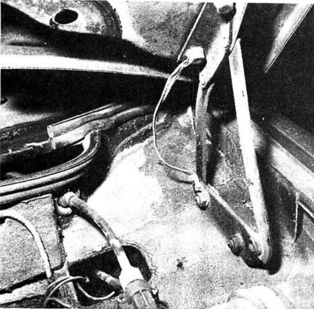
**Fig. 1: Additional bonnet bonding strap fitted to an Austin Maxi**
