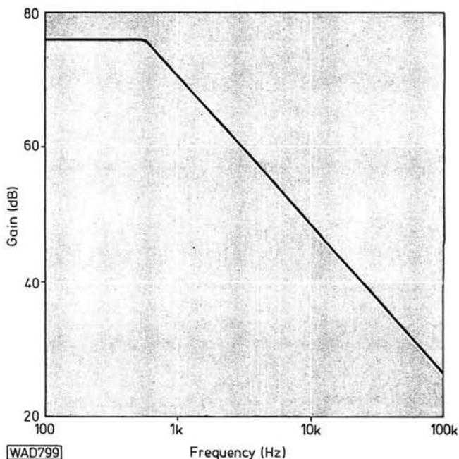
Fig. 5: Open-loop gain versus frequency
