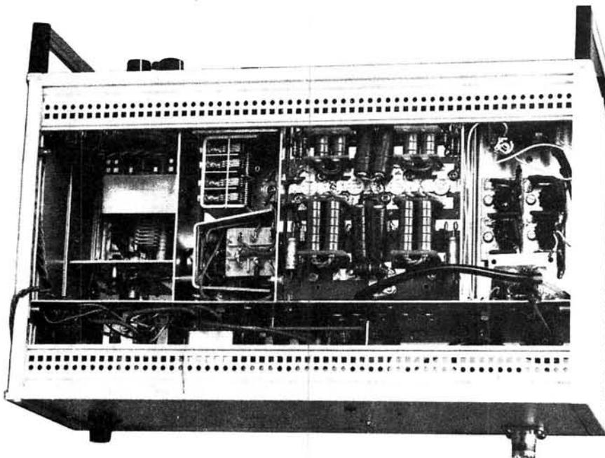
**View of the top of the *PW* Helford with the lid removed. The p.a. is central with the preselector capacitor and the v.f.o. to its left. The speaker is mounted on the lid with its magnet fitting into the space above the v.f.o. capacitor**
