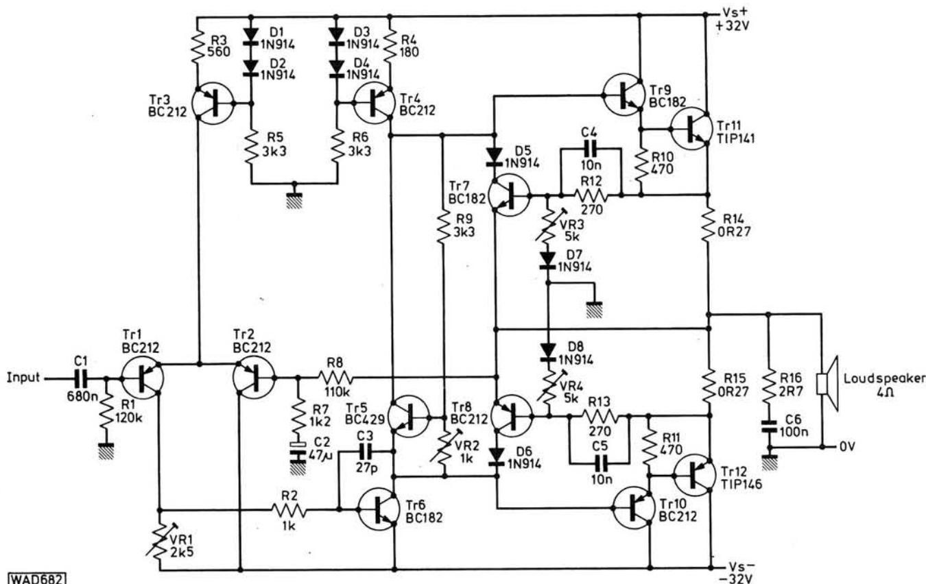
Fig. 18: A 75W amplifier circuit
