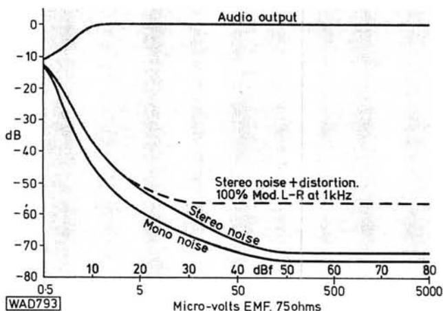
Graph showing audio output and signal-to-noise and signal-to-noise-plus-distortion on stereo for various input signal levels on 98MHz
