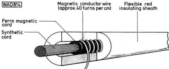
**Fig. 3: Cross-sectional view of Sparkrite ferro-inductive h.t. lead**
