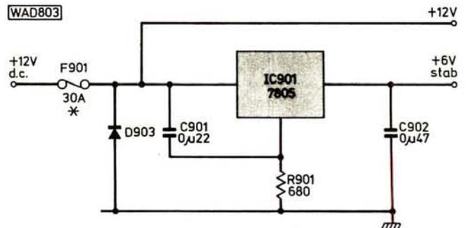
Fig. 27: The circuit diagram of the 6V stabiliser
