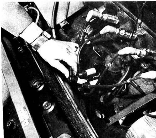
the cable passes from the electrically noisy area of the engine compartment, through the bulkhead screen, into the interior of the vehicle, it is good practice to fit a 3A in-line choke close to the coil terminal.
