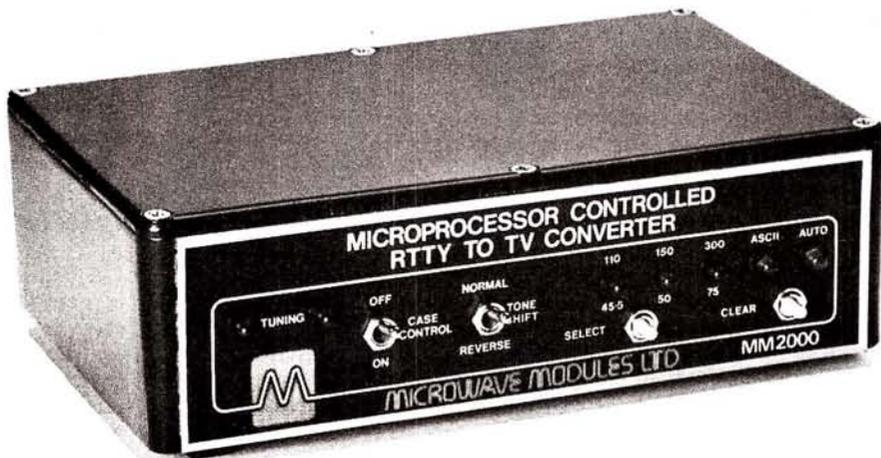
made by means of phono sockets. The power supply input of 12.5V, at approximately 1A, is by means of a DIN socket. Plugs are supplied with the unit for connection to these sockets.
