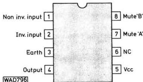
Fig. 2: Pin-outs for 8-pin d.i.l. package
