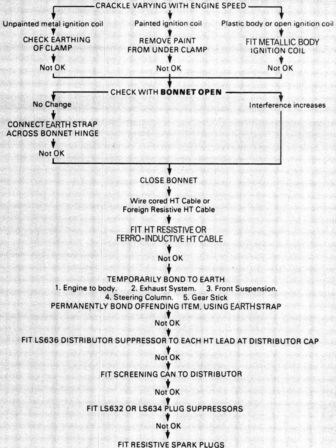
Fig. 5: Flow chart detailing the complete path of h.t. suppression
