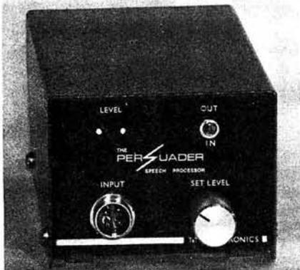
The input will accept signals over the range 0.5mV to 100mV and is suitable for most standard microphones. Once the "set level" control has been adjusted to show the correct level on the two l.e.d.s, the output will be automatically correct for the rig and microphone being used.
