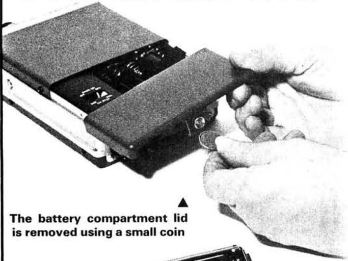
▲ The battery compartment lid is removed using a small coin
