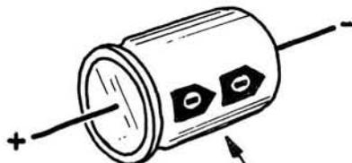
For double-ended capacitors, the can is always negative, regardless of any other markings or the colour of the bung.
