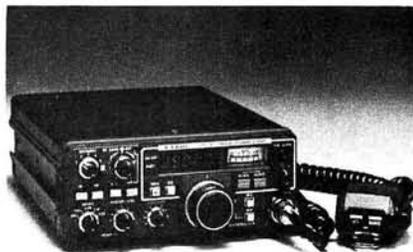
**Trio** have just announced that they will be introducing the TR-9500 70cm all mode (f.m., u.s.b., c.w. and l.s.b.) transceiver based on, and almost identical to, the very popular TR-9000 2m all mode transceiver.
