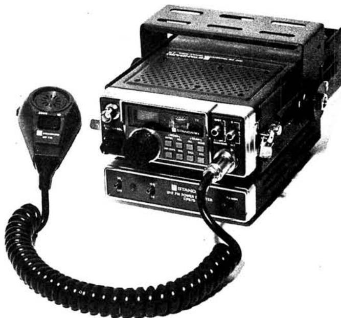
repeater and reverse repeater working. Unlike the C7800 this rig is equipped with this useful function which makes repeater operation much easier.
