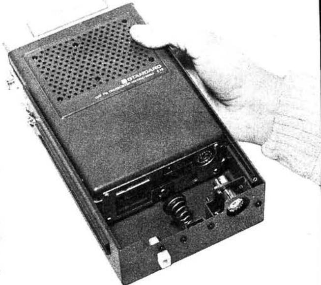
▲ The C78 slides into its special bracket, making all connections at the same time
