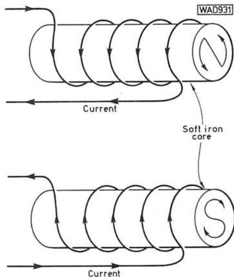
**Fig. 12: Field direction in a solenoid**
