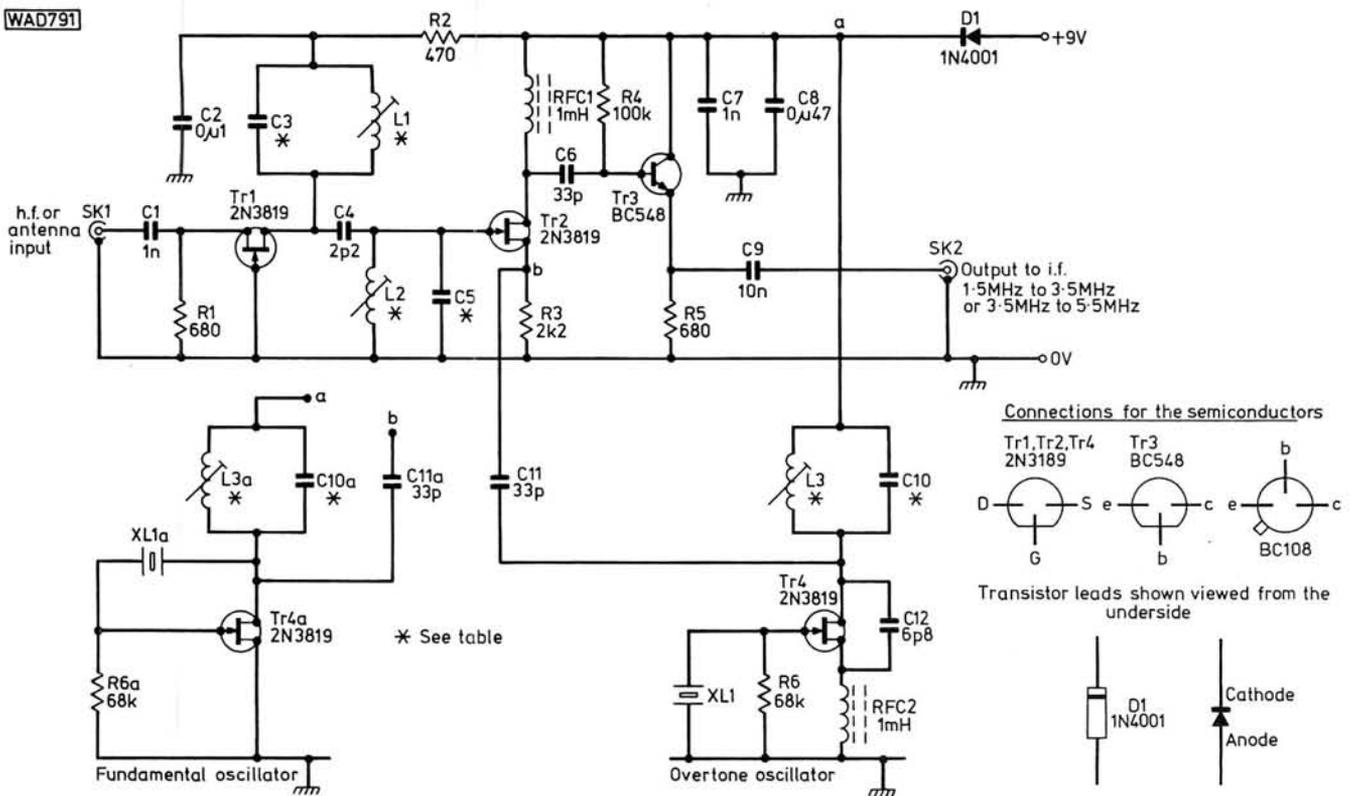
Fig. 2: Circuit diagram of the h.f. converter
