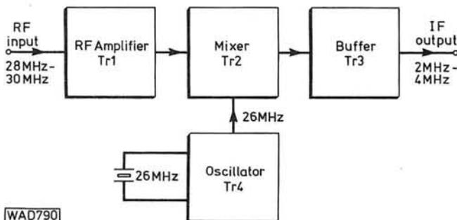
Fig. 1: Block diagram of the h.f. converter. Frequencies shown for 10m amateur reception
