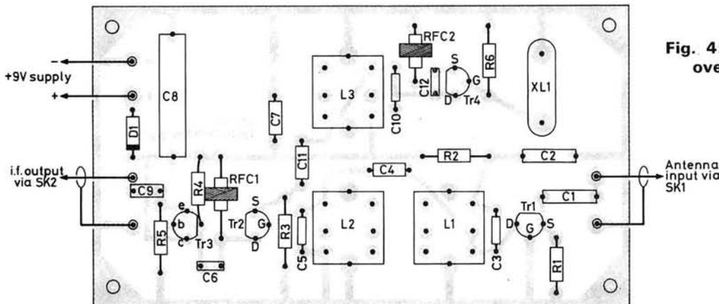
Fig. 4: Component overlay for overtone crystal oscillator
