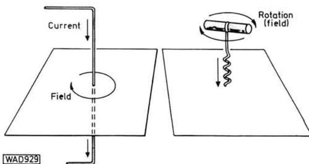
**Fig. 10: The direction of a magnetic field shown by the corkscrew rule**
