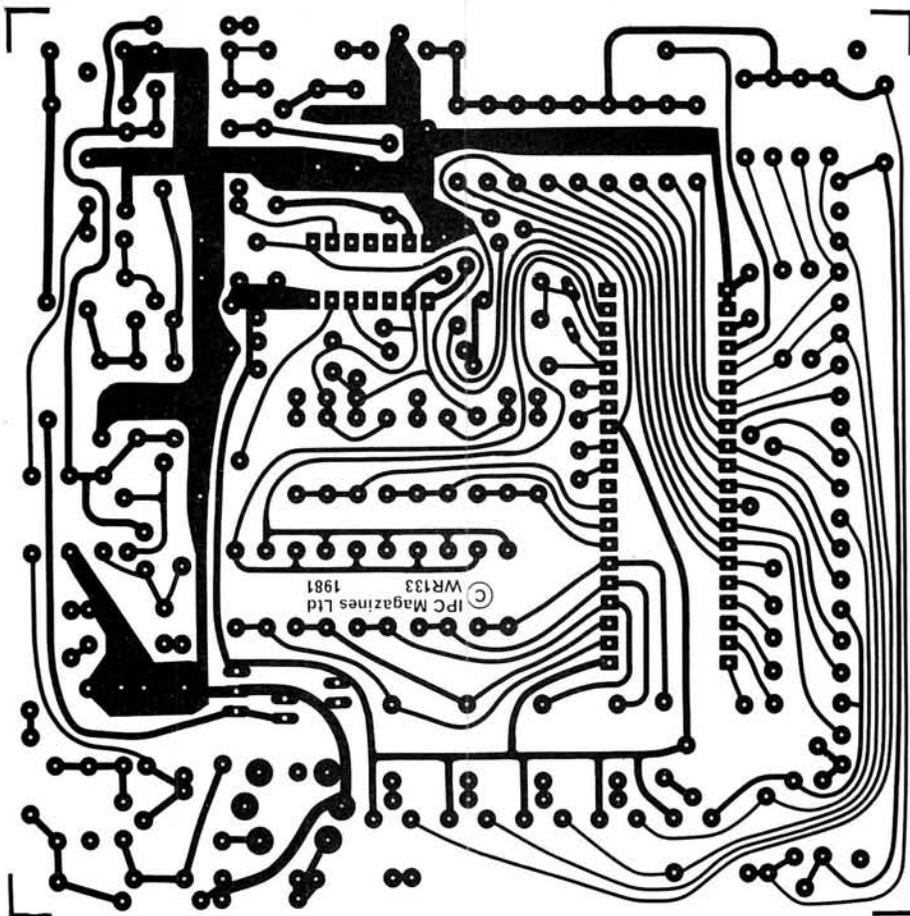
Fig. 6: Track pattern for the digital board, shown full size
