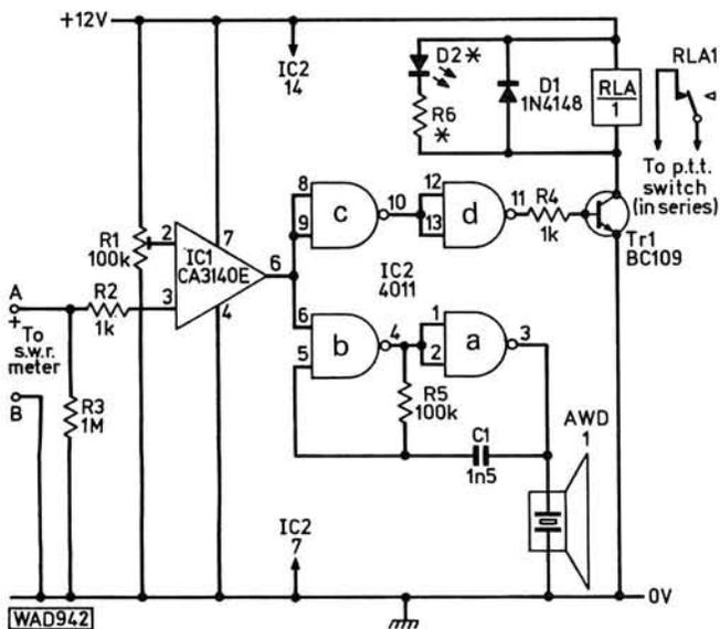
Fig. 1: The circuit diagram of the s.w.r. warning alarm
