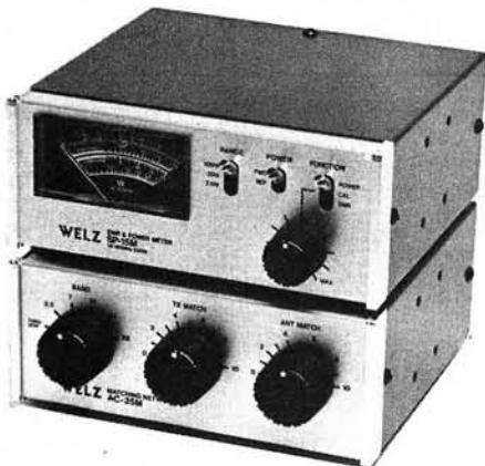
Moving up-market, we come to three s.w.r. and power meters intended for base-station use and with larger-scale meters. The SP-200 covers 1.8-160MHz at powers up to 1kW, and the SP-400 130-500MHz at 150W. The SP-300 (also shown here) is really
