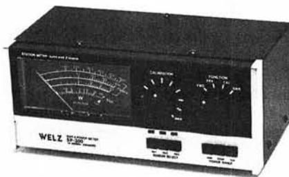
three instruments in one, with separate sensors and input/output sockets for ranges of 1.8-160MHz at up to 1kW, 1.8-200MHz at up to 200W, and 130-500W at up to 150W (all carrier powers).
