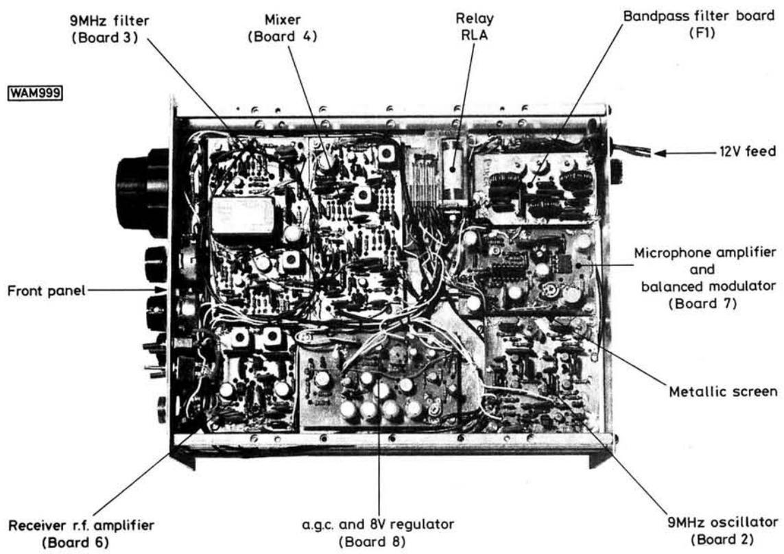
**Fig. 42: General layout of the transceiver under side**
