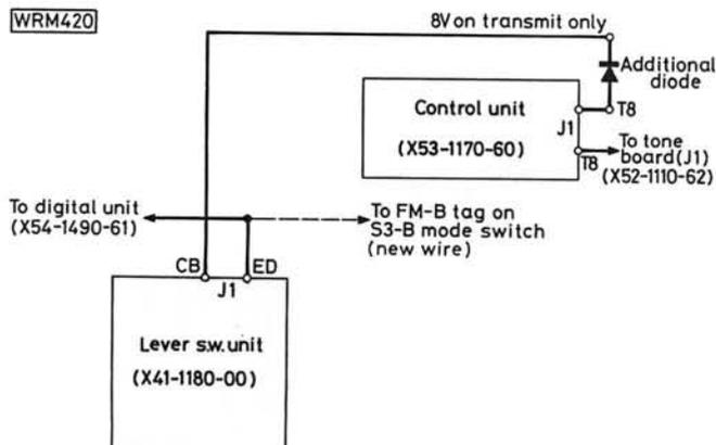
There are no external changes to the set as the mode switch (S3) is used to initiate the reverse repeater function by using the FM-B position to activate the correct shifts on both 2m and 70cm, -600kHz and +1.6MHz respectively. The FM-A position provides reverse repeater operation when the "SHIFT" button is depressed. The alternative shifts that were available are disabled by the mod to the mode switch.
