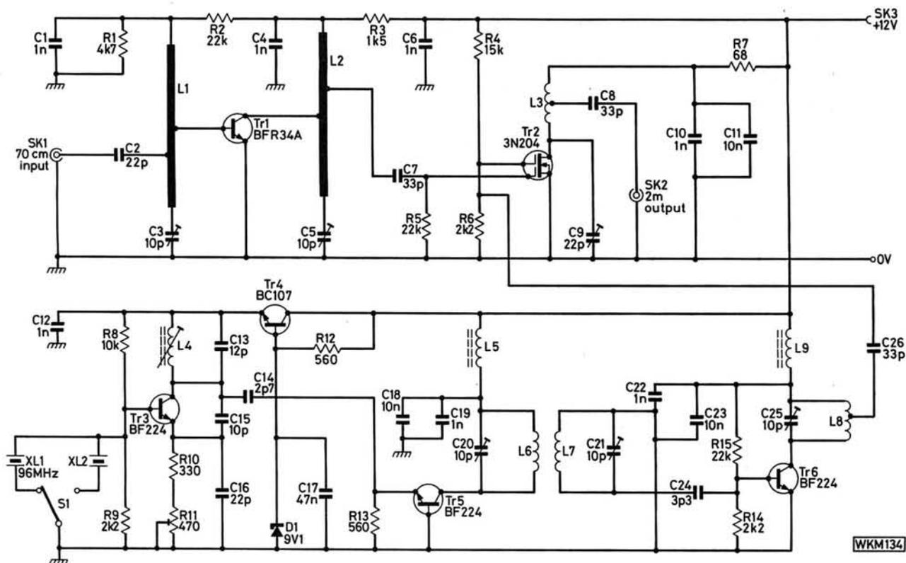
Fig. 1: Circuit diagram of the converter
