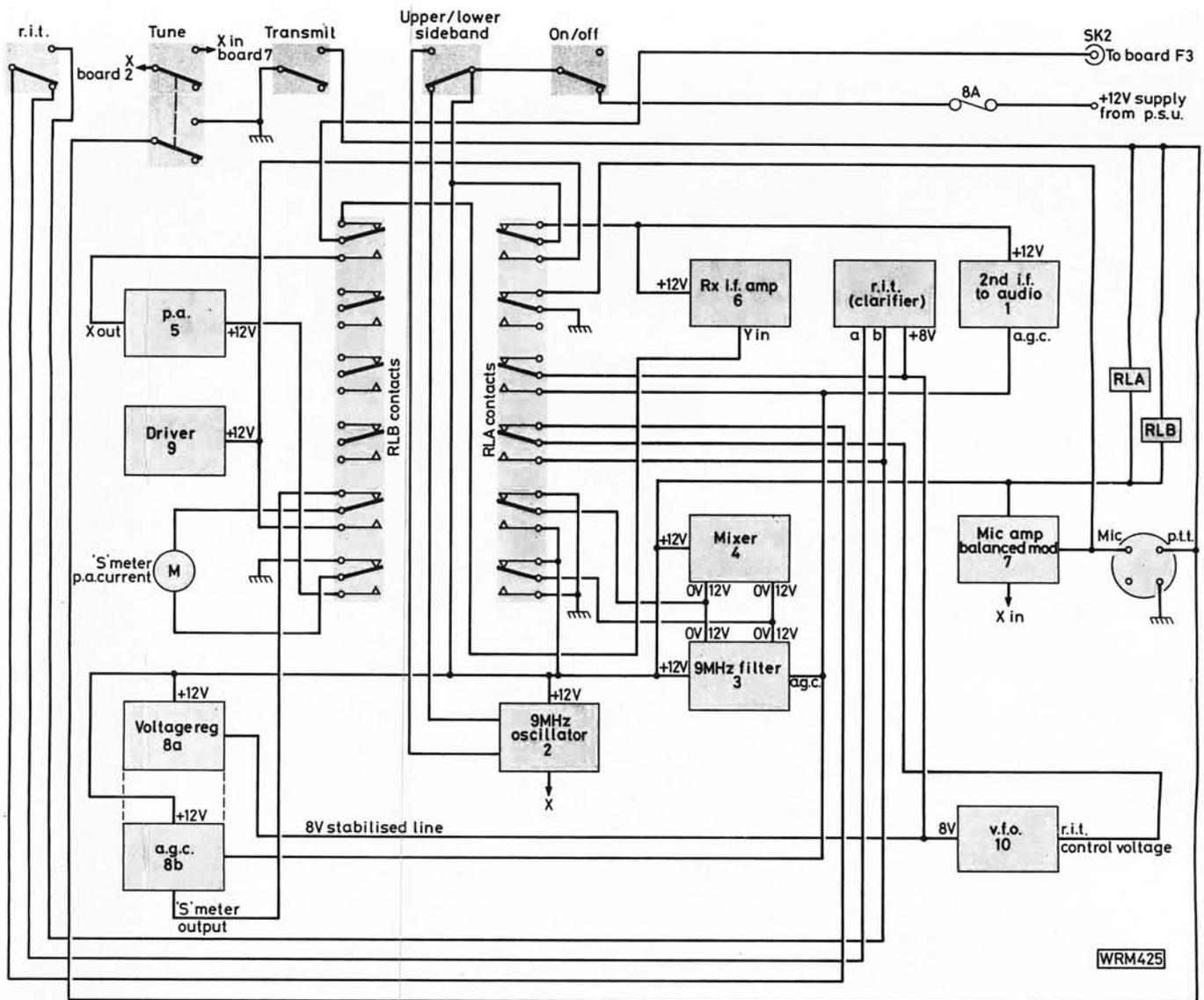
**Fig. 40: Relay and front panel switching diagram**
