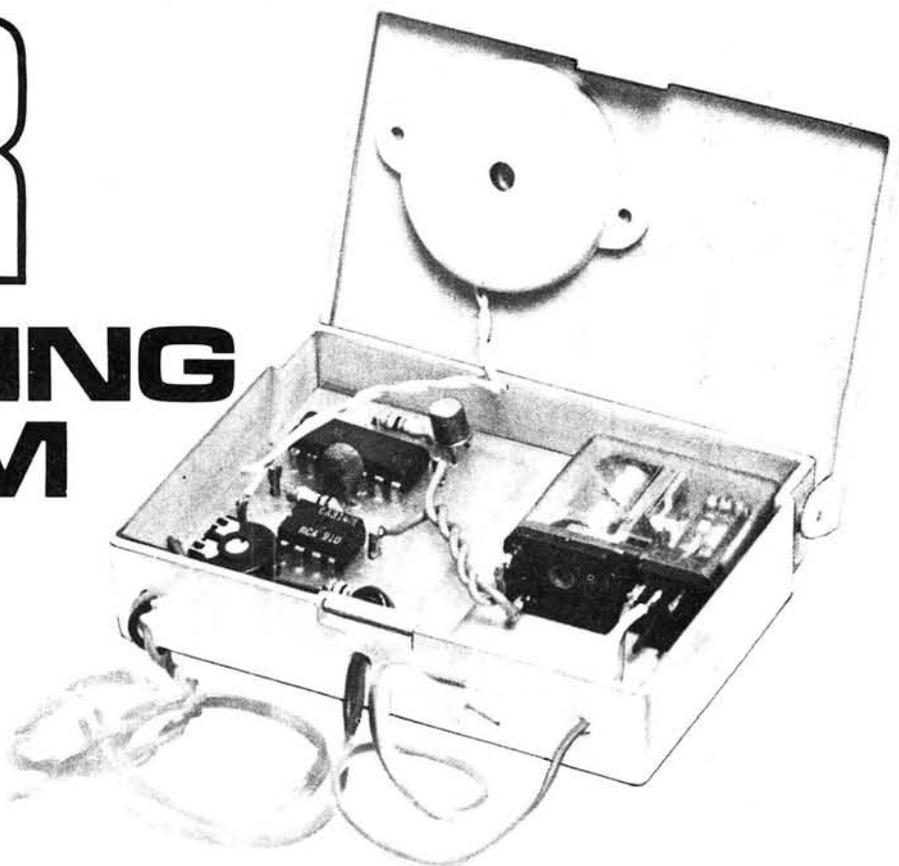
One of the main worries of a radio operator is of transmitting either without an antenna or with a faulty antenna connection, resulting in a high s.w.r. and, often, a useless p.a. stage. This design provides an alarm in such circumstances, with the option of automatically switching the transmitter off.
