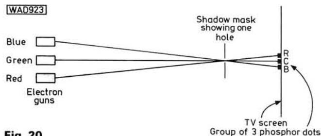
which glows blue when energised by an electron beam, whilst the other two glow green and red respectively.
