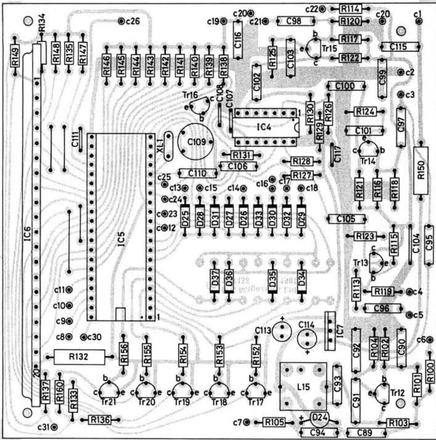
Fig. 7: Component layout for the digital board. See text regarding R151 and R106 to R112
