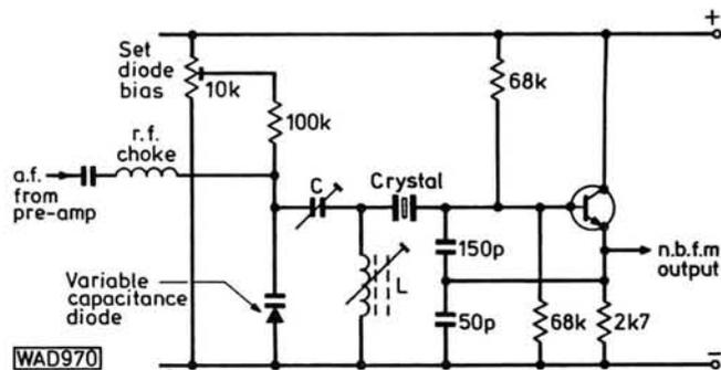
Fig. 58: A typical n.b.f.m. oscillator circuit
