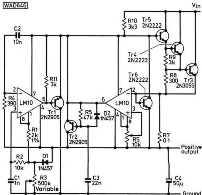
**Fig. 8: A laboratory power supply providing 0V to 50V at outputs of up to 1A**
