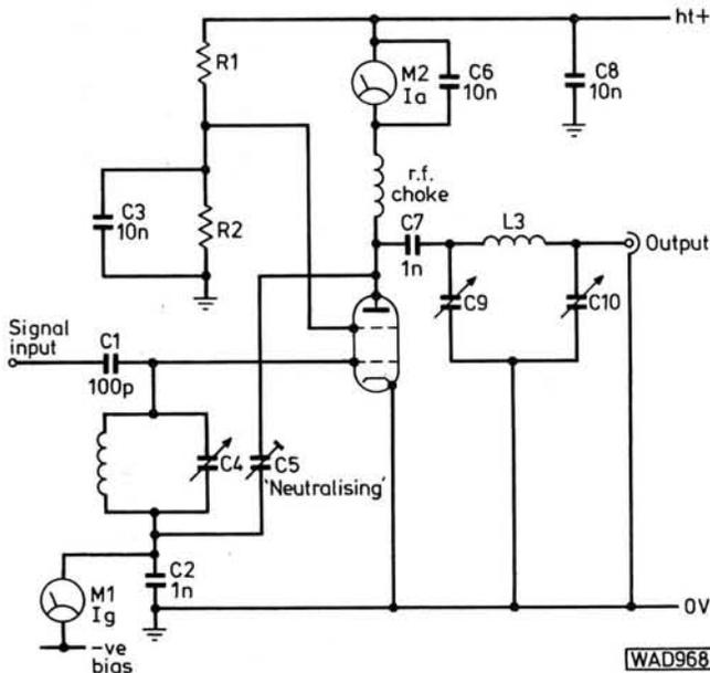
Fig. 56(a): Linear power amplifier
