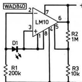
Fig. 3: A light detector using the LM10
