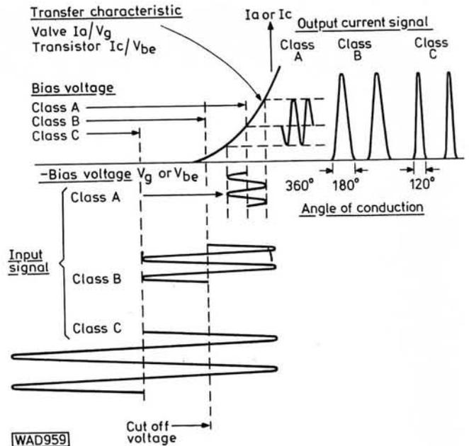
Fig. 48: Operating conditions for Class A, B and C
