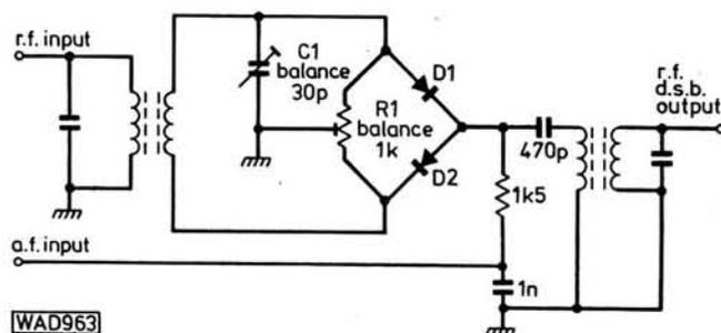
Fig. 54: Diode bridge modulator
