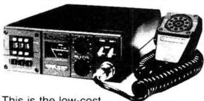
This is the low-cost, easy to use economy model. Full bank – 80 channels at 25KHz spacing by easy to use press button switches. 12 $\frac{1}{2}$ KHz spacing if required, and the same reliable performance as the famous IC240. Price £169.
