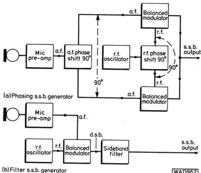
Fig. 53: Two methods of generation of an s.s.b. signal
