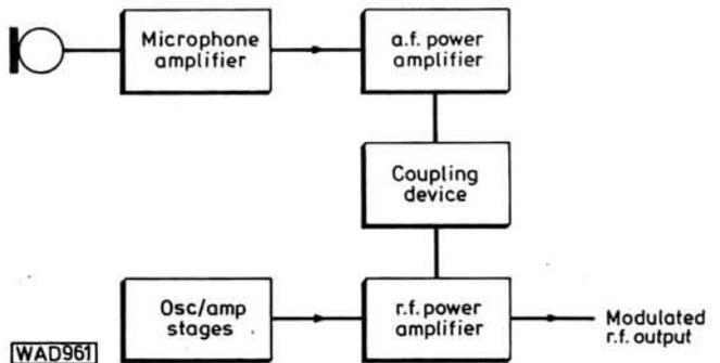
**Fig. 52(a): Block diagram of a.m. (A3E) transmitter**
