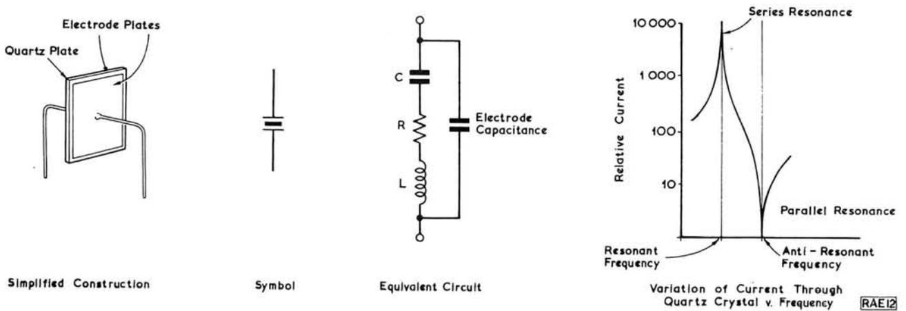
**Fig. 61: Features of a quartz crystal**
