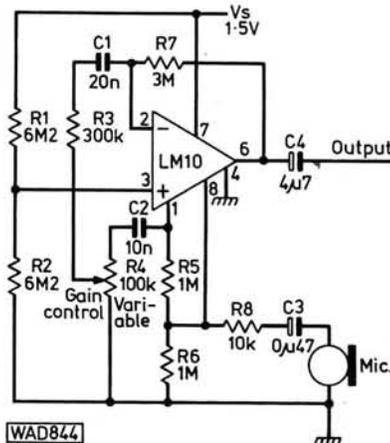
**Fig. 7: A microphone amplifier with a gain of 60dB using one i.c.**
