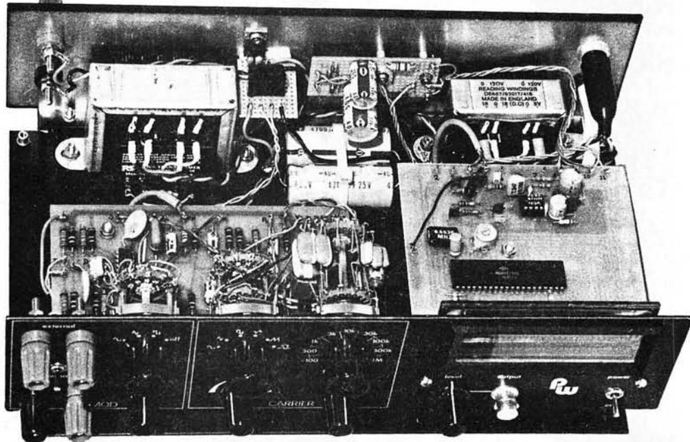
**Fig. 6: Frequency counter power supply board**
