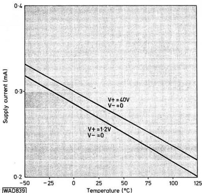
Fig. 2: Variation of supply current with temperature
