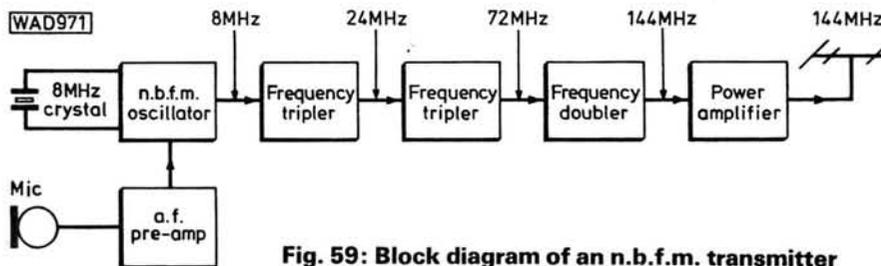
Fig. 59: Block diagram of an n.b.f.m. transmitter
