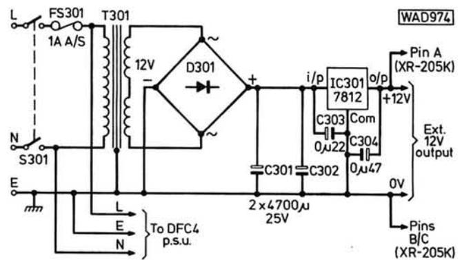
Fig. 3: Waveform generator power supply circuit
