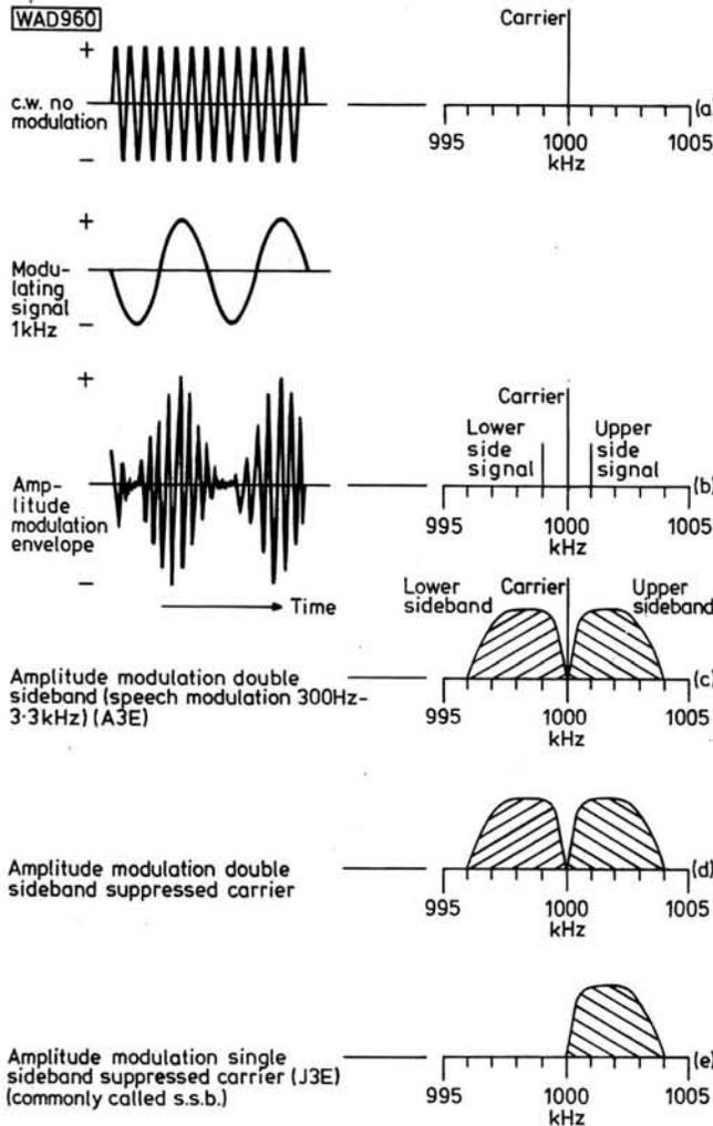
**Fig. 51: Examples of a.m. envelopes showing sidebands**
