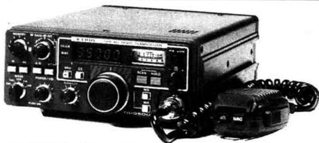
The TR9500, a 70cm multimode mobile giving SSB, FM and CW operation in a compact rig based on the phenomenally successful 2 metre 9000. Combining the convenience of FM with the "DX ability" of SSB on the 70cm band this is the rig all discerning VHF and UHF amateurs have been waiting for.
