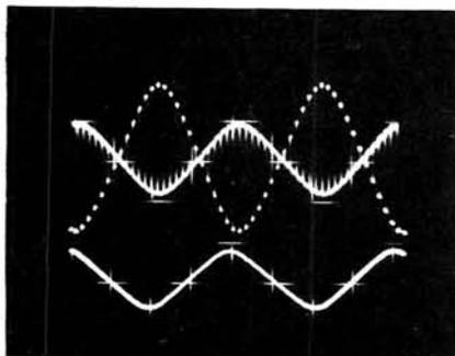
**One of the weird waveforms you can produce. Suppressed-carrier mod of pulses by an a.f. sinewave. Note the polarity reversal of the pulses on each half-cycle**
