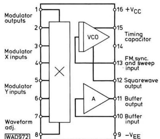
Fig. 1: XR-205 system block diagram and pin-outs
