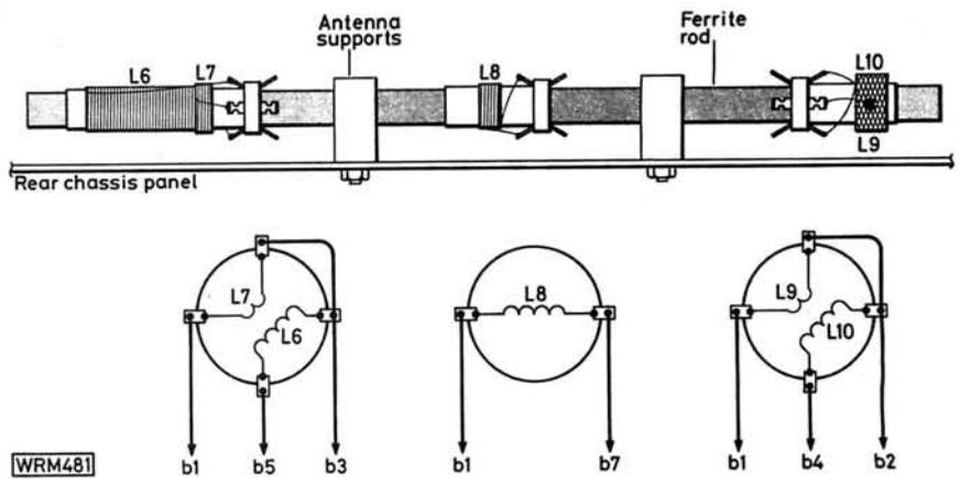
**Fig. 15: Connections to the TV r.f. unit**
