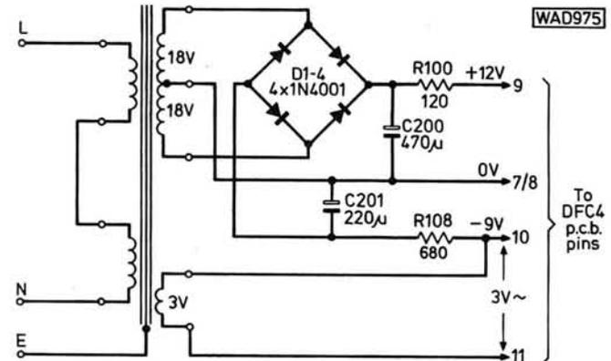
Fig. 4: Power supply for the DFC4 digital frequency counter
