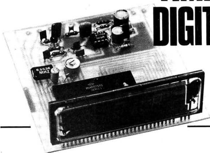
A digital readout adds a touch of class to a receiver as well as giving a more accurate and easily read indication of frequency. Our special offer this month is a complete kit of parts to enable you to add a 3½ digit readout with a large bright phosphorescent display to your a.m. or f.m. receiver.
