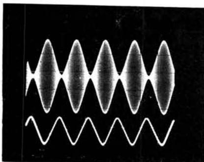
**A 90% modulated a.m. waveform (top). Note how the envelope follows the modulating waveform shown on the bottom trace**
