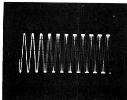
**A frequency-modulated carrier. The oscilloscope trace is triggered, and therefore steady at the left-hand end**
