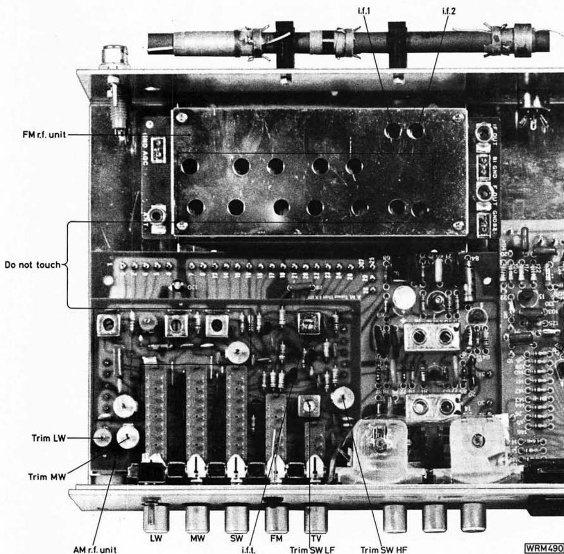
**Fig. 17: The f.m. and a.m. r.f. units with their respective tuning adjustments marked**
