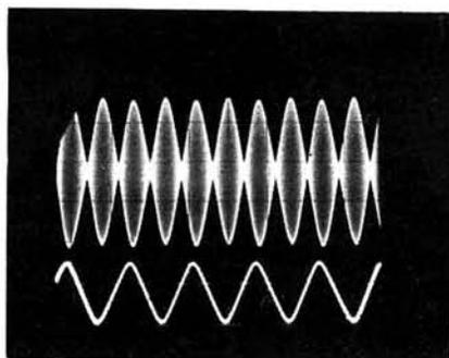
**A d.s.b. suppressed carrier a.m. waveform (top). Note the two envelope peaks per cycle of the modulating waveform**
