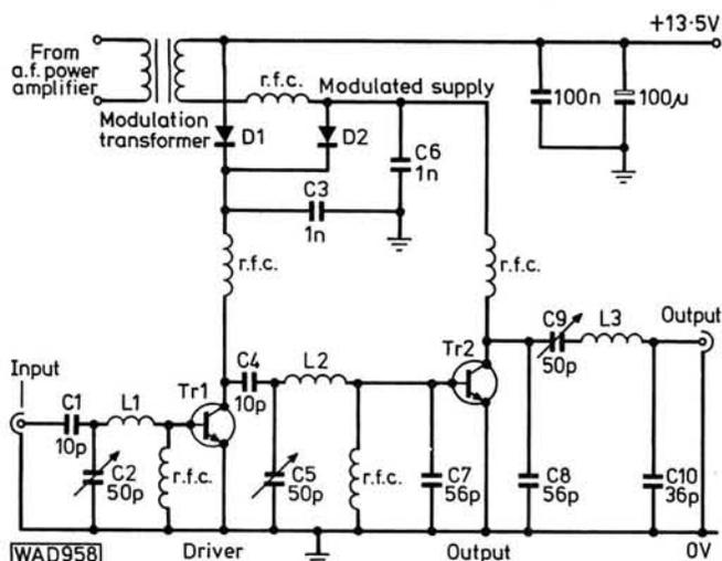
Fig. 52(b): Output stage of 144MHz a.m. transmitter
