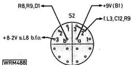
**Fig. 2: Connections to ON/OFF switch S2. Position 1 OFF, 2 CONVERTER ON and 3 CONVERTER AND BFO ON**
