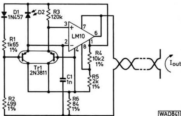
Fig. 4: A logarithmic light sensor circuit. This has a response similar to the human eye as far as variations in intensity are concerned
