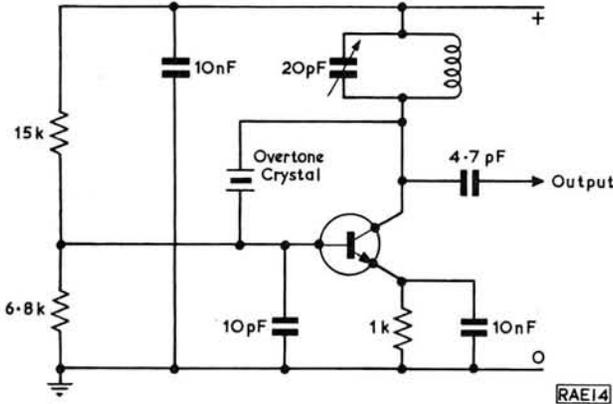
**Fig. 62: An overtone crystal oscillator circuit**
