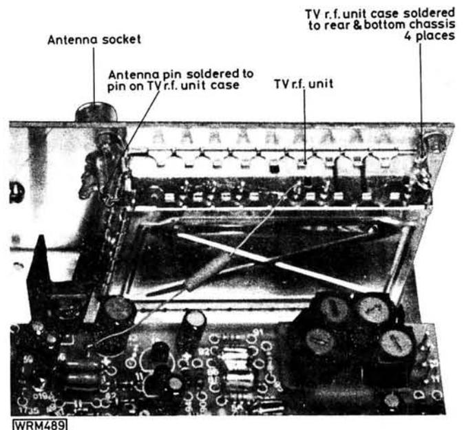
Fig. 16: The mounting of the TV r.f. unit
