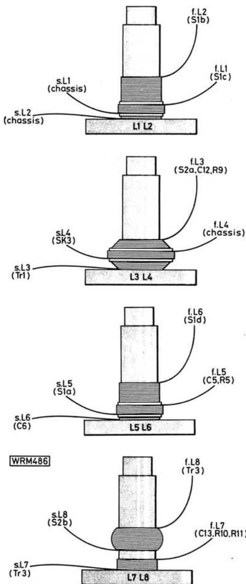
**S = start of winding, F = finish of winding. All turns are wound in the same direction**
