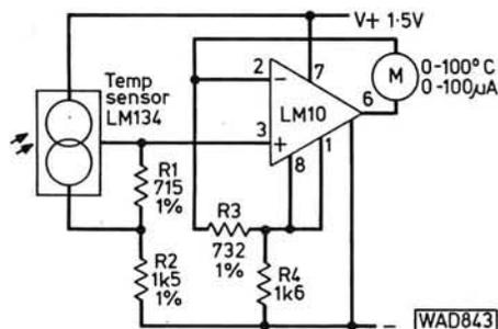
**Fig. 6: An electric thermometer**
