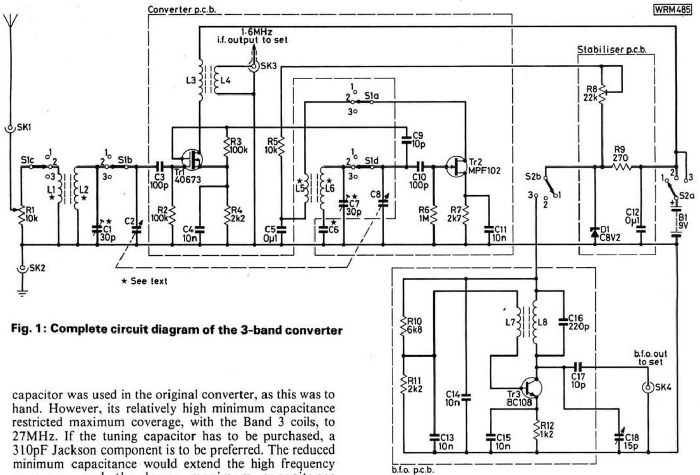
Fig. 1: Complete circuit diagram of the 3-band converter
