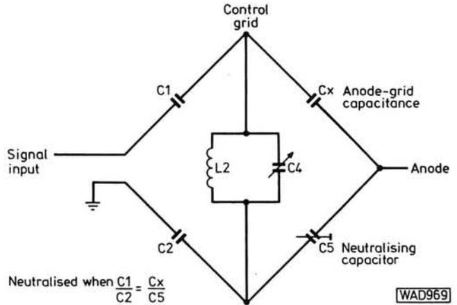
Fig. 56(b): Equivalent circuit of Fig. 56(a)
