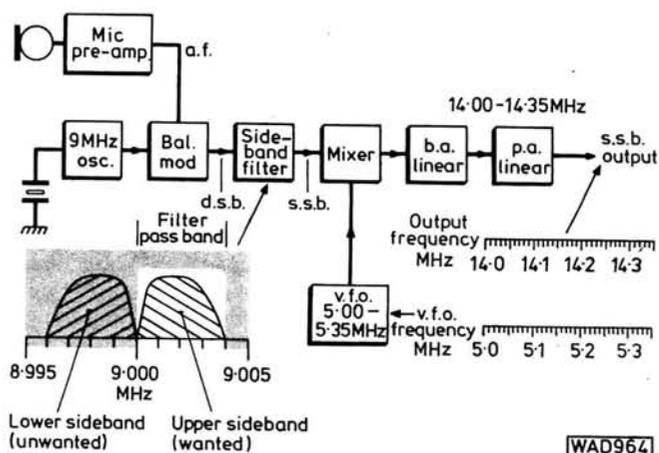
Fig. 55: Block diagram of a single band s.s.b. transmitter
