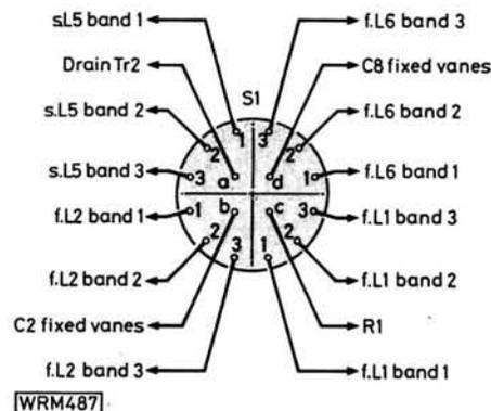
**Fig. 3: Connections to band selector switch**
