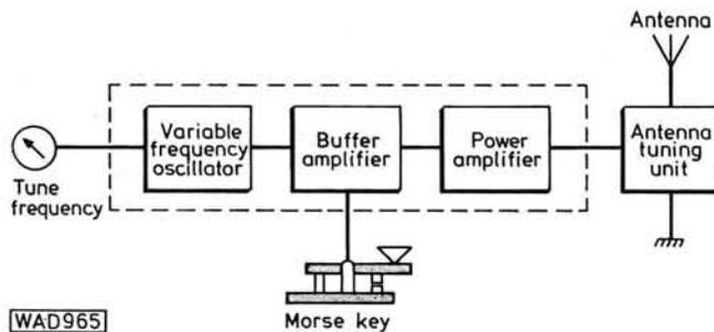
Fig. 47: Block diagram of a c.w. transmitter
