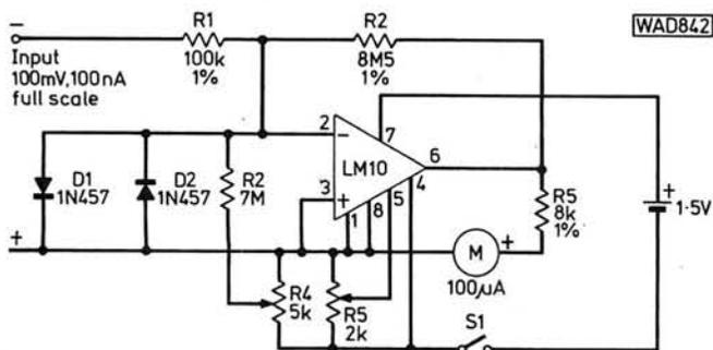
**Fig. 5: A 10mV, 100nA meter circuit using the LM10**
