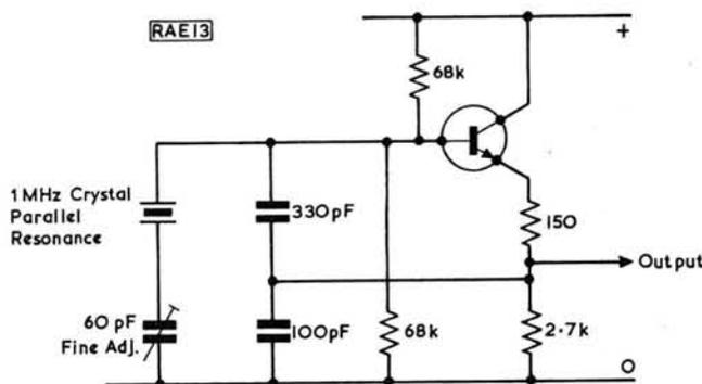
Fig. 60: A basic crystal oscillator circuit
