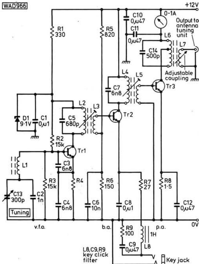
Fig. 49: The circuit diagram of the c.w. transmitter of Fig. 47
