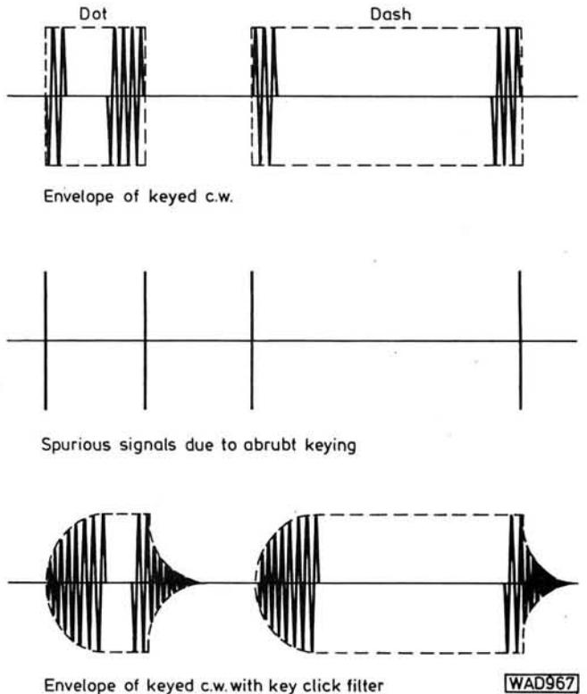
Fig. 50: Signal envelopes with and without key click filter
