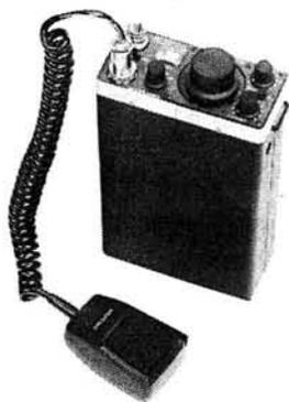
For those of you who enthuse over portable SSB operation on the hills and mountains of the UK, or wish to chat to the local lads whilst seated by your fireside, then the Mizuho SB2X 2 metre SSB portable is the rig for you. One watt output on the SSB frequencies 144.000 to 144.600 and the ability to listen to the beacon frequencies from 144.800 to 145.000 (also transmit).
