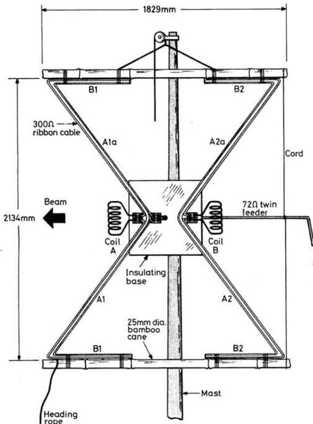
Fig. 1: A1a = A1 = A2a = A2 = 1.37m, B1 = 800mm, B2 = 851mm
