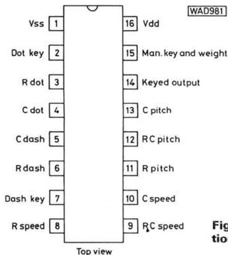
**Fig. 6: Pin functions for the Curtis 8044**
