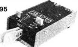
Experienced radio operators, both professional and amateur, know the advantages of an electronic key. Fatigue-free operation and smooth and consistent morse code. The EK121 will work with all modern amateur radio transceivers and operates from either internal batteries or external 6v DC. Speed is 4-30 wpm. A nice key at an incredible price.
