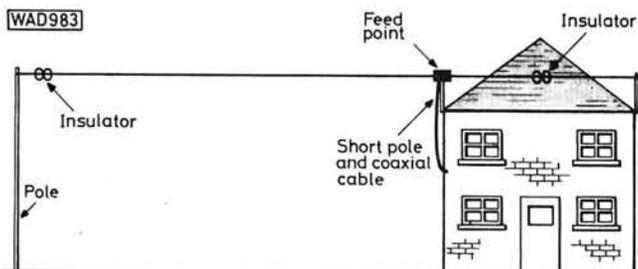
**Fig. 3: The author's final layout for the DX dipole**
