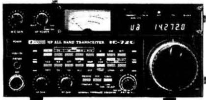
This is the best money can buy. AM, SSB, RTTY and CW. Built-in fan, speech processor, two VFO's and APC. Tuning rates down to 10Hz and memories. General coverage receiver from 100KHz to 30MHz (transmit too if you have a licence!) Run from 13vDC or use PS15 mains PSU.
