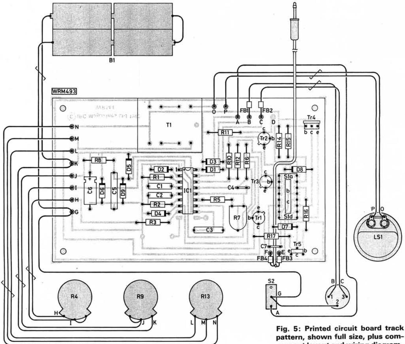
Fig. 5: Printed circuit board track pattern, shown full size, plus component layout and wiring diagram
