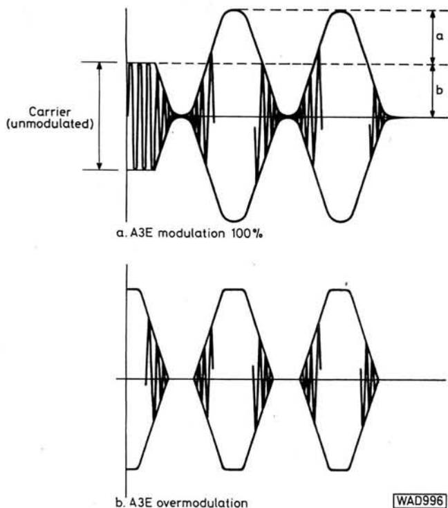
**Fig. 68: Modulation patterns for an A3E signal. Note that in the overmodulated condition flattening of the peaks will usually occur**
