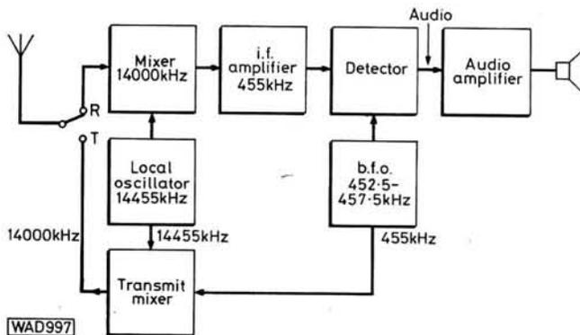
**Fig. 1: Block diagram of a basic superheterodyne receiver with additional outputs from the b.f.o. and local oscillator taken to a transmit mixer stage to provide a signal of the same frequency as the one being received. Thus a basic c.w. transceiver is formed**
