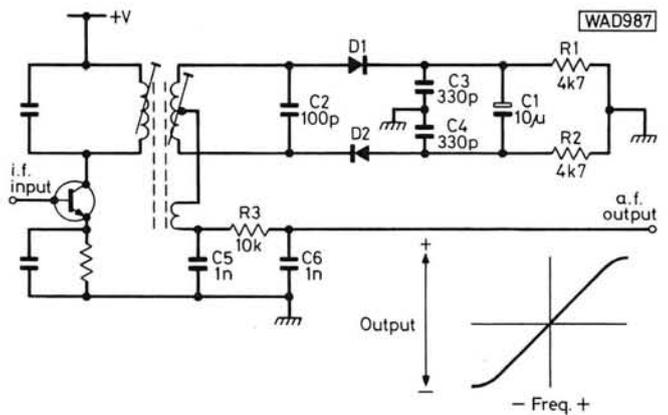
Fig. 78: Ratio detector f.m. demodulator
