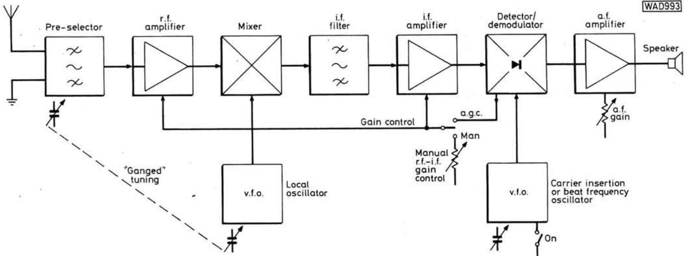
**Fig. 71: Block diagram of a basic superheterodyne**
