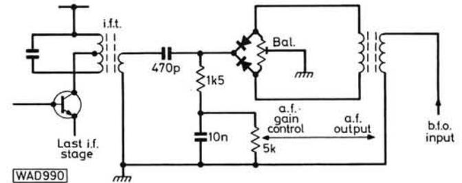
Fig. 77: The balanced demodulator
