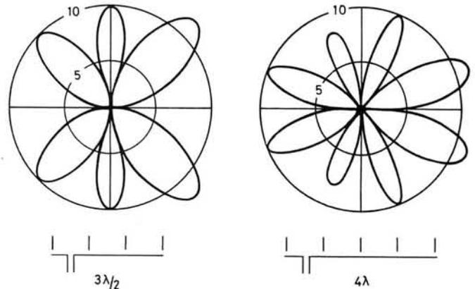
Fig. 2: Radiation patterns of offset fed dipoles
