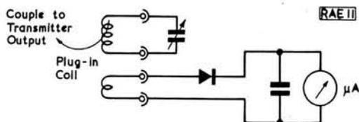
Fig. 63: An absorption wavemeter circuit
