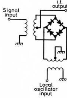
Fig. 73(b):  $\blacktriangle$  Diode ring mixer
