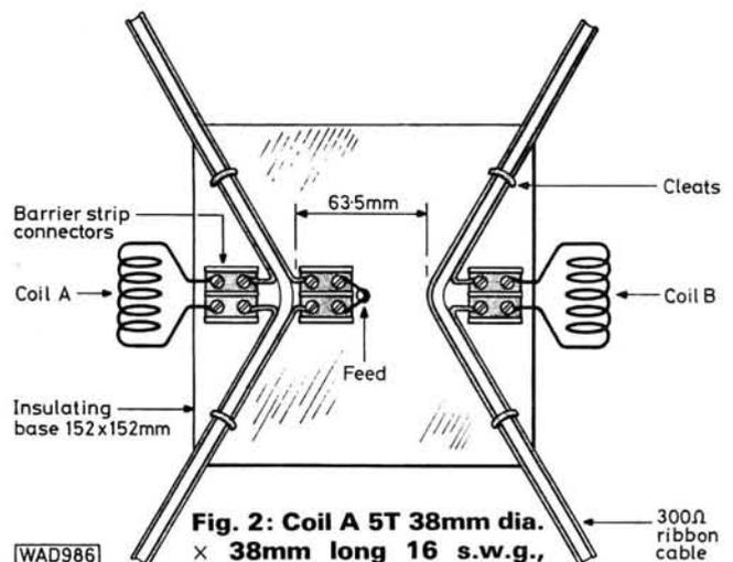
Fig. 2: Coil A 5T 38mm dia. x 38mm long 16 s.w.g., Coil B 7T 32mm dia. x 45mm long 16 s.w.g.
