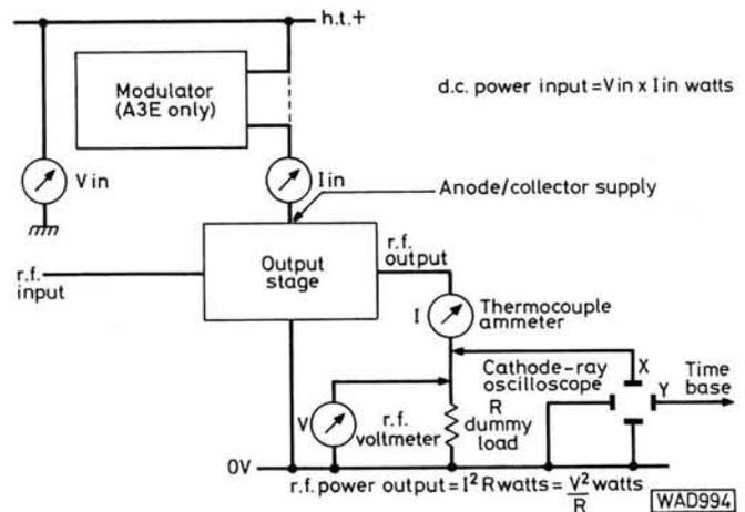
**Fig. 67: Transmitter power measurement**
