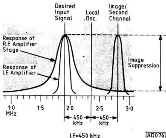
**Fig. 72: Suppression of the second channel or image response**
