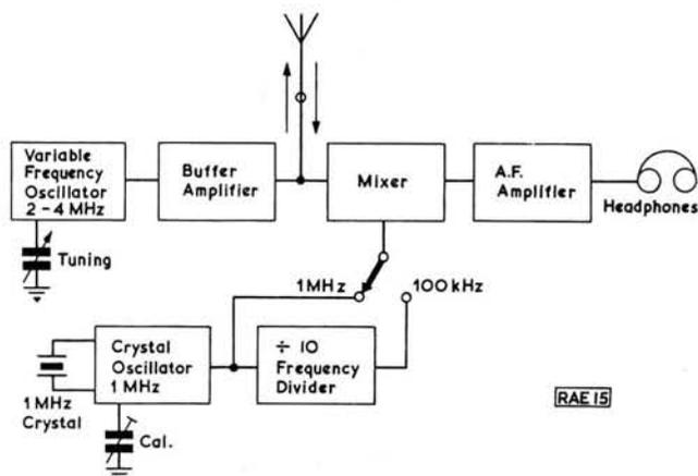
Fig. 64: Block diagram of a heterodyne frequency meter
