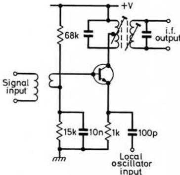
Fig. 73(a):  $\blacktriangle$  Transistor mixer stage
