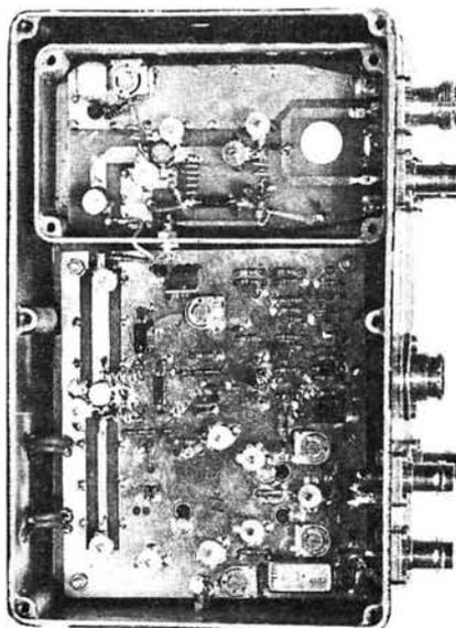
The linear final p.a. stage features a rugged, well proven, silicon transistor to obtain a continuously rated r.f. output of 1.3W. Printed stripline techniques are used with antenna changeover switching accomplished by a *pin* diode  $\lambda/4$  relay, which has an insertion loss of under 0.5dB.
