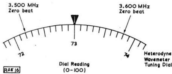
**Fig. 65: Interpolating between crystal calibrator points**
