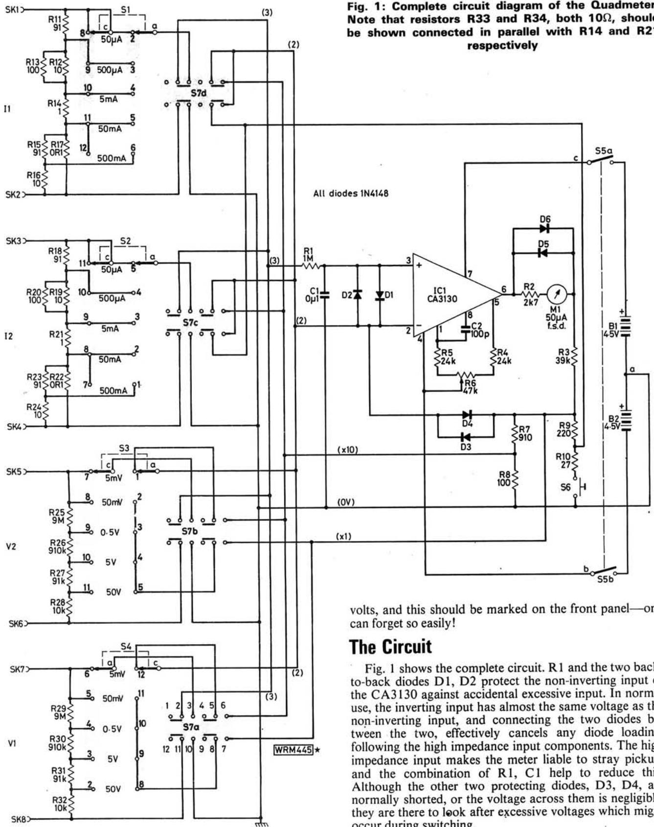
**Fig. 1: Complete circuit diagram of the Quadmeter. Note that resistors R33 and R34, both 10Ω, should be shown connected in parallel with R14 and R21 respectively**
