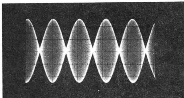
Fig. 2: Two tones of equal amplitude on s.s.b.
