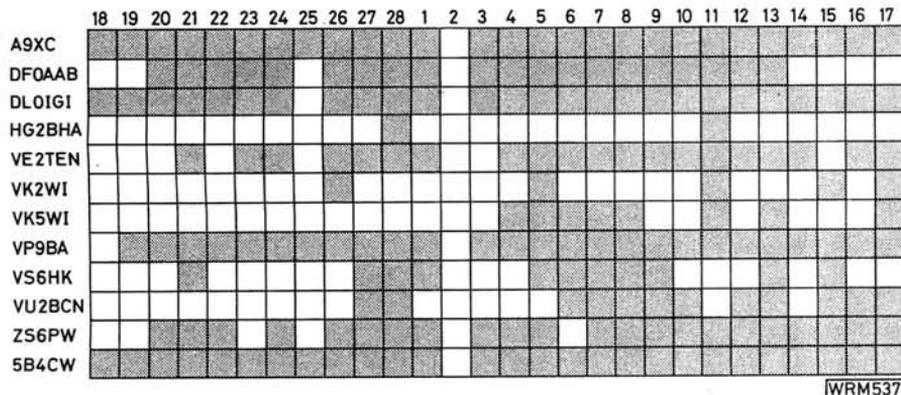
Fig. 3: 28MHz beacon reception. Note the blackout on March 2
