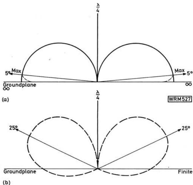
**Fig. 3: (a) Vertical angle radiation pattern of a quarter-wave vertical antenna over a perfectly conducting ground-plane of infinite dimension. (b) When the ground-plane is of some infinite dimension, e.g. one wavelength and consists of a number of radials, the vertical angle of maximum radiation is tilted to about 25 degrees**
