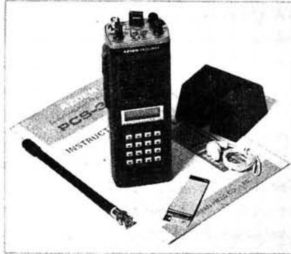
i.f.s. Receiver sensitivity is quoted as less than 0.2 $\mu$ V for 12dB SINAD over the complete bandwidth, with an audio output level of 200mW from the combined built-in speaker microphone.
