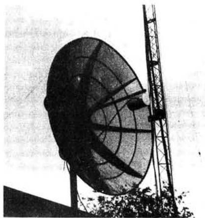
**Fig. 6: 2.5m dish for 1296MHz**
