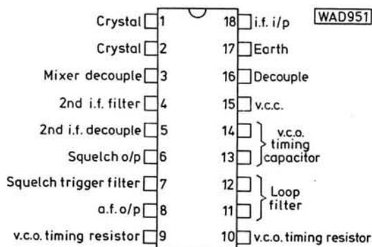
Fig. 2: Connections of the SL6600C
