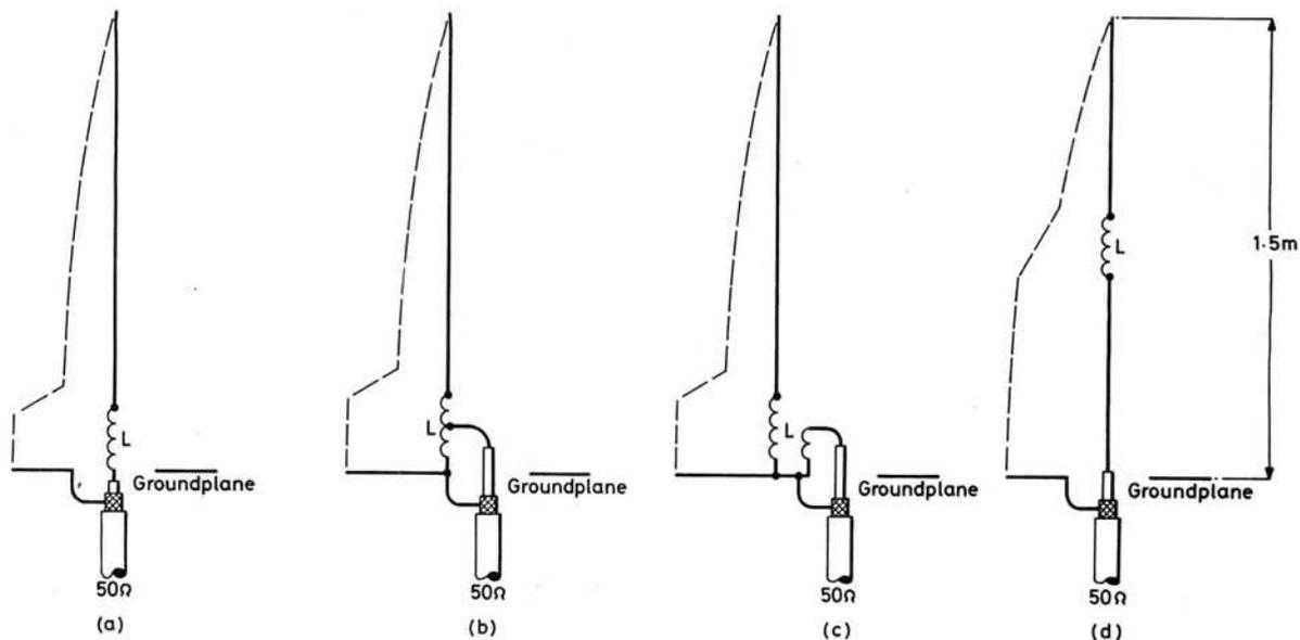
**Fig. 1: (a) Series-fed antenna with inductive loading at the base. (b) Shunt-fed by tapping into the loading coil at the base. (c) Link coupled shunt-fed base coil. (d) Centre loaded series-fed (see text). N.B. only (a), (b) and (c) meet the Home Office requirements for CB antennas**
