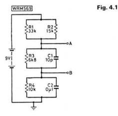
No. 1: You were asked to calculate the potentials at "A" and "B". As the capacitors do not affect the steady d.c. conditions, we ignore them. Resistor R1 in parallel with R2 becomes
