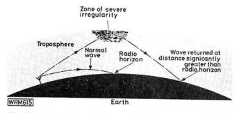
Fig. 4: One mode of enhanced-distance tropospheric propagation
