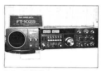
The Yaesu FT-102S (the low-power version) plus the SP-102 loudspeaker with switchable a.f. filters
