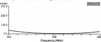
Fig. 4: VSWR—bandwidth readout from a Ring-Base antenna tuned for the 144MHz amateur band
