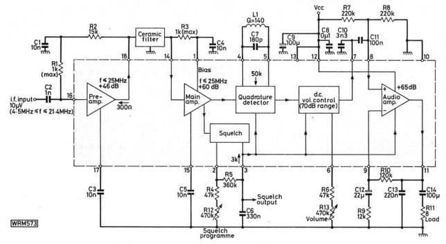
Fig. 3: Basic circuit and internal blocks for the **SL6640C**
