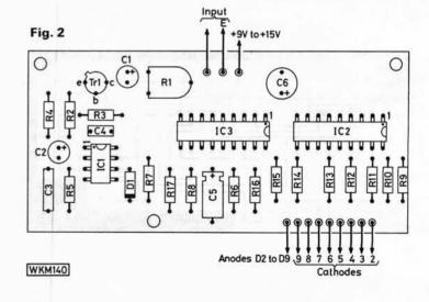
properly to transients. The decay time is much longer, since the only discharge path for C5 is through R6 and the high input impedance of the display circuitry. The reason for having a relatively long decay time is that once the unit has responded to a transient, the display reading is held long enough to be clearly visible to the user.
