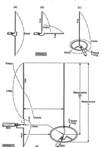
Fig. 1: Evolution of the Ring-Base Antenna
