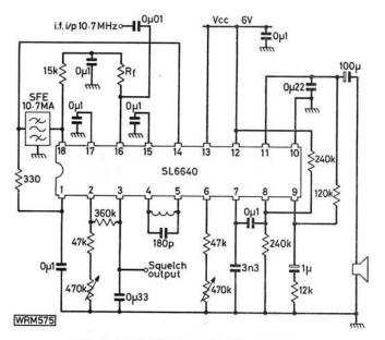
Fig. 5: A 10-7MHz SL6640C circuit
