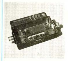
The a.t.u. should be installed as close as possible to the base of the antenna and connected via an s.w.r. meter to the CB rig. As the circuit functions equally well in both directions, the unit may be connected either way round.
