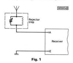
The rejector, which is placed between the antenna lead-in and the receiver (Fig. 1) operates best when used with a receiver with a low input impedance, which is pretty well standard with communications receivers. The impedance of the rejector is high at resonance and consequently its ratio to the receiver's impedance is also high so most of the energy from the unwanted station is dissipated in the trap.
