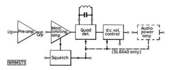
Fig. 1: Block diagram of the SL6640C and the SL6650C, the dashed components being incorporated in the SL6640C only
