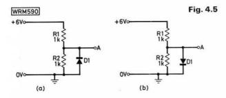
Consider, then, the examples in Fig. 4.5. In part (a), the diode is reverse biased so the potential at "A" will be +3V, just as if the diode was not in circuit. In Fig. 4.5(b), however, the diode is forward biased and since its opencircuit voltage would be 3V it will conduct, with 0.6V across it. Thus the potential at "A" will be +0.6V.
