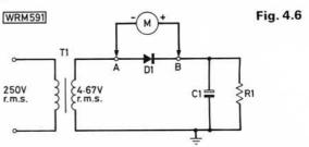
Using the meter on the d.c. volts range across the diode we shall read the average p.d. across it. The average d.c. potential at "A" is zero while the average potential at "B" is +6V. So the meter will indicate 6V. Note the polarity of the meter connections necessary to measure this voltagethis is why the cathode is marked with a "+" sign on printed circuit boards.
