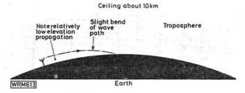
Fig. 2: Radio horizon distance with the bend of the wave path exaggerated for clarity
