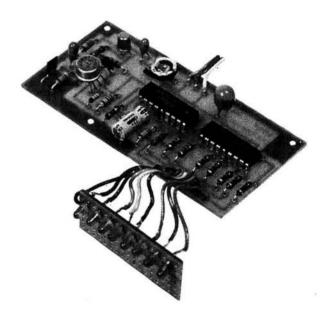
The display drivers can be used in either the "bar" or "dot" mode. In the former case, a true bargraph display is obtained with the number of l.e.d.s illuminated being proportional to the input voltage. In the "dot" mode only one l.e.d. at a time is switched on, this being the highest in the sequence that the input voltage merits.
