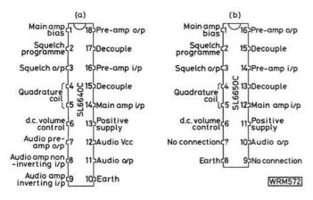
Fig. 2: Pin connections for the SL6640C and for the SL6650C
