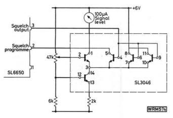
Fig. 4: This circuit may be used with the SL6650C for driving a signal strength meter
