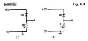
Figs. 4.3(a) and (b) show the two modes of operation of a diode while Figs. 4.4(a) and (b) show the circuit and physical appearance of the diode respectively. In Fig. 4.4(b), the "+" sign which often appears on printed circuit boards shows the cathode end of the diode.
