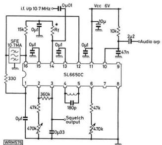
Fig. 6: A 10-7MHz circuit using the SL6650C device
