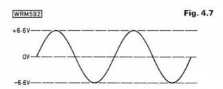
Although the meter does not show it, however, the voltage across the diode is varying at the frequency of the a.c. and varies sinusoidally between -0.6V on positive peaks of the voltage at "A" and +12.6V on negative peaks. The average of these two extreme potentials is 6V, which the meter indicates. Note that the diode must withstand a "peak inverse voltage" of 12.6V, almost double the peak of the a.c. applied to its anode.
