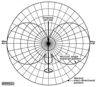
Fig. 3: Vertical angle radiation pattern taken from the prototype Ring-Base antenna as shown in the photo
