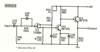
Fig. 1: 50MHz pre-amplifier circuit
