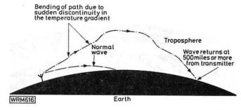
Fig. 5: This sort of tropospheric propagation resulting from modification of the refractive index by sudden discontinuities of the temperature gradient is sometimes called "tropospheric ducting"
