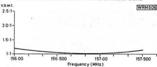
Fig. 5: VSWR—bandwidth readout from a Ring-Base antenna tuned for the 156MHz marine communications band
