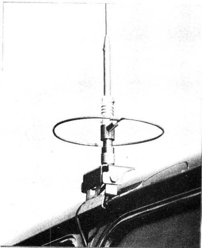
**Gutter-mounted mobile version of the ring-base antenna, fitted with PL259 plug. The inductor has not yet been sleeved**
