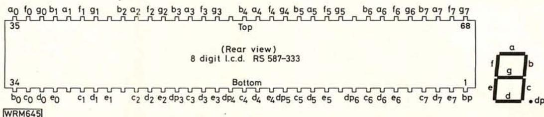
**Fig. 11: Connection details of the l.c.d. display together with segment notation. Non-notated pins are left unconnected**
