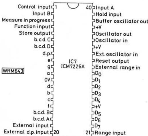
Fig. 12: Pin-out details of the ICM 7226A device
