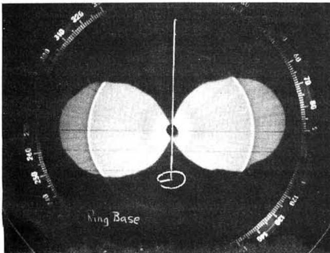
Free-space radiation plot obtained from a 941.9MHz scale model of the ring-base antenna
