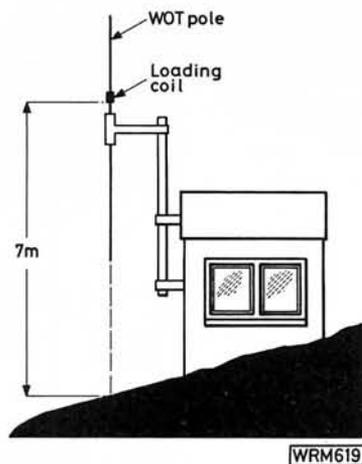
**Fig. 8: The antenna height definition of the HO. A height in excess of 7m requires the r.f. power from the transmitter to be reduced to 0.4 watt**
