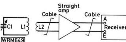
Fig. 2: Ordinary loop with amplifier
