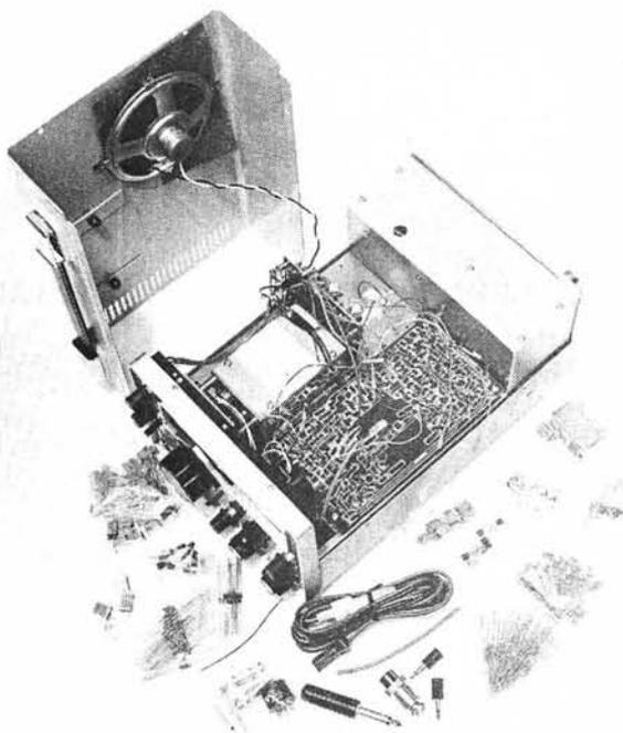
So far as I know the Shimizu SS-105S is unique, certainly in the UK, being a part-built, part-kit h.f. transceiver. For someone with a reasonable amount of constructional experience, it provides a useful insight into the system design of a multi-mode rig which, though it lacks many of the frills and gadgets which seem to cram every new "black-box" these days, nevertheless provides all the basic requirements for c.w. or s.s.b. operating, and n.b.f.m. too, if you so desire.
