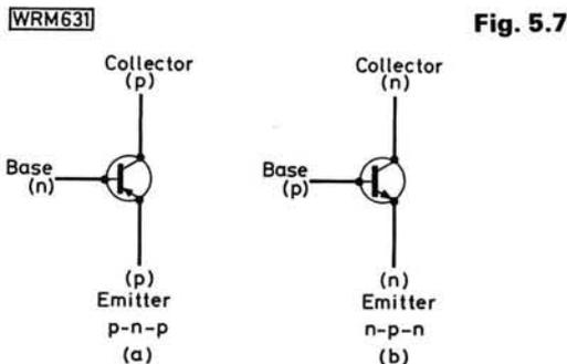
So the base-emitter potentials we can expect to measure are exactly the same as for the junction diode and, if suspect, the base-emitter junction can be tested by ohmmeter in exactly the same way as the diode.
