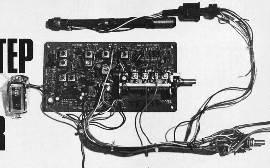
This module contains a complete m.w., l.w. and v.h.f. stereo tuner suitable for use with a d.c. power supply and a stereo audio amplifier.
