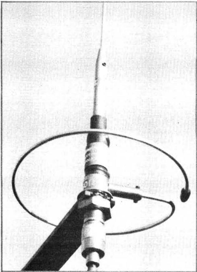
The assembled base station version, showing the mounting bracket and base assembly
