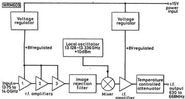
Fig. 2: Schematic diagram of the K-band down converter
