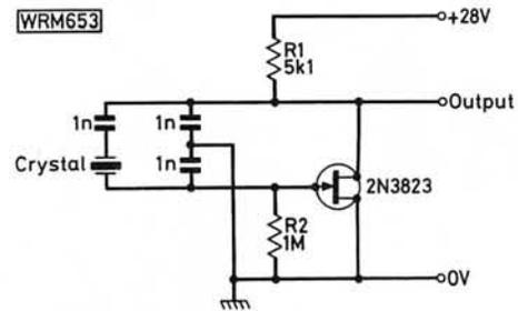
Fig. 2: A Colpitts crystal oscillator circuit
