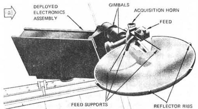
**Shuttle Integrated Radar and Communications sub-system for K-band use**
