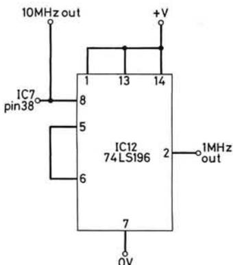
**Fig. 6: Circuit details of the optional divider stage to provide a 1MHz calibration signal. The p.c.b. track will require modification**
