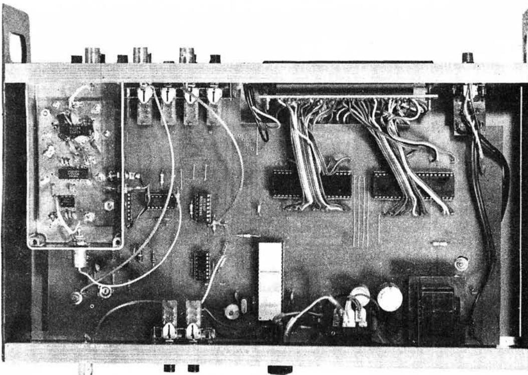
Photograph of the author's prototype 600MHz frequency meter. The approximate cost to construct this version would be £100
