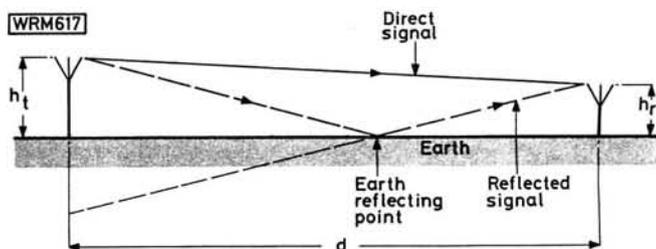
Fig. 6: A receiving antenna responds to two signals over a direct and reflected path, the net signal then falling as a function of the inverse square of the distance
