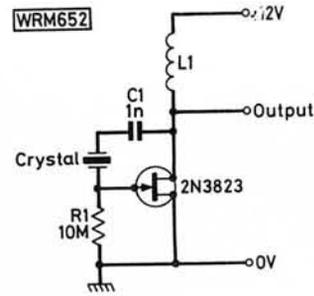
Fig. 1: A simple Pierce oscillator circuit
