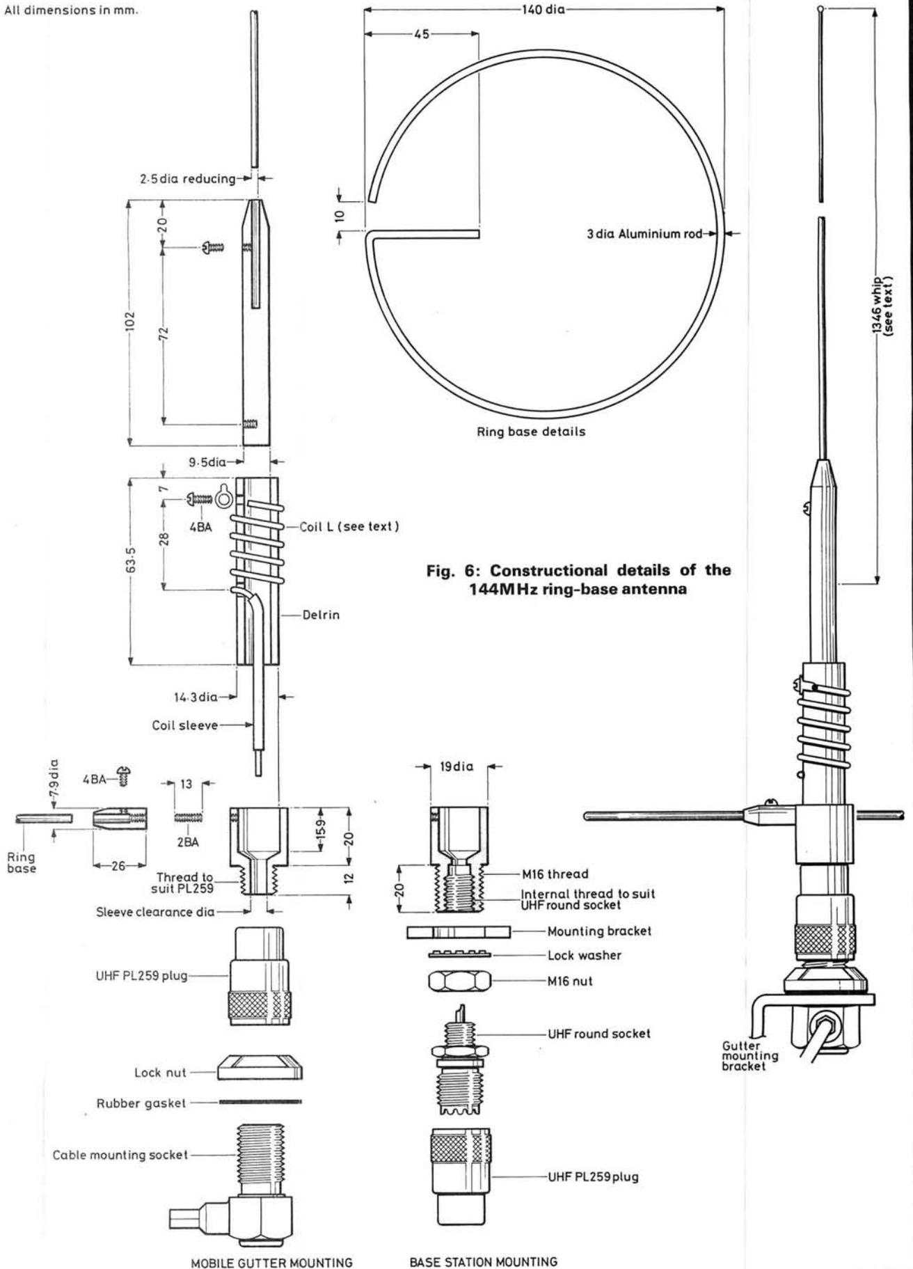
Fig. 6: Constructional details of the 144MHz ring-base antenna
