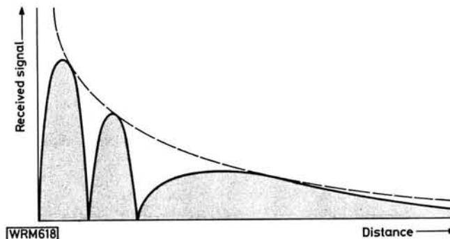
Fig. 7: Showing how the received signal varies with distance from the transmitting antenna
