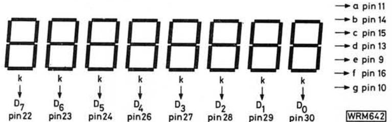
Fig. 13: Connection details of the alternative I.e.d. display. All segment anodes are paralleled, cathodes connect to appropriate pins on IC7
