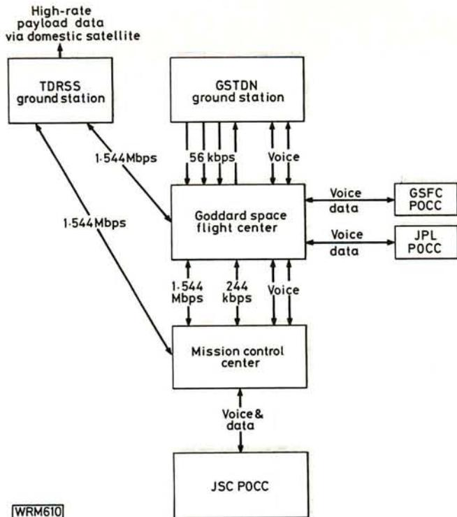
Fig. 4: Flow diagram of ground communications
