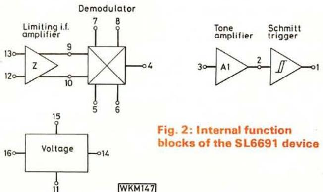
Fig. 2: Internal function blocks of the SL6691 device
