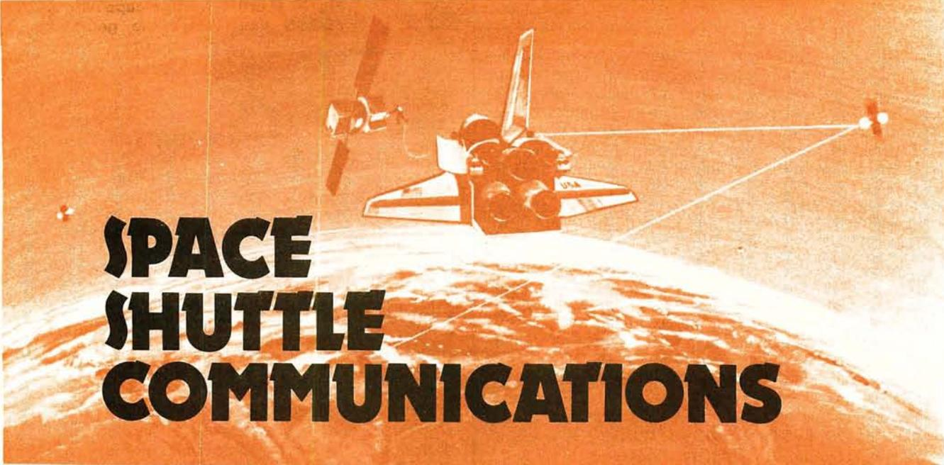
A diagram showing a space shuttle in orbit above Earth's surface. Two Tracking and Data Relay Satellites (TDRSS) are also in orbit. Lines represent communication links between the shuttle and the satellites, and between the satellites and each other. The Earth's horizon is visible at the bottom.
