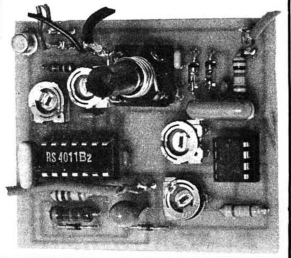
When the voltage on pin 2 rises via the C5/R5 network to the transfer potential, the gate is enabled and the circuit begins to produce its pulse output. This is then amplified by the transistor stage Tr1 which drives the speaker.
