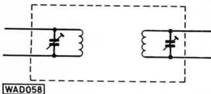
Fig. 1: Original i.f. transformer
