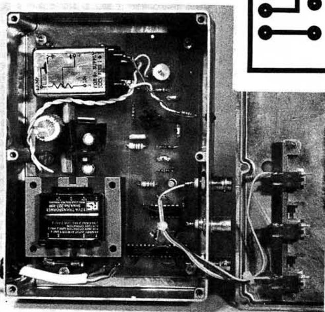
connections made with ribbon cable. The three sockets and i.e.d. were mounted in the side of the box, and on the opposite side a hole was drilled for the mains lead strain relief bush. Diode D3 is soldered directly to the i.e.d. D2 and is fitted as the i.e.d. is switched across an a.c. supply.
