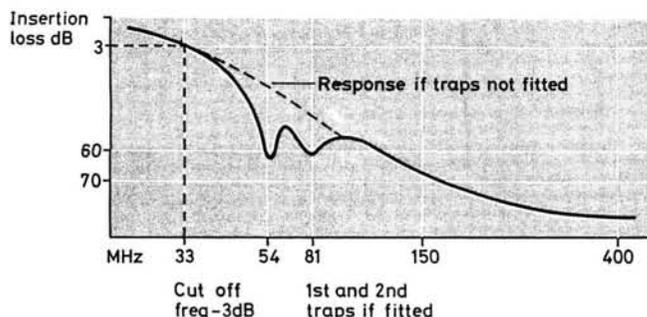
**Fig. 3(a): Typical frequency response of low-pass filter (not to scale). The series tuned traps (if fitted) will normally be tuned to the second and/or third harmonics of the 27 to 30MHz band. The basic circuit is as shown**
