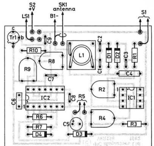
Fig. 2: Track pattern and component layout for the p.c.b. shown full size
