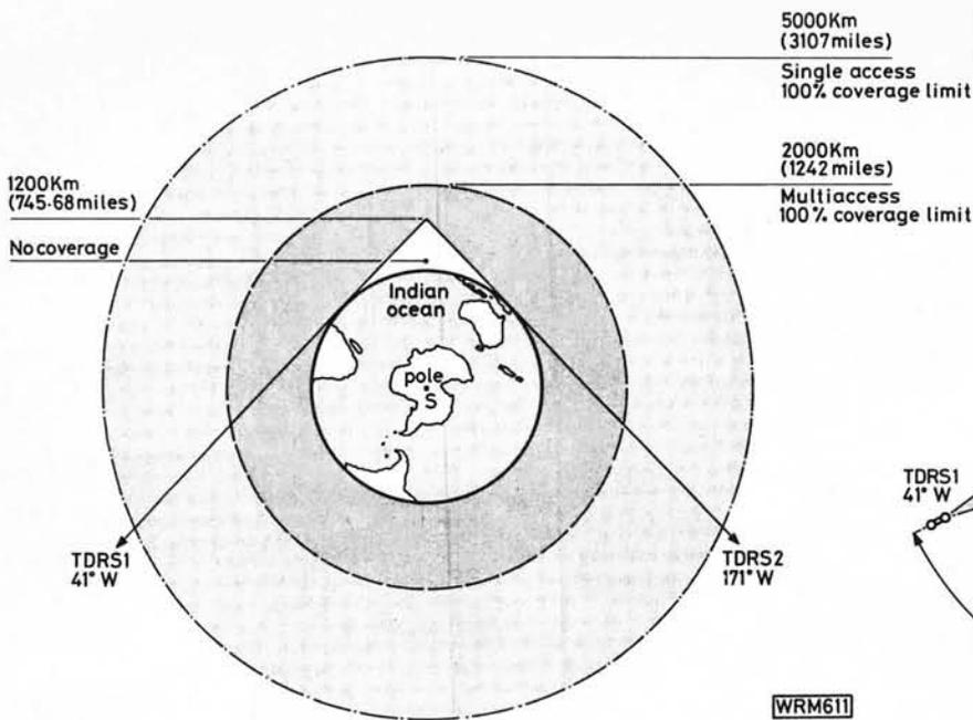
**Fig. 3: (Left) Coverage capability of the TDRSS and below the geometry of placement**
