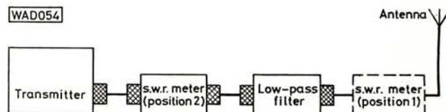
Fig. 1: General layout of equipment for transmitting
