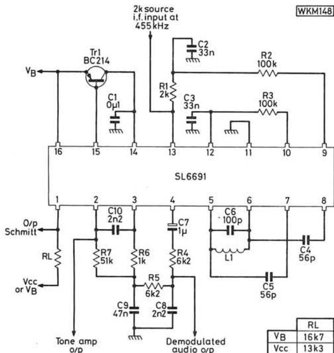
Fig. 3: A SL6691 circuit for demodulating an f.m. signal and providing a paging output if required
