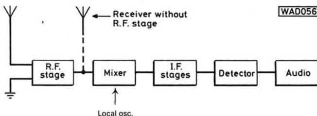
Fig. 1: Block diagram of a superhet receiver
