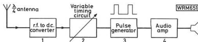
Fig. 1: Block diagram of the time-out alarm
