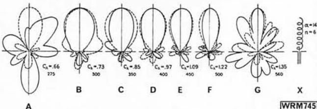
**Fig. 2.3:** Radiation patterns of a nominal 400-450MHz six turn helical antenna across the range 275-560MHz
