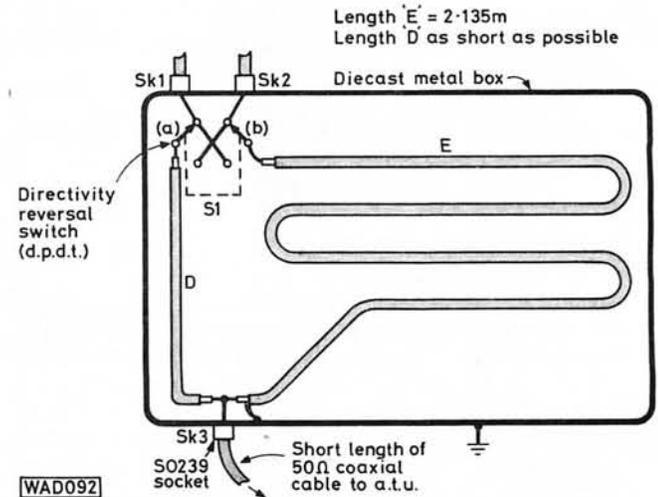
Fig. 3: Internal details of the phase reversing unit
