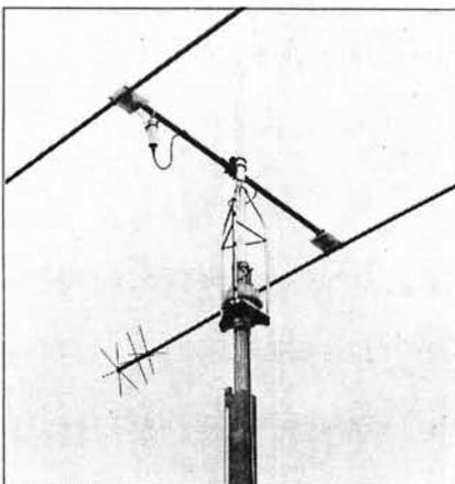
**The RH1 rotator head, with KR-400 and G4MH Minibeam. The mast is only partly extended**
