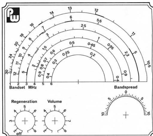
Fig. 4: The front panel dial of the LMS receiver, shown here half full size. Solid lines around the scale are broadcast bands with amateur allocations shown dotted
