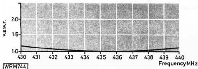
**Fig. 2.2:** The v.s.w.r. readout obtained from the prototype 432MHz Slim Jim
