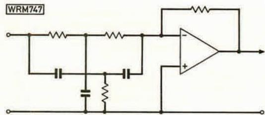
Fig. 1: The basic bridge circuit
