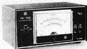
The PM 2000A is an accurate means of measuring your peak envelope out put of power on SSB. The unit has been inspected by the Home Office and found suitable for its purpose. SWR measurements can also be made but the PM 2000A does what all other SWR meters cannot do, i.e., tell your peak cutout power as required in your licence.
