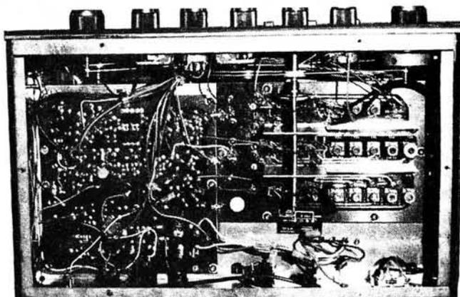
pin 6, the black one from BLK goes to pin 3 and the remaining yellow wire coming from B-YELL is soldered to pin 4. The new r.f. transformer is soldered to a small bracket which is attached to the rear of the main tuning capacitor using the small screw that holds on a wiring clip. The four short ends of the wires left on the medium wave winding on the ferrite rod are tied onto the rod so that they are available in the future.
