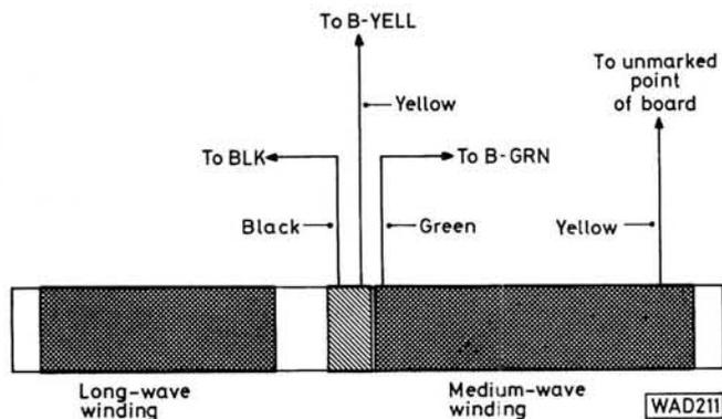
Fig. 2: Ferrite rod antenna, viewed from rear
