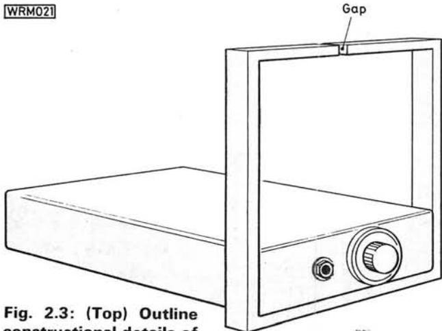
Fig. 2.3: (Top) Outline constructional details of the ferrite rod antenna. (Above) Frame antenna details
