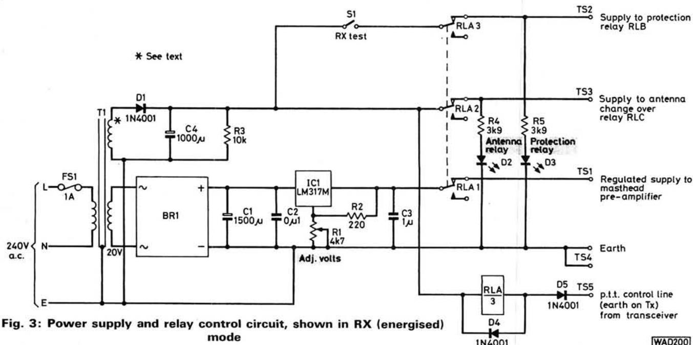
Fig. 3: Power supply and relay control circuit, shown in RX (energised) mode
