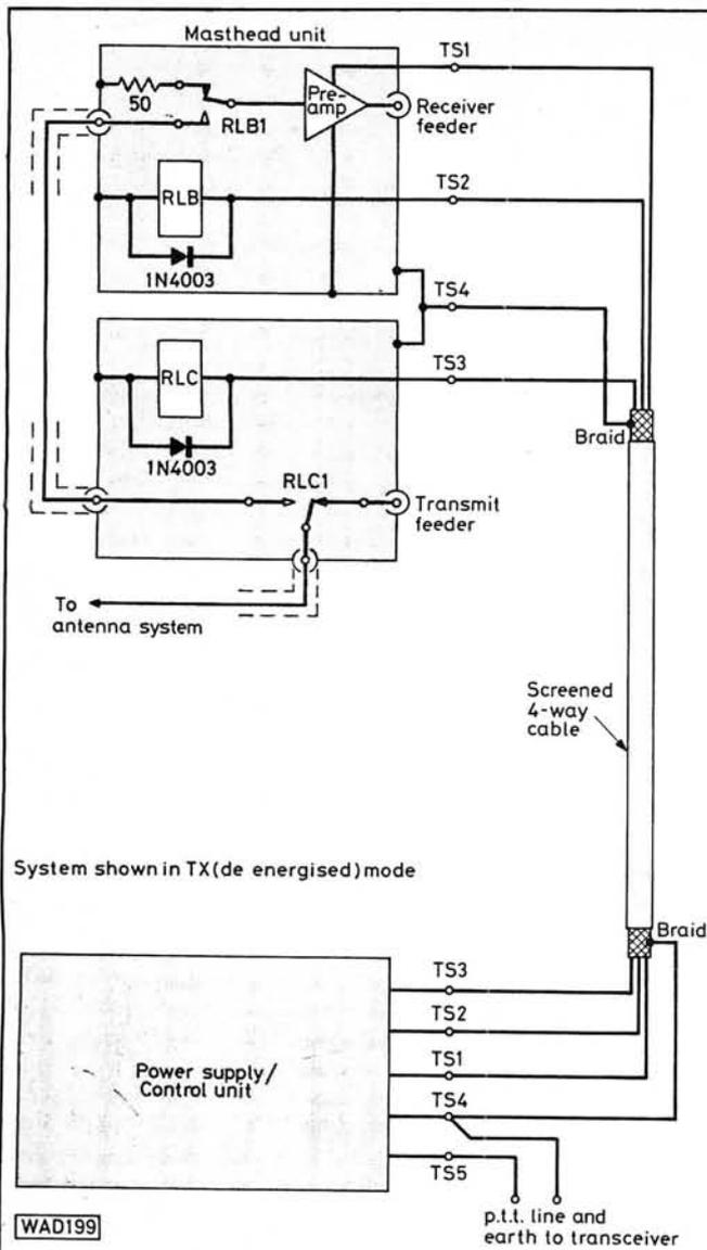
**Fig. 4: System interconnections and relay control arrangements of the masthead pre-amplifier**
