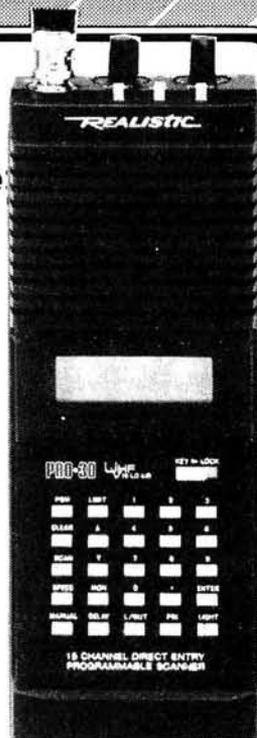
**Realistic PRO-30.** Scan up to 16 of your favourite channels continuously, or search a selected frequency range for new or unpublicised channels. Scan and Search in two speeds. Two-second Scan Delay, selectable for each channel prevents missed replies. Has jacks for external antenna and earphones. Requires six "AA" batteries or mains or DC adapter. Memory backup requires four silver-oxide batteries. **20-9131**
