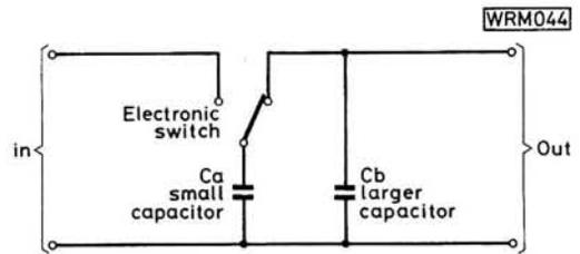
**Fig. 1: The basic arrangement of a switched capacitor filter**
