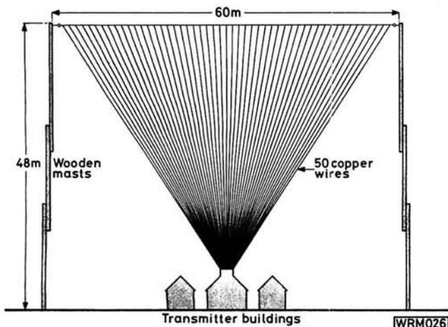
**Fig. 2.1: The temporary antenna system set up by Marconi and G.S. Kemp at Poldhu and which was used for transmitting the first wireless signals across the Atlantic Ocean to St. John's, Newfoundland**
