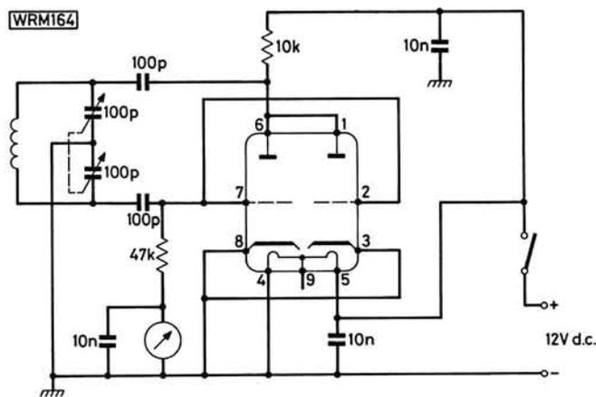
Fig. 1: Circuit of grid dip oscillator using a 12V d.c. supply for both valve heater and h.t. Other valve types which may be used, with similar pin connections, are the ECC81 and ECC83. Four or five plug-in coils may be used to cover 1.8 to 30MHz although the circuit will work into the v.h.f. range. Fixed capacitors should be silver mica or similar. The meter can be a 50 or 100µA f.s.d. type
