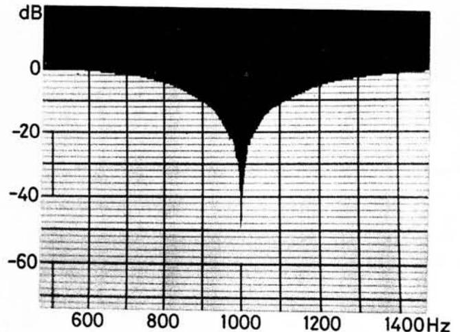
Measured frequency response of the prototype tuned to 1kHz on "Manual"
