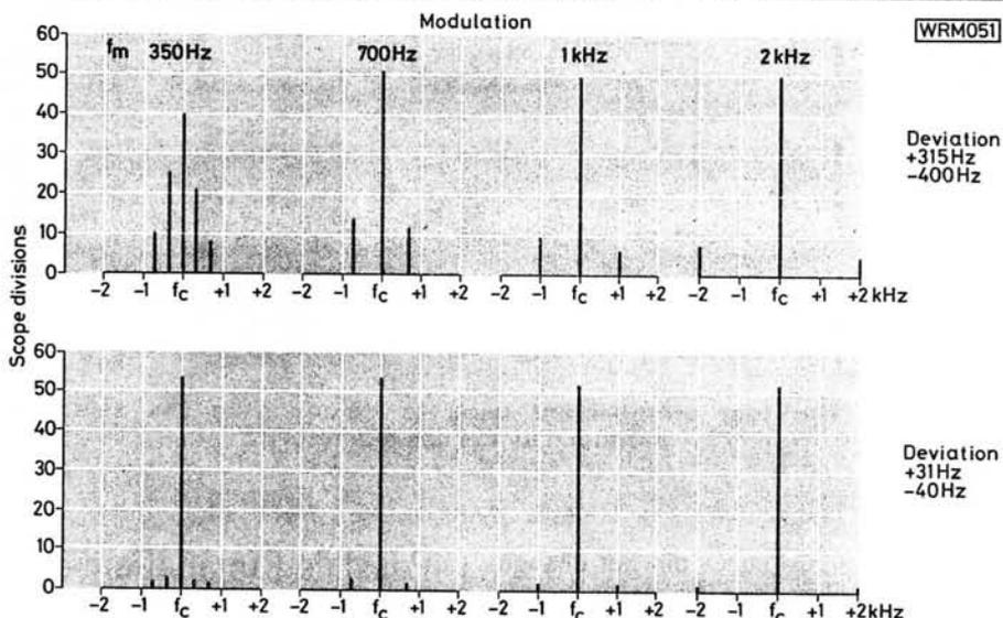
Fig. 5: Sideband amplitudes are shown to reduce with a reduction in deviation or an increase of modulation frequency
