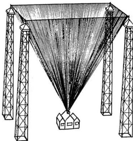
**Fig. 2.2: The original Glace Bay (Nova Scotia) antenna for transatlantic service erected 1902**
