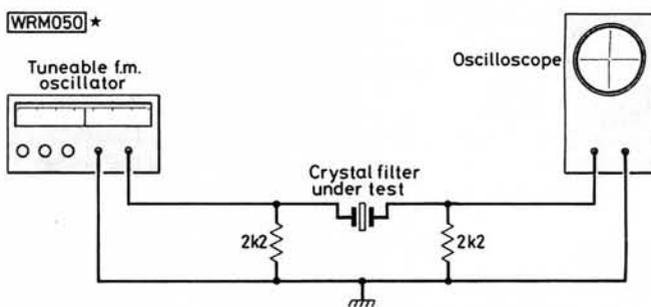
Fig. 4: Test arrangement used to demonstrate sideband amplitude variations
