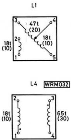
Fig. 2: Coil winding details
