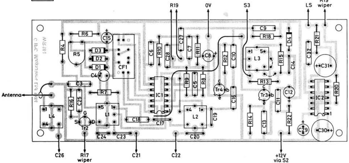
Fig. 3: Full-size p.c.b. track pattern and component layout for the receiver
