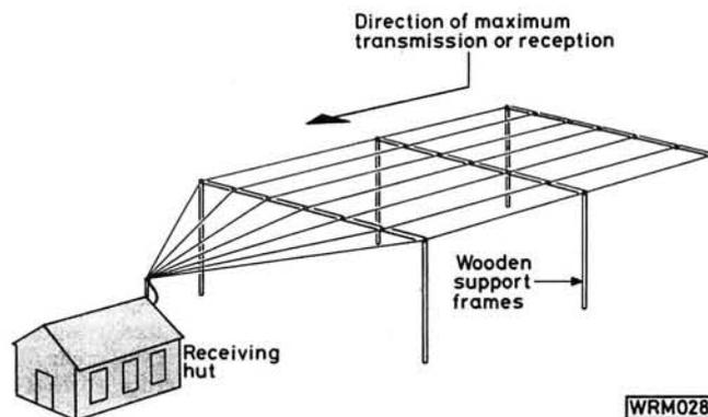
**Fig. 2.4: Marconi's patent "bent antenna" for directional transmission and reception**
