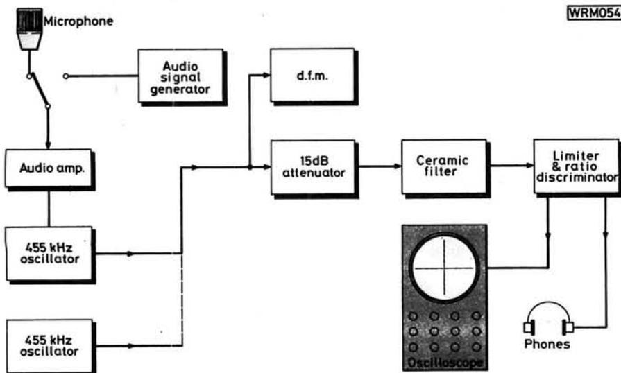
Fig. 8: The test arrangement used to demonstrate the selectivity produced by the use of a filter
