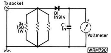
**Fig. 1: Suitable circuit for low power measurement in a 50Ω system. The resistors should not be wirewound. All leads (except those to voltmeter) should be as short as possible (10mm maximum). The meter will read  $(\sqrt{100P-0.6})$  volts for a power of P watts (16.7V at 3 watts)**
