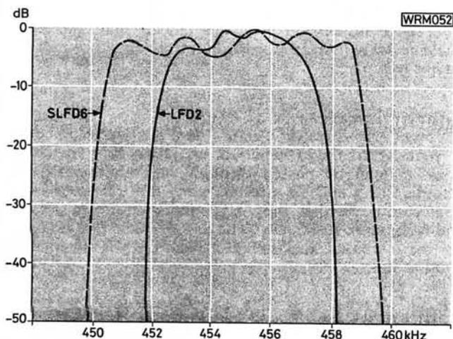
Fig. 6: Comparison of passband characteristic response curves
