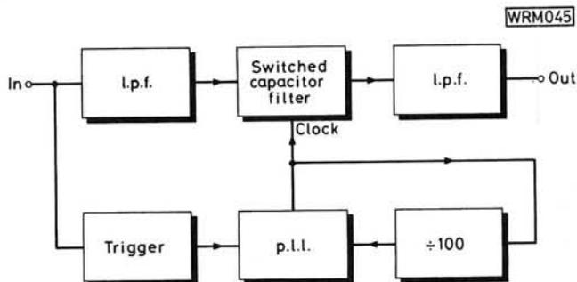
Fig. 2: The Auto-Notch Filter block diagram
