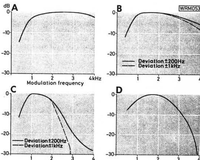
Fig. 7: Audio response curves, A: without filter, carrier 455kHz, deviation  $\pm 200$ Hz and  $\pm 1$ kHz—no change except in amplitude. B: SLFD6 filter under the same conditions. C: LFD2 response. D: The LFD2 again but with deviation adjusted to keep modulation index at 0.3
