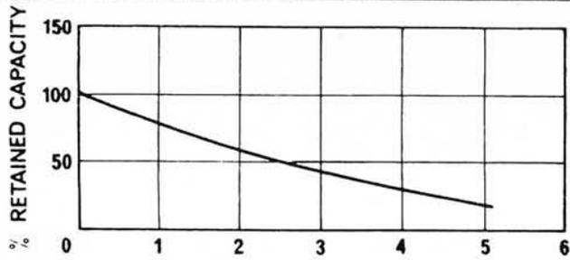
Charge retention with time for nickel-cadmium cells
