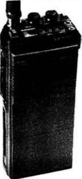
The ultra compactness of the FT203R is due mainly to Yaesu's chip component circuit board assembly, the chip components being installed automatically by robots. The 203's features include thumbwheel frequency selection, built in S/PO meter, 2.5W RF O/P at 10.8V, (3.5W O/P with FNB4). Vox activated switching is possible when used in conjunction with YH-2. Accessories supplied include FNB3, FTE-2 tone unit, CSC6 case and YHA-14A antenna.
