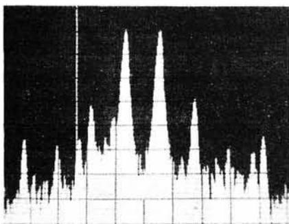
Spectrum analyser plot of 3rd order i.m.d. at 14.1MHz. Tones 800 and 1400Hz. Scale 10dB/div. vertical, 500Hz/div. horizontal. The suppressed carrier is just to the right of the bright line
