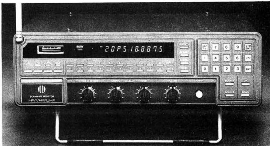
receiver's coverage to be extended down to 150kHz and up to 3.7GHz; also available is a dedicated regulated power supply unit and data interface unit.
