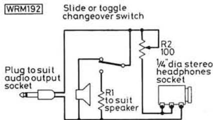
Fig. 1: Simple circuit for a unit providing rapid changeover from speaker to headphones when VR1 is adjusted for comfortable listening level
