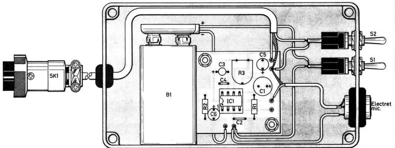
Fig. 2: Component layout and p.c.b. track pattern shown full size. The version shown uses an electret insert mounted in the enclosure wall within a rubber grommet. An appropriate socket/captive plug would be fitted in place of the insert if used with the original transceiver hand-held microphone
