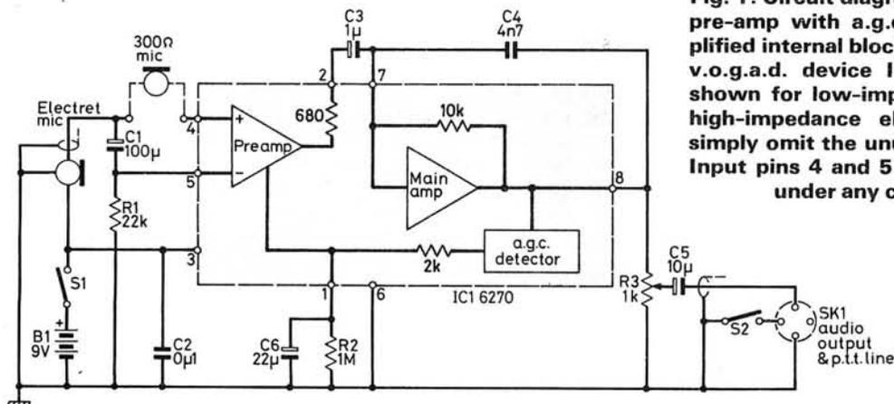
Fig. 1: Circuit diagram of the microphone pre-amp with a.g.c. including the simplified internal block diagram of the 6270 v.o.g.a.d. device IC1. Connections are shown for low-impedance dynamic and high-impedance electret microphones, simply omit the unused alternative type. Input pins 4 and 5 must not be earthed under any circumstances
