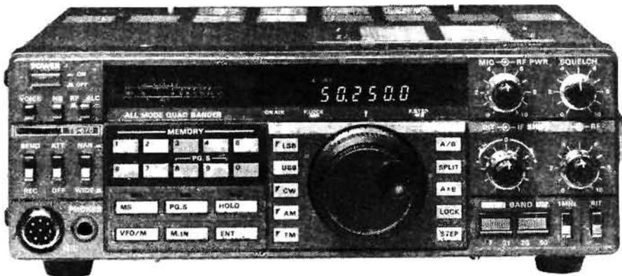
modes available, twin v.f.o.s and 80 memory channels, which can be programmed for mode, memory scan, etc. Whilst primarily intended for base stations use the TS-670 is compact enough for mobile installation.
