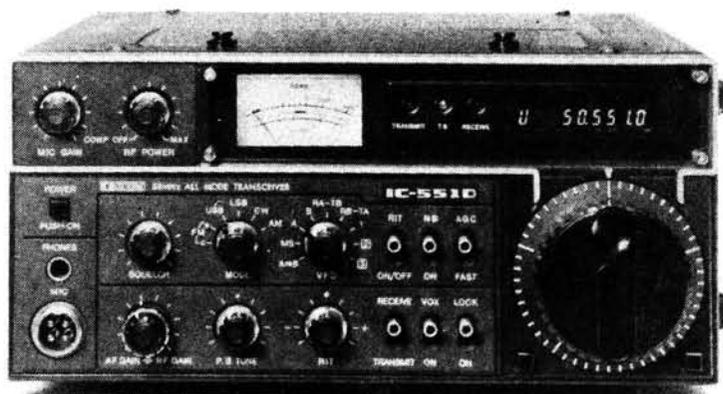
This base station has all mode capability, SSB, CW, AM and FM (when optional FM is installed). It covers 50-54MHz with 80 watts variable R.F. output power (40 watts A.M.), Dual VFO's for split frequency operation. 3 memory channels and memory scan, program scan with adjustable scanning speed and auto stop when a signal is received. A powerful audio output, 2 watts at 8ohms for easy listening even in noisy surroundings.
