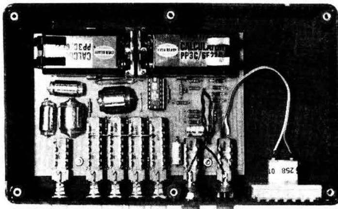
This photograph shows the p.c.b. fitted into a metalised plastics box. Any suitable size of box or case can be used, ideally though it should be metallic or metalised
