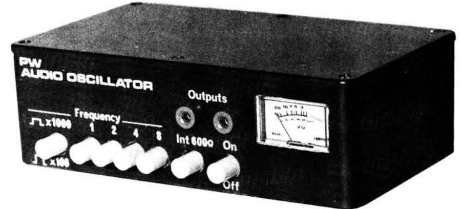
is selected in the range 1–15 by operating four switches in binary sequence. A multiplier switch then sets the final frequency to be 100Hz to 1500Hz in 100Hz steps or 1kHz to 15kHz in 1kHz steps. This approach has the great advantage from a project point of view, in that provided good quality components are used for the Wien
