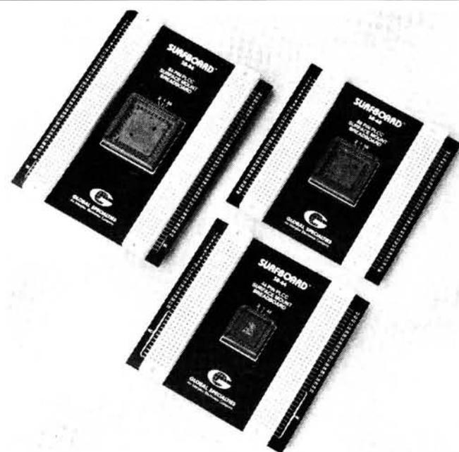
JEDEC "type A" p.l.c.c. polarised for easy registration. Stand-offs are provided for heat dissipation.
