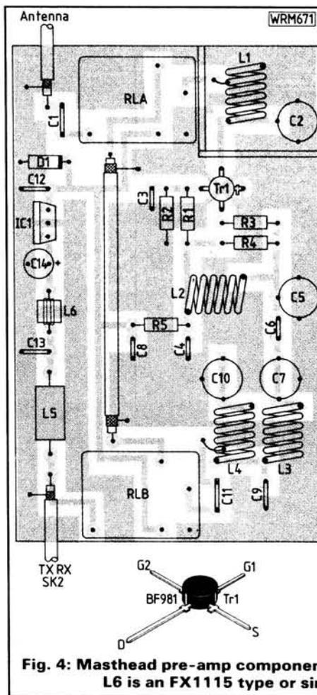
Fig. 4: Masthead pre-amp component layout. Note the ferrite bead used for L6 is an FX1115 type or similar with a 2mm centre hole
