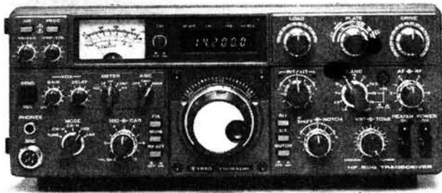
The TRIO TS830S is for the operator who wants a dedicated amateur bands only transceiver, who is used to and wants a pair of 6146B valves in the PA stage and who wants a compact rig which has its own built in power supply. The TS830S is for the radio amateur who requires a rig capable of rising above today's crowded band conditions, a rig that has, as standard, the necessary features that will produce
