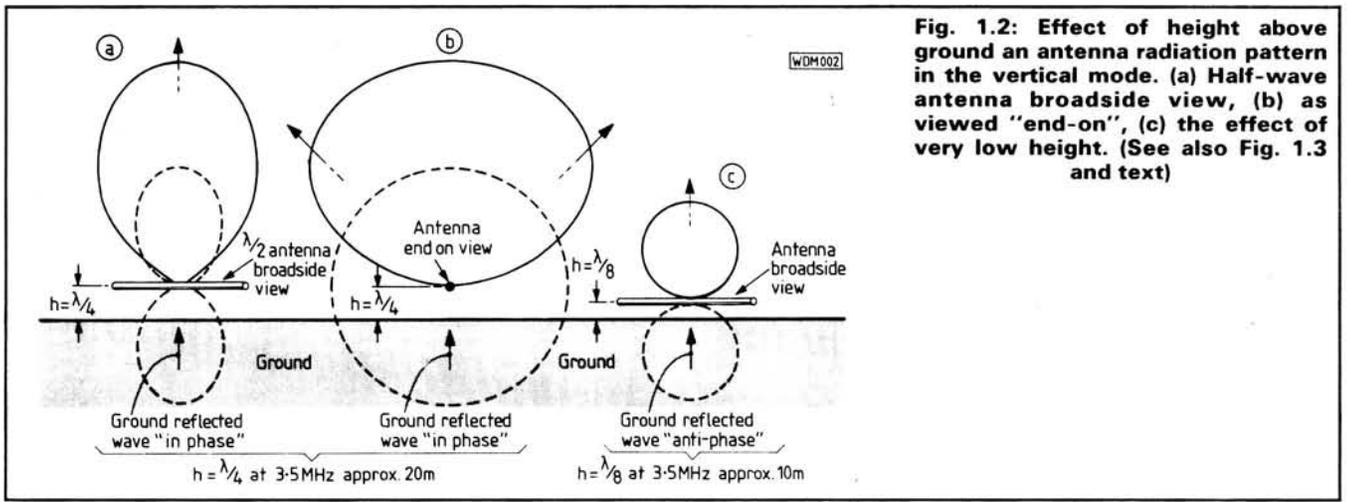
**Fig. 1.2: Effect of height above ground an antenna radiation pattern in the vertical mode. (a) Half-wave antenna broadside view, (b) as viewed "end-on", (c) the effect of very low height. (See also Fig. 1.3 and text)**
