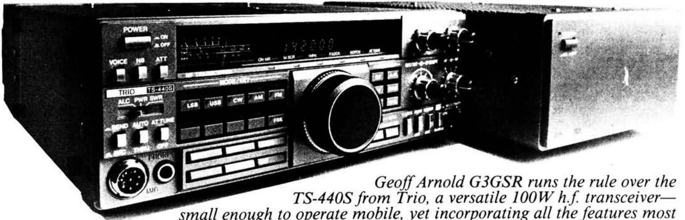
*Geoff Arnold G3GSR runs the rule over the TS-440S from Trio, a versatile 100W h.f. transceiver—small enough to operate mobile, yet incorporating all the features most amateurs would look for.*
