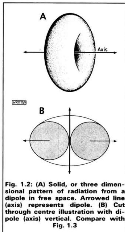
Fig. 1.2: (A) Solid, or three dimensional pattern of radiation from a dipole in free space. Arrowed line (axis) represents dipole. (B) Cut through centre illustration with dipole (axis) vertical. Compare with Fig. 1.3
