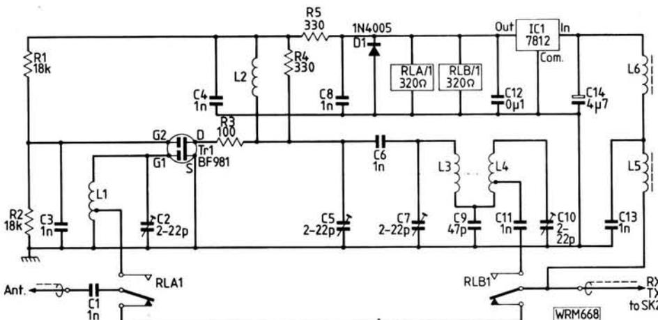
Fig. 1: Circuit diagram of the masthead pre-amp
