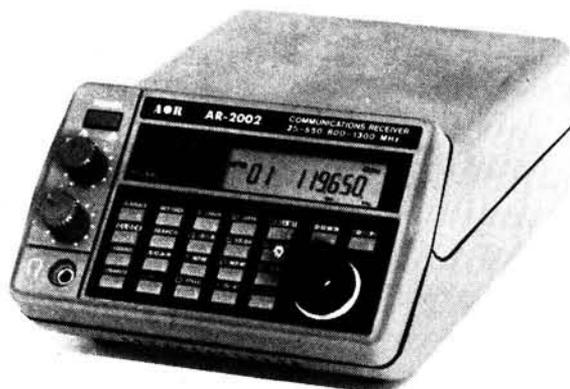
**Frequency range of the AR2002** is from 25 to 550 and from 800 to 1300 MHz. Modes of operation are wide band FM, narrow band FM and AM. The receiver has 20 memories, memory scan and a search mode which checks frequencies between user designated limits.
