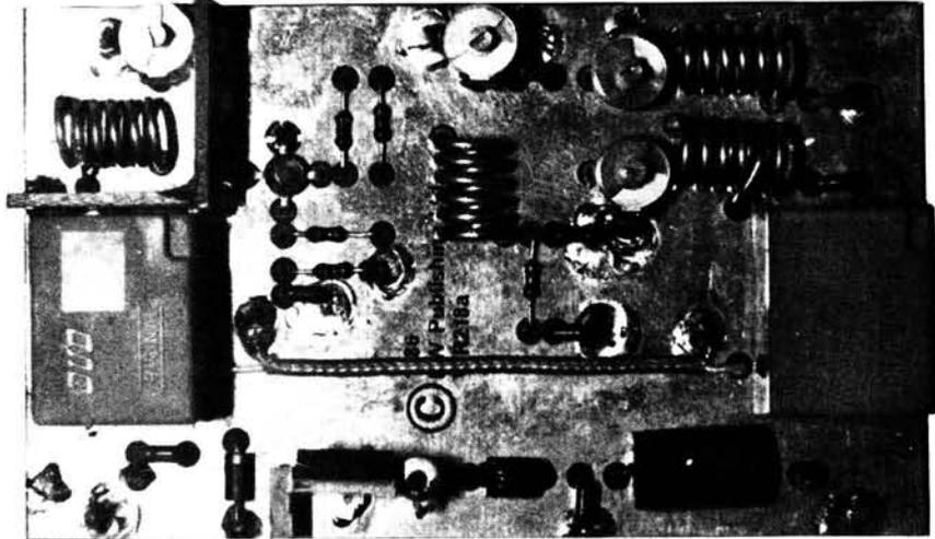
*Pep-up your station with this high performance 144MHz band pre-amp from Peter Rouse GUIDKD. The design possesses high gain, low noise, good dynamic range and an onboard regulator that will compensate for volts drop in the supply on long feeder runs.*
