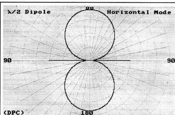
Fig. 1.1: Radiation pattern. Horizontal Dipole. Compare with line diagram of "solid free-space" radiation field as in Fig. 1.2
