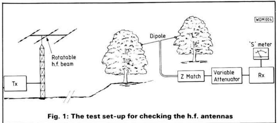
Fig. 1: The test set-up for checking the h.f. antennas
