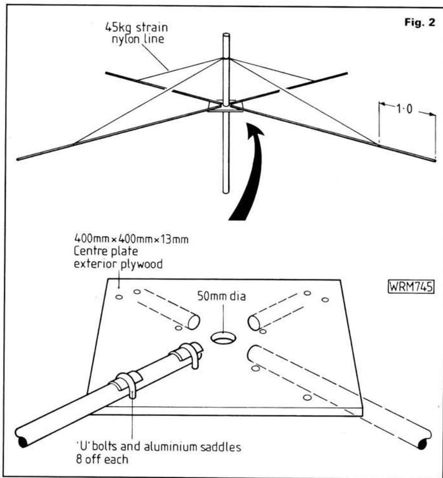
On assembling the framework, ensure that the spiders are straight and spaced at the distance shown in Fig. 1 before drilling any holes. The U-bolts or saddles should be tightened just enough to hold the spiders in position while trimming, yet slack enough to allow movement under gentle pressure for final adjustments.
