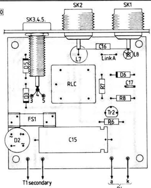
Fig. 5: Power supply component layout
