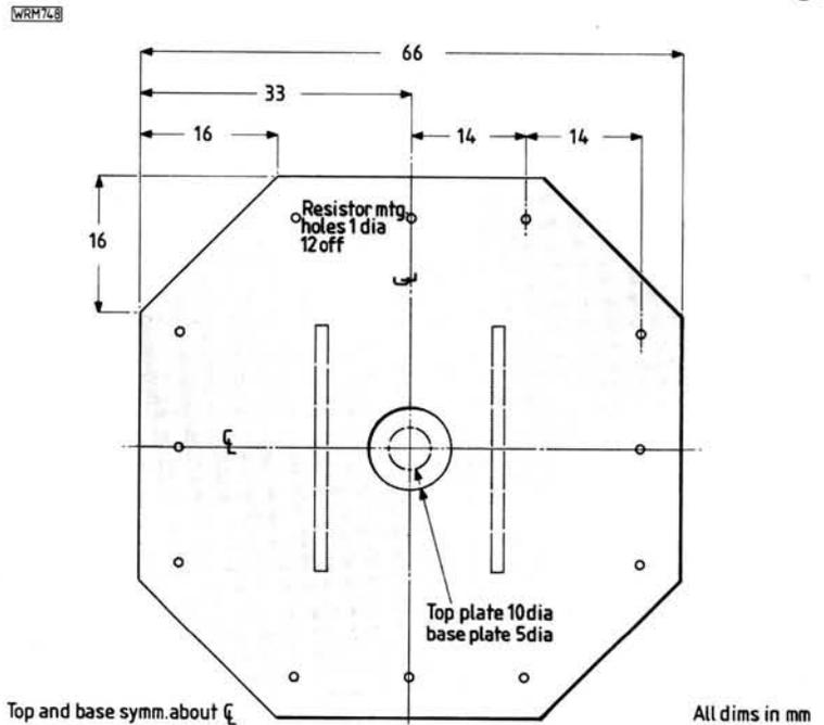
“inside” the bottom plate to be soldered by simply poking the solder between the resistors and touching it on the rod and then the c.c.b.
