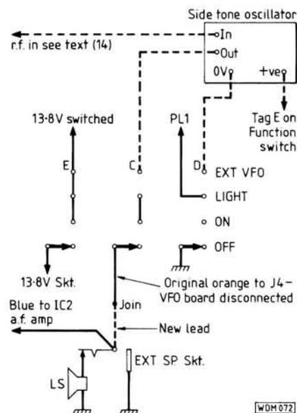
Fig. 5: New wiring between function switch and oscillator
