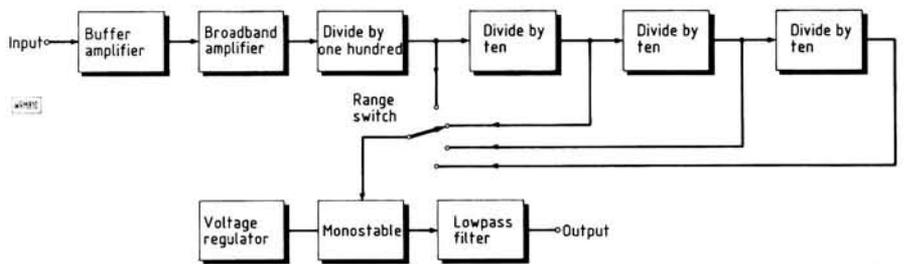
Fig. 2. Block diagram for the d.v.m. to d.f.m. converter
