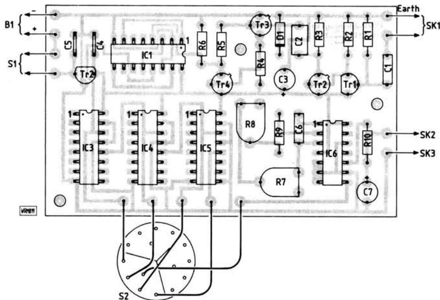
Fig. 5. Single-sided track pattern and component layout of converter (shown full size)
