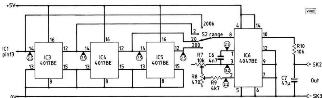
Fig. 4. Circuit diagram of range, monostable, and filter stages. All measurements made with d.v.m. set to d.c. volts, input signal 20mV 1MHz
