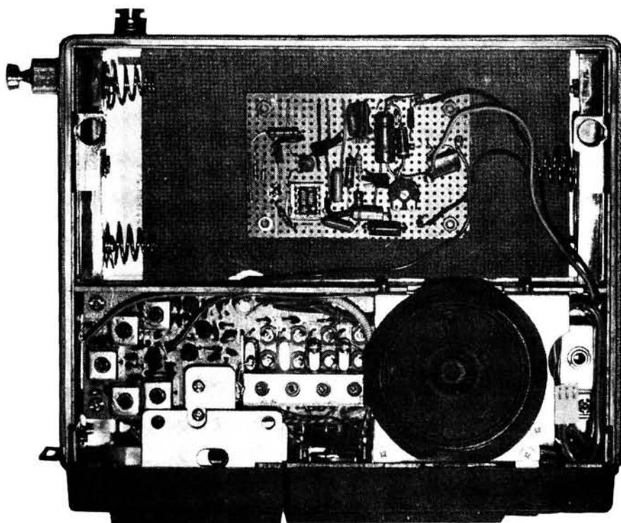
Prototype oscillator installed in IC-202E battery compartment
