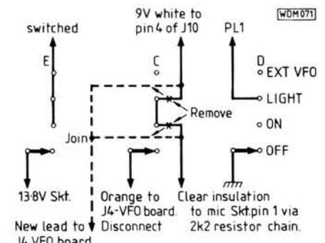
Fig. 4: Original function switch wiring and modification to 9V supply
