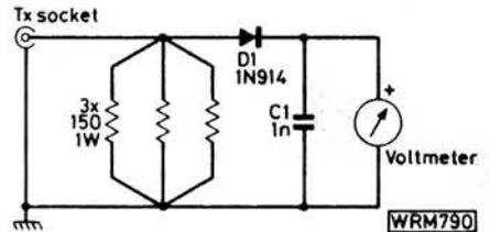
**Fig. 1: Suitable circuit for low power measurement in a 50 system. The resistors should not be wirewound. All leads (except those to voltmeter) should be as short as possible (10mm maximum). The meter will read (100p)—0.6v for a power of P watts (16.7V at 3W)**
