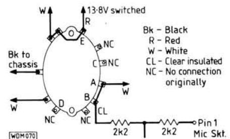
Fig. 3: IC-202E function switch
