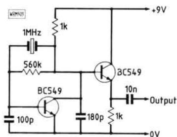
Fig. 6. Circuit diagram for simple calibration oscillator
