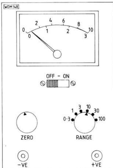
The front of the multimeter, showing the necessary panel markings
