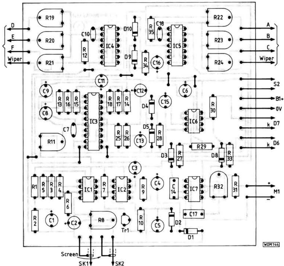
**Fig. 6: Single-sided p.c.b. track pattern and component overlay, shown full size**
