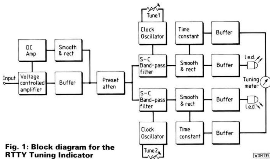
**Fig. 1: Block diagram for the RTTY Tuning Indicator**
