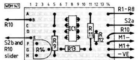
The Veroboard layout of the multimeter
