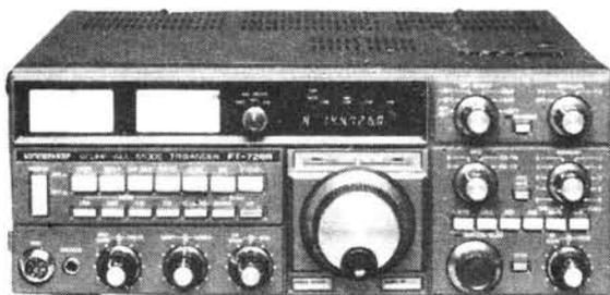
★ Specifications for VHF/UHF options. All modes LSB, USB, CW & FM. 10W RF output & <math><0.25\mu\text{V}</math> for 12dB sinad. Synthesised dual VFO's & 11 memories. Switchable freq. steps and programmable RPT shift. Full duplex operation (with optional module). Packet radio compatibility.
