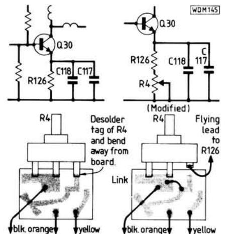
**Fig. 1: (Top) Circuit diagram of pre-driver stage before and after modification. (bottom) View from the track side of the control p.c.b. before and after modification**
