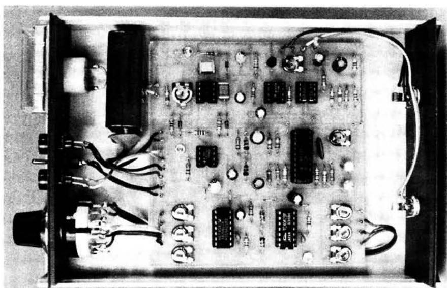
iron being held in place no longer than is really necessary. At this stage pins are fitted to the board at the points where connections to off-board components will eventually be made.
