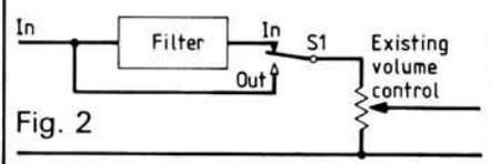
this gives 3dB down points at 733 and 867Hz or approximately 150Hz bandwidth. The input impedance is high which means it can be connected to nearly any audio circuit and the output impedance is fairly low. In fact it is safest to keep the output load above about 250 ohms so as not to cause problems in the 741.
