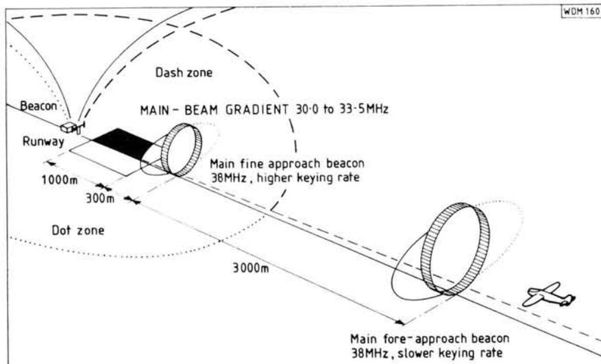
Fig. 1.5: The principle of the Lorenz blind-landing system
