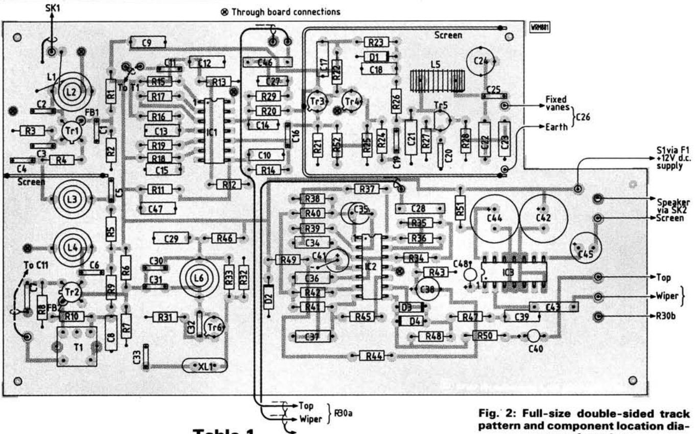
**Fig. 2: Full-size double-sided track pattern and component location diagram of receiver**
