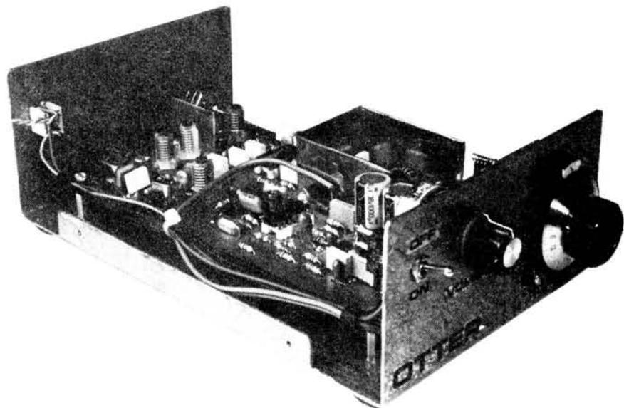
giving the receiver optimum performance around the six metre calling frequency 50.2MHz, where most of the activity takes place.
