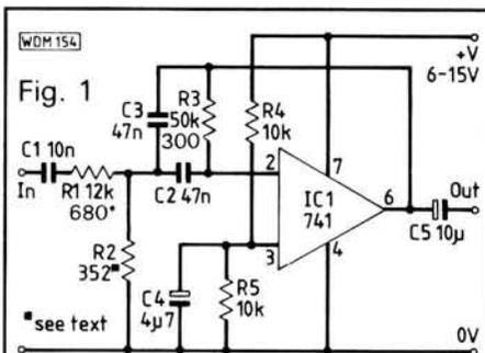
Note that the resistors R1, R2 and R3 are made up of two resistors in each case. See the text for further details
