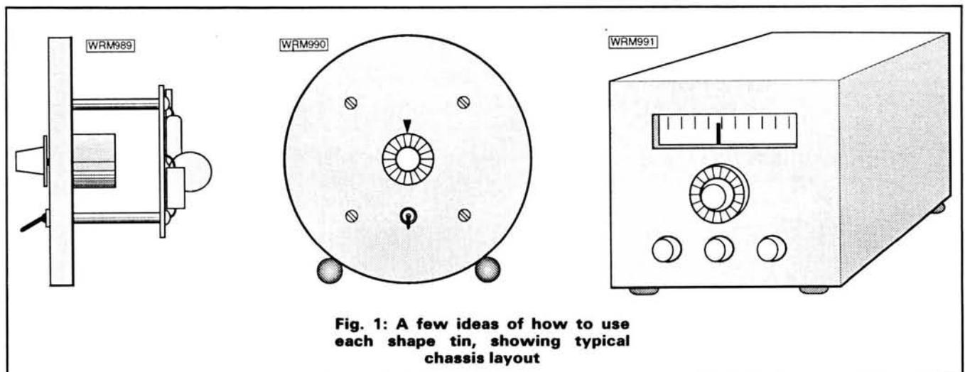
**Fig. 1: A few ideas of how to use each shape tin, showing typical chassis layout**
