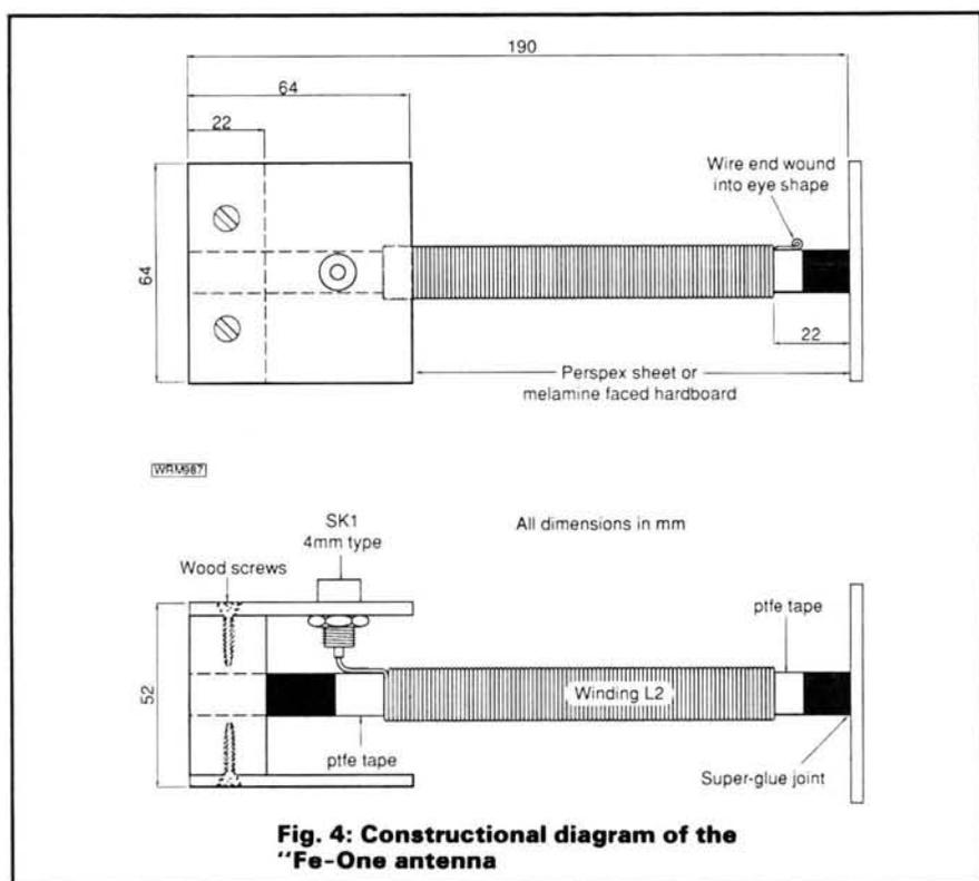
**Fig. 4: Constructional diagram of the "Fe-One" antenna**
