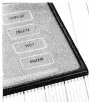
artificial beepers or lights. The metal dome provides the actual electrical contact of the switch so there is no possibility of a "click" occurring without electrical contact being made. Being metal also means that the switch can handle larger currents than conventional flexible membranes and offer greater reliability.
