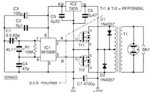
Fig. 2: Basic synchronous d.c. to a.c. converter circuit. The gates of Tr1 and Tr2 are connected to points A and B shown in Fig. 4. Resistors R2 and R3 together with IC3 need not be used.
