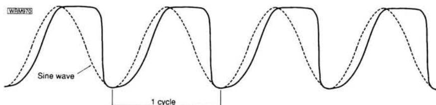
Fig. 10.1: A distorted waveform
