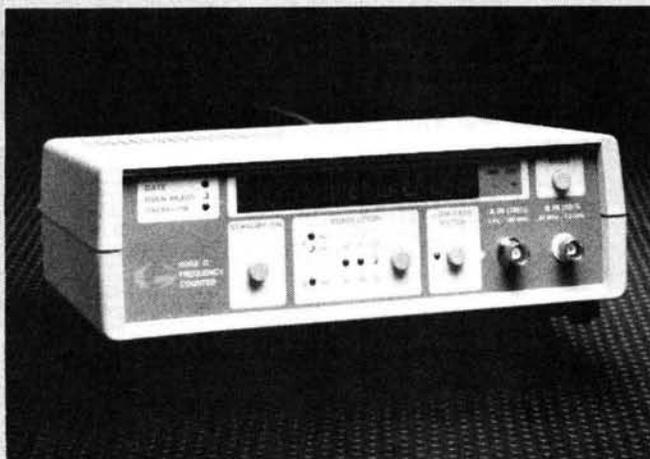
signals from 5Hz to 100MHz with an impedance of 1MΩ/20pF. Input B accepts signals from 80MHz to 1.3GHz with a 50Ω impedance.
