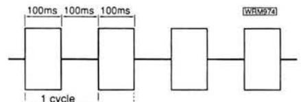
Fig. 10.6: The shaped envelope for Morse dots
