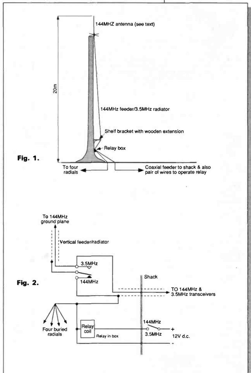
the relay in a die-cast box to protect it. Any plastics box would be just as good. Spread a little sealant around the point where the cables enter the box to keep moisture out.
