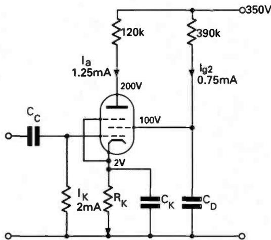
**Fig 4.1: Shows an EF86 pentode valve with anode, cathode and screen resistors and the various voltages that constitute the d.c. conditions.**
