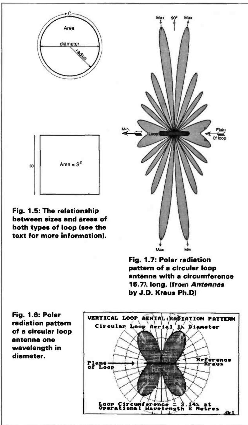
Fig. 1.5: The relationship between sizes and areas of both types of loop (see the text for more information).
