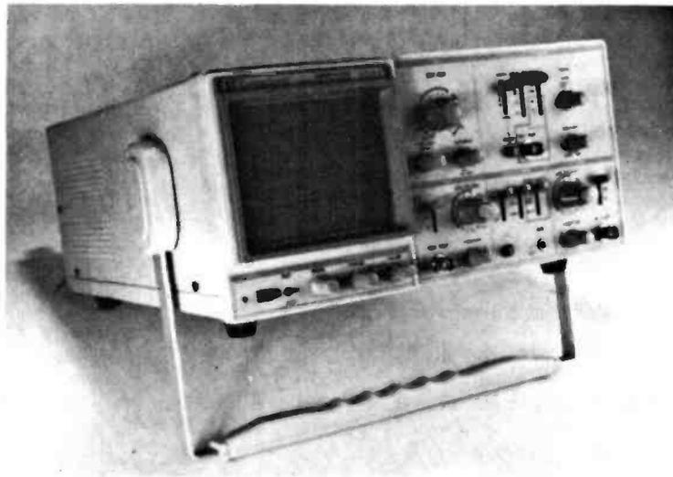
The Topward TOS-7000 series of oscilloscopes distributed by Maplin Electronics has great appeal to the amateur and professional. The 7021 reviewed here represents a very popular model from the range that has particular appeal to the amateur. It features a 20MHz bandwidth, triple trace and a clear 150mm rectangular display.
