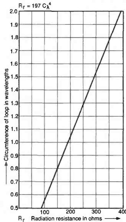
Fig. 1.9: Radiation resistance of small loops.
