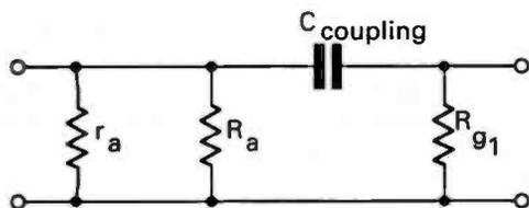
Fig. 4.6: The low frequency equivalent circuit.
