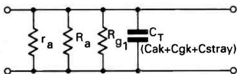
Fig. 4.5: High frequency gain equivalent circuit.
