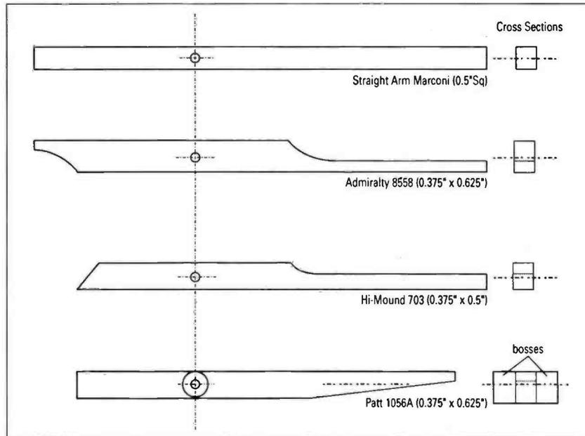
should not exceed 125mm, otherwise noticeable flexing will occur. Selecting a rectangular section of say 0.375 wide x 0.5 inch deep makes a practical alternative to 0.5in square section.
