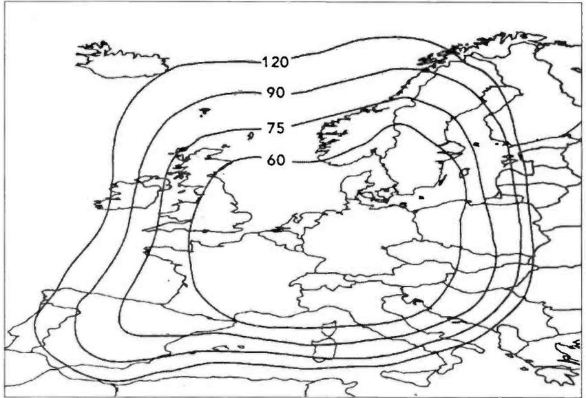
Fig. 1: The Astra satellite coverage footprint.
