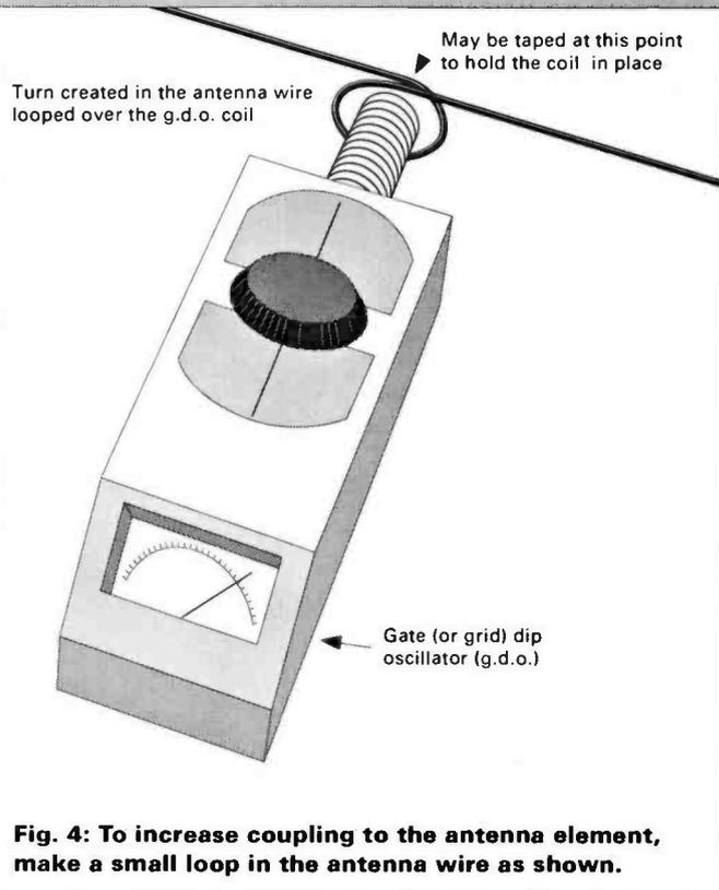
Fig. 4: To increase coupling to the antenna element, make a small loop in the antenna wire as shown.
