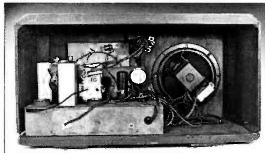
Fig. 2: Rear, internal view of the American receiver.
