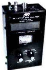
The latest model. It lets you quickly adjust your aerial on site. Instant digital frequency readout of resonance and VSWR. Saves hours of work. Battery powered, you can watch the changes as you adjust your aerial system. Ideal for beams, dipoles, whips and all 50 Ohm coax designs. Get your system tuned in minutes not hours!
