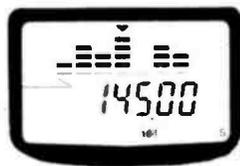
80 memories, 2 Watts on ni-cads, 5 Watts on 12V. But the unique feature is the Spectrum Display. The bargraph shows the strength of the signal you are receiving plus the strength of signals on the 3 channels either side. Watch a spectrum display of the activity as you tune the band. It's the most amazing handheld we have seen!
