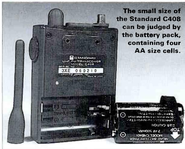
The small size of the Standard C408 can be judged by the battery pack, containing four AA size cells.
