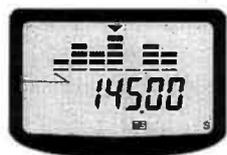
80 memories, 2 Watts on nicads, 5 Watts on 12V. But the unique feature is the Spectrum Display. The bargraph shows the strength of the signal you are receiving plus the strength of signals on the 3 channels either side. Watch a Spectrum Display of the activity as you tune the band. It's the most amazing handheld we have seen!
