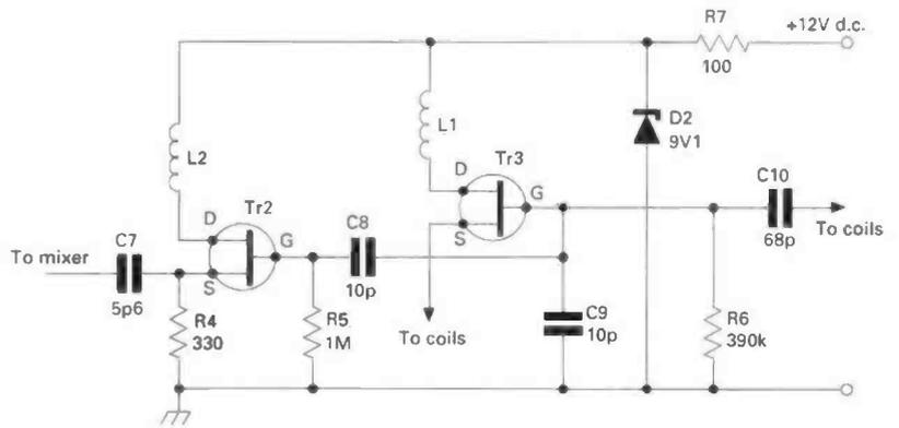
**Fig. 7: New v.f.o. employing f.e.t.s, which can be mounted on the existing p.c.b. (see text).**
