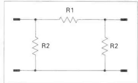
Fig. 2: An unbalanced p network.
