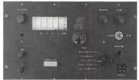
Fig. 4: Tuning scale and front panel controls.
