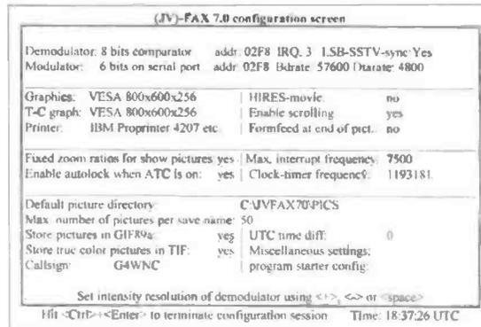
Fig. 1: The JVFA 7.0 configuration screen.
