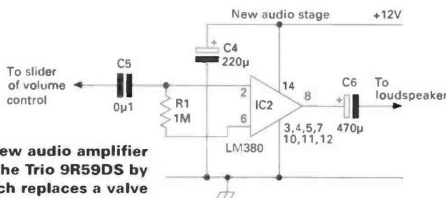
Fig. 3: The new audio amplifier circuit for the Trio 9R59DS by G4BXD, which replaces a valve (see text).
