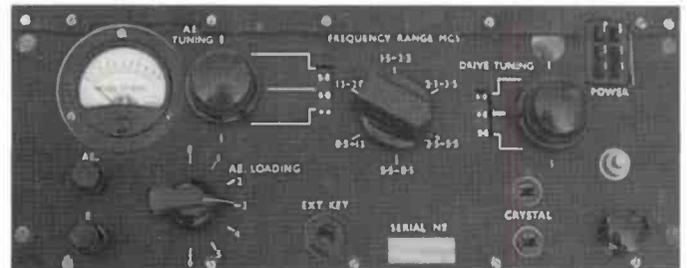
Fig. 5: Transmitter unit of the clandestine transmitter/receiver showing tuning arrangements for the power amplifier (p.a.) stages and provision for crystal control (see text).
