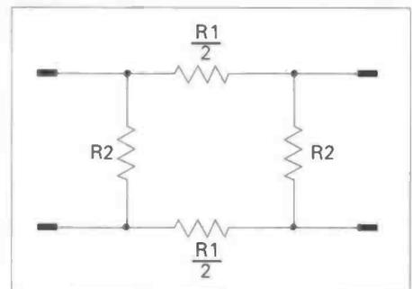
Fig. 4: A balanced p network.
