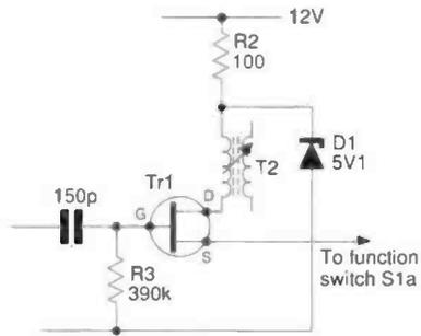
**Fig. 5: The transistorised b.f.o. modification using a f.e.t. The modification is mounted directly onto the existing p.c.b. (see text).**
